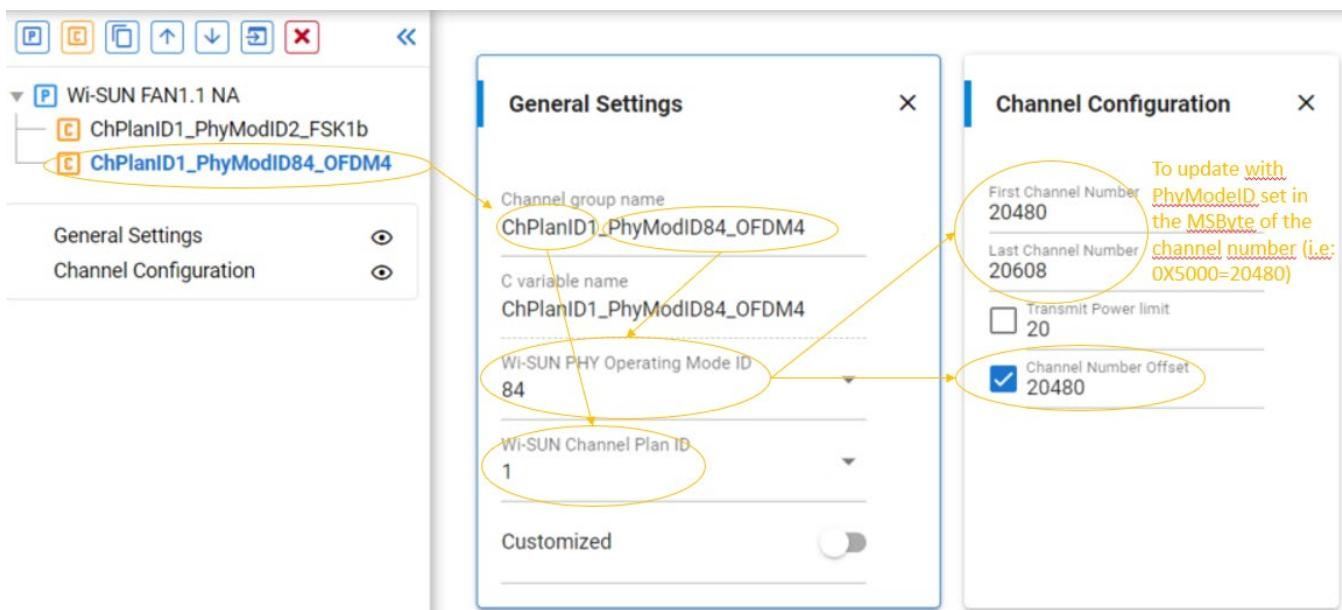
5. Add other channels and configure them as previously described for Mode Switch configuration. Use the following tables to compute the base channel number.
