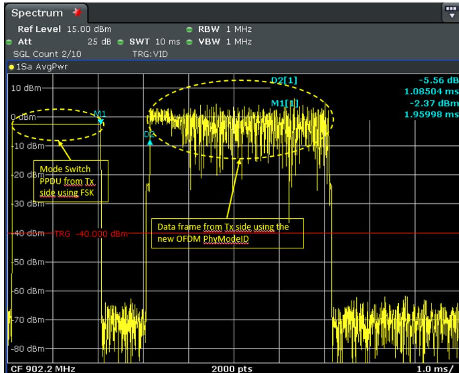
Note: After the Mode Switch PPDU, the data frame might use another carrier frequency. The resolution bandwidth (RBW) of the spectrum analyzer should be set according to this new frequency, so that zero span can detect the data frame transmitted.
