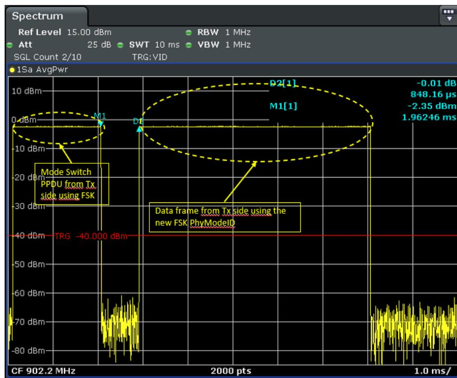
The following illustrates a Mode Switch from FSK to OFDM PhyModelID with CSMA-CA enabled.
