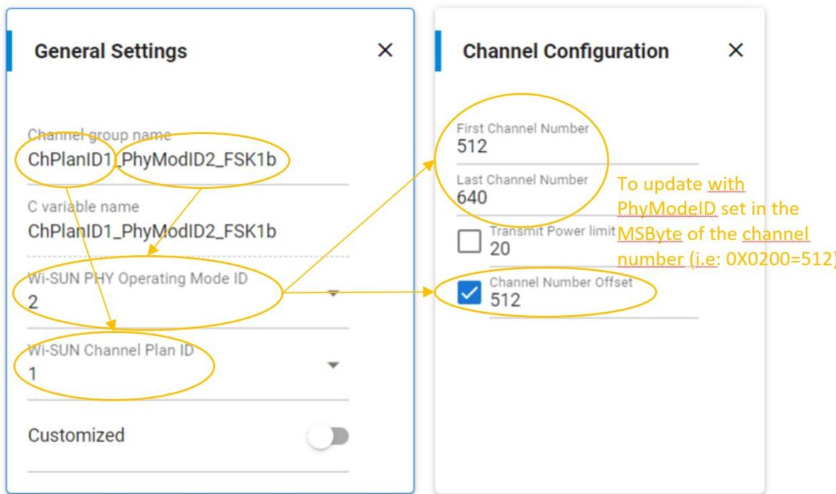
Note: The Wi-SUN Channel Plan ID list proposed depends on the Wi-SUN Regulatory Domain and on the selected Wi-SUN PHY Mode ID. The Wi-SUN Channel Plan ID selected supports automatically getting the base frequency and the channel spacing according to the Wi-SUN FAN 1.1 specification.
