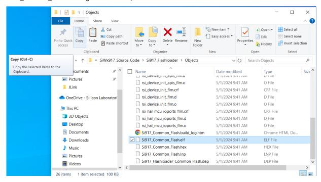
2. Paste the copied Si917\_Common\_Flash.elf file in the path: [Installed\_Path]/SEGGER/Jlink as shown below.
