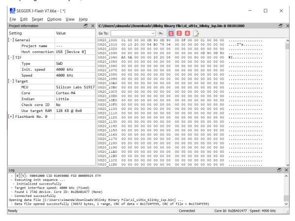
12. To flash the blinky application onto the SiWx917 device, click on Target → Manual Programming → Program.
