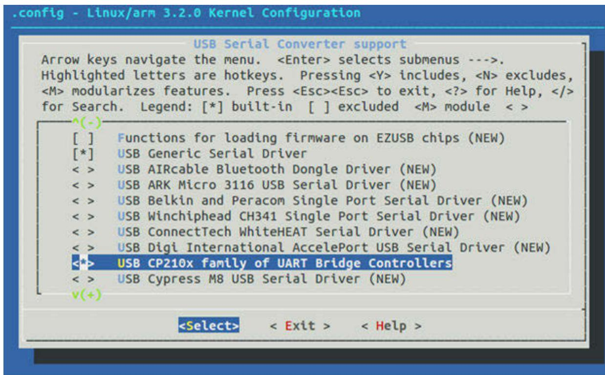
Figure 6.4. menuconfig: USB Serial Converter Features
