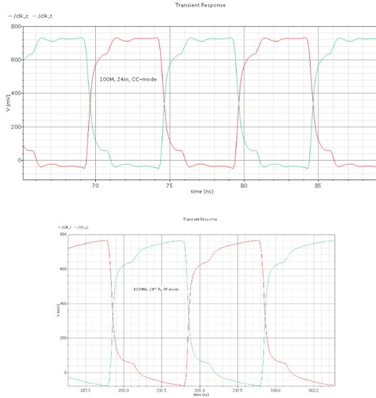
Figure 4.1. Simulated Waveforms Driving 24", 100 Ω Differential, Lossy Microstrip
