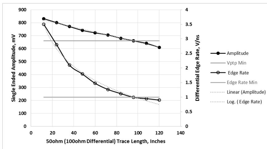
**Figure 5.1. Push-Pull Driver Signal Degradation vs. Line Length**
