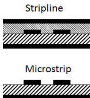
**Figure 3.2. Two Types of Differential Clock Traces**
