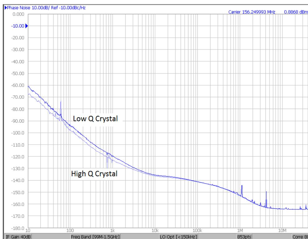
Figure 3. Si5345 156.250 MHz Phase Noise Using a High Q vs. Low Q 48.000 MHz Crystal
