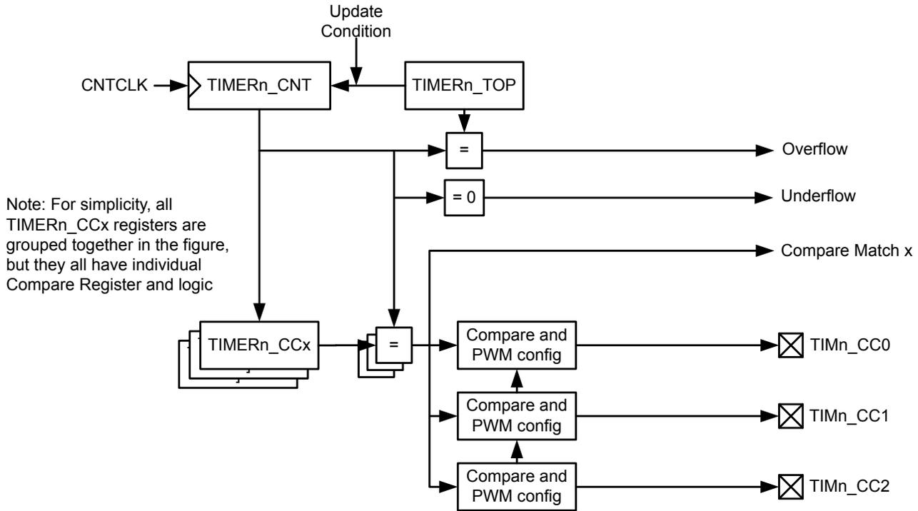
**Figure 19.14. TIMER/WTIMER Block Diagram Showing Comparison Functionality**
