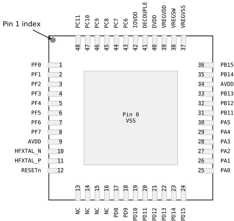
Figure 6.2. EFM32PG12B5xx in QFN48 Device Pinout
