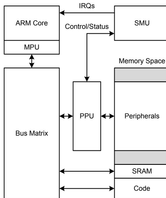
**Figure 11.1. Bus-Level Security System View**
