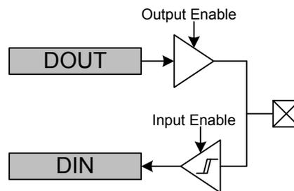
**Figure 31.3. Push-Pull Configuration**
