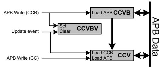
**Figure 19.16. TIMER/WTIMER Output Compare/PWM Buffer Functionality Detail**
