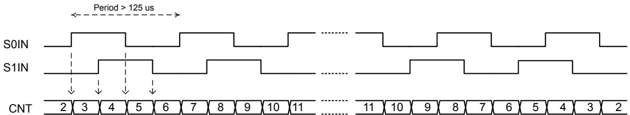
Figure 15.6. PCNT Oversampling Quadrature Decoder 4X mode
