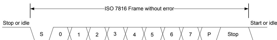
**Figure 17.15. USART ISO 7816 Data Frame Without Error**
