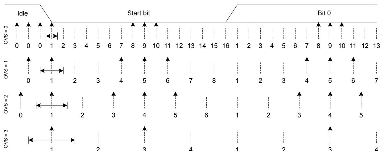
**Figure 17.7. USART Sampling of Start and Data Bits**
