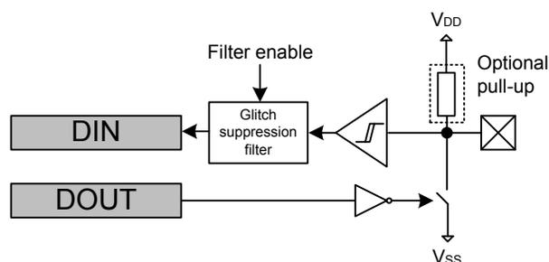
Figure 31.4. Open-drain
