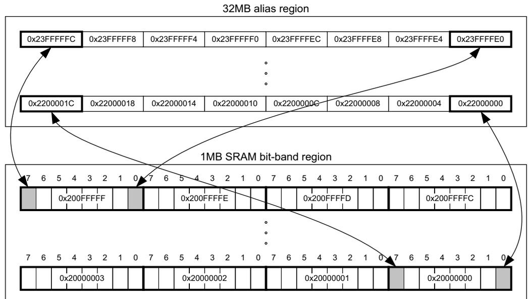
Figure 2-1 Bit-band mapping
