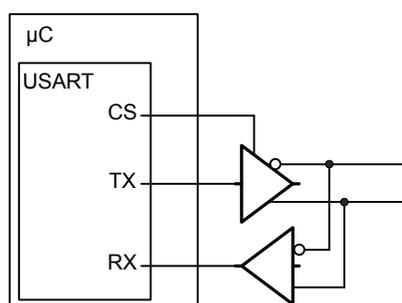
**Figure 17.10. USART Half Duplex Communication with External Driver**
