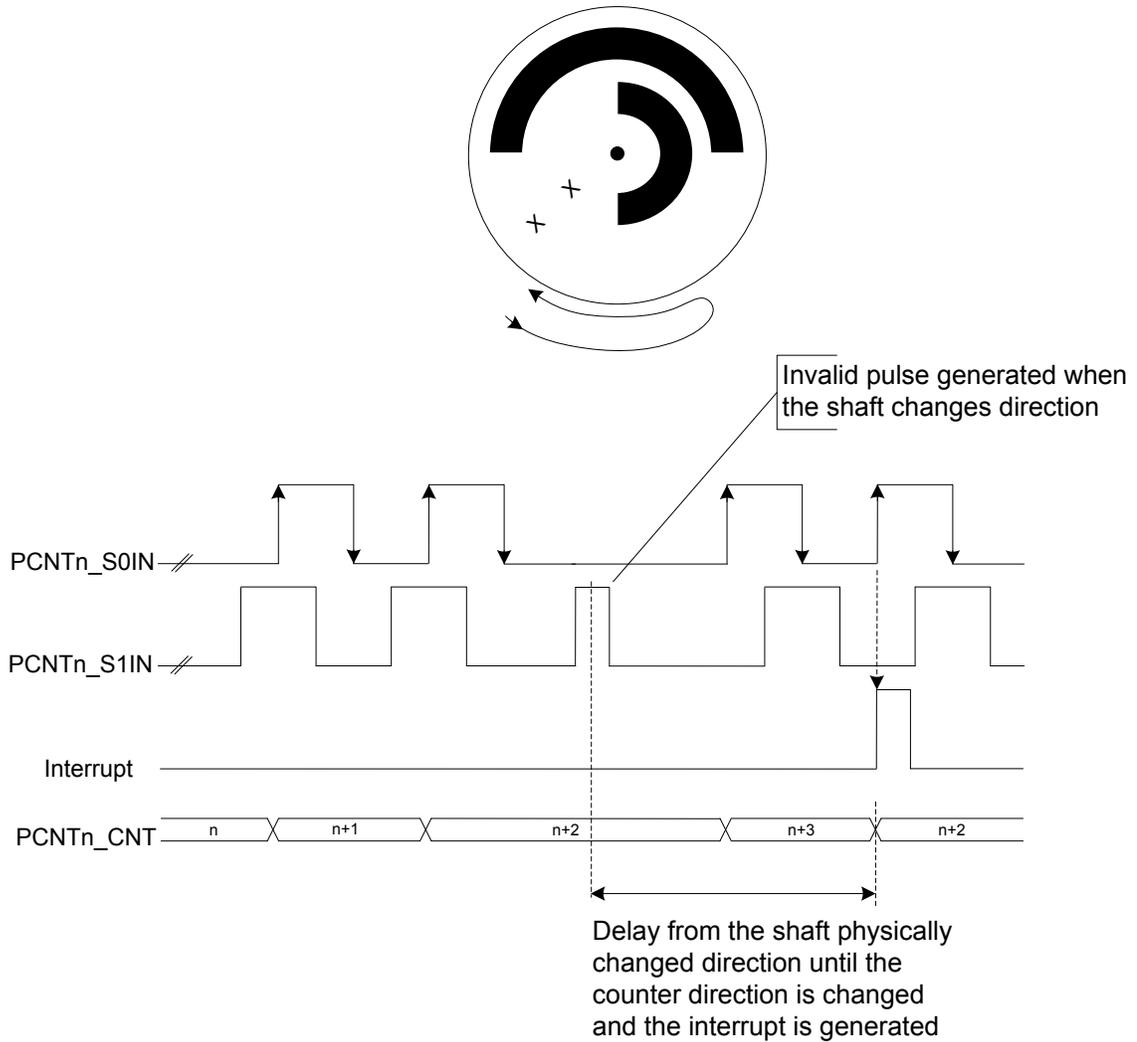
**Figure 15.13. PCNT Direction Change Interrupt (DIRCNG) Generation**
