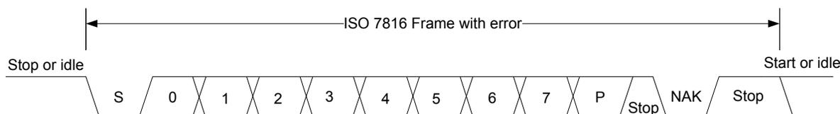
**Figure 17.16. USART ISO 7816 Data Frame With Error**
