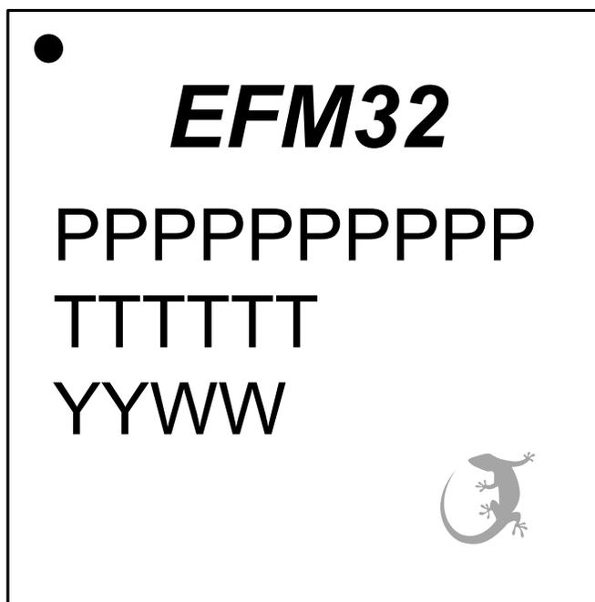
**Figure 7.3. BGA125 Package Marking**
