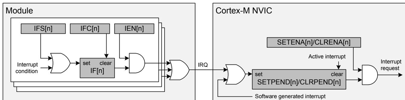
Figure 3.1. Interrupt Operation
