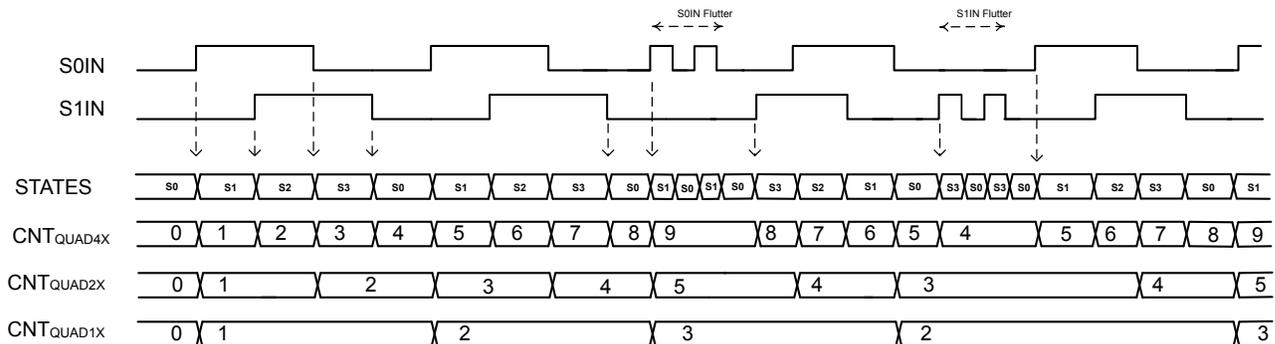
Figure 15.7. PCNT Oversampling Quadrature Decoder with Flutter Removal
