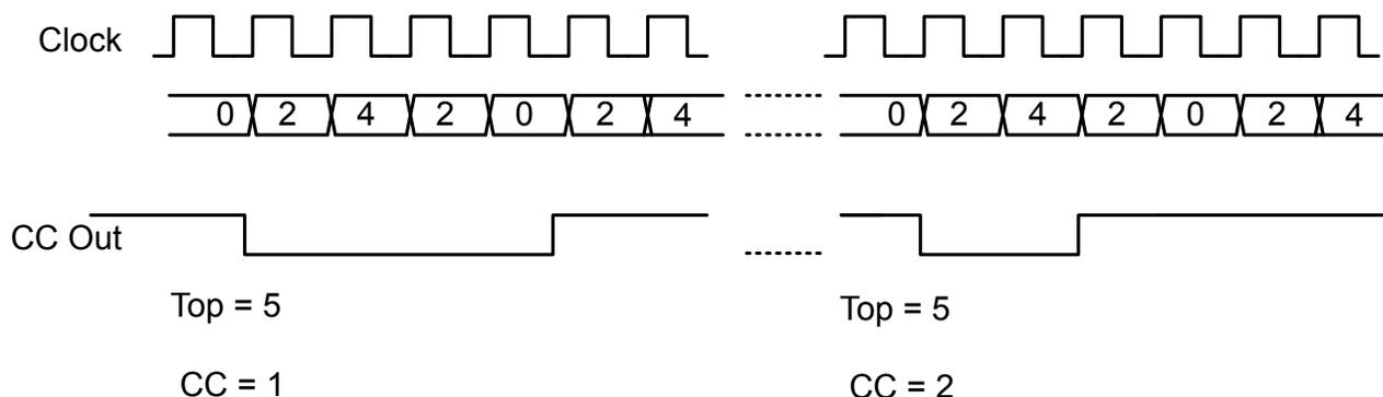
**Figure 19.34. TIMER/WTIMER CC out in 2x mode**
