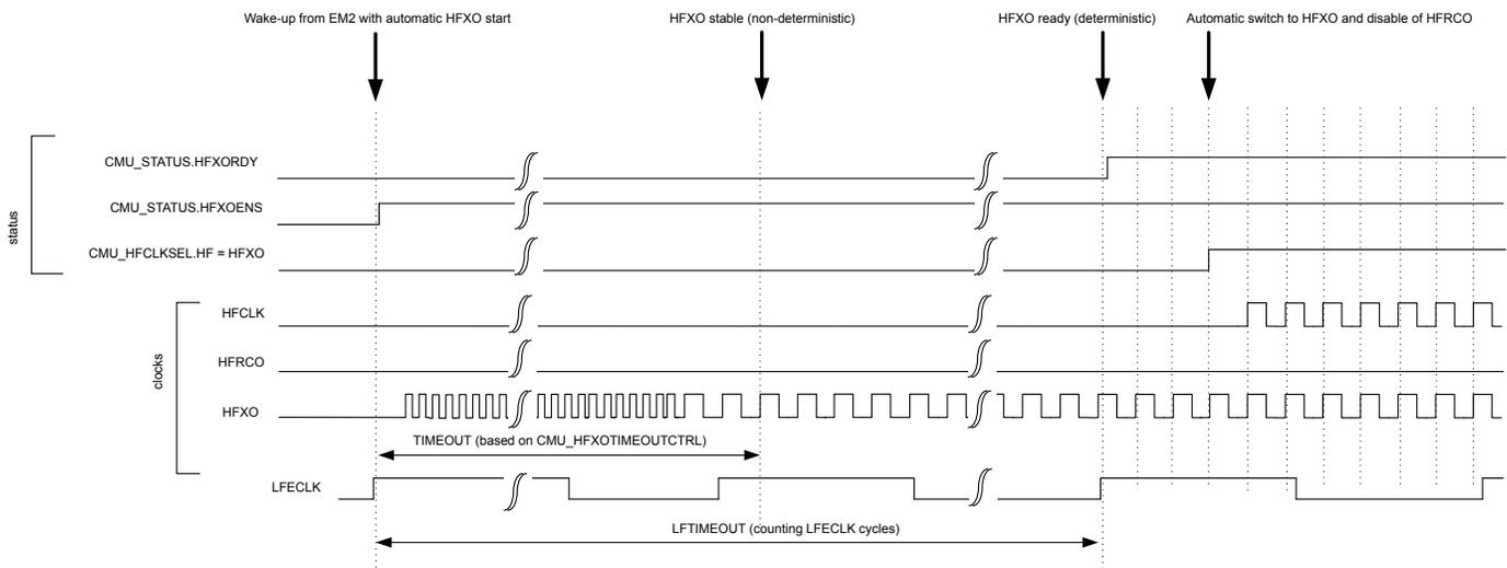
**Figure 10.3. CMU Deterministic HFXO startup using LFTIMEOUT**
