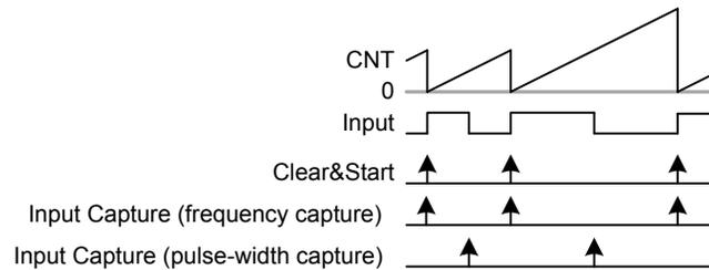
**Figure 19.13. TIMER/WTIMER Period and/or Pulse width Capture**
