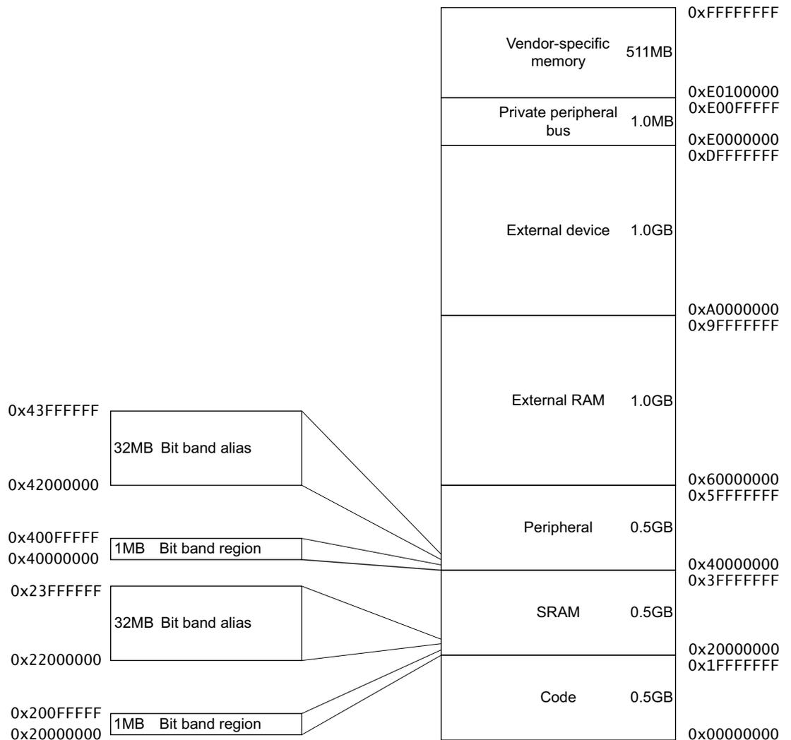
The regions for SRAM and peripherals include optional bit-banding regions. Bit-banding provides atomic operations to bit data, see [Optional bit-banding on page 2-16](#).
