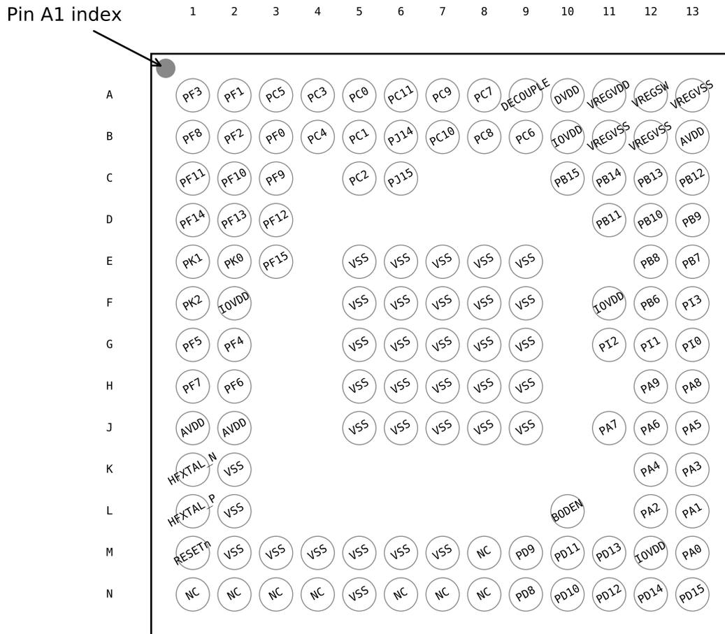
**Figure 6.1. EFM32PG12B5xx in BGA125 Device Pinout**
