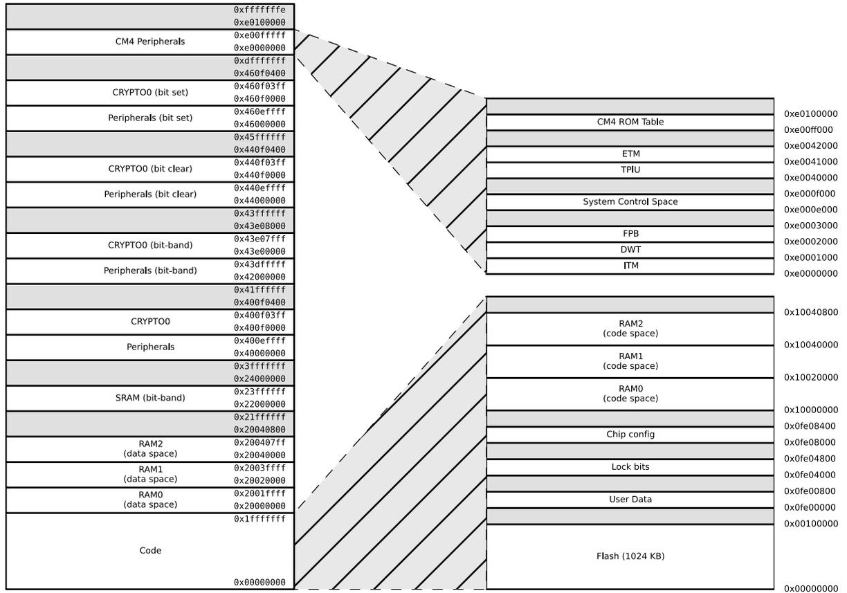
**Figure 4.2. System Address Space with Core and Code Space Listing**
