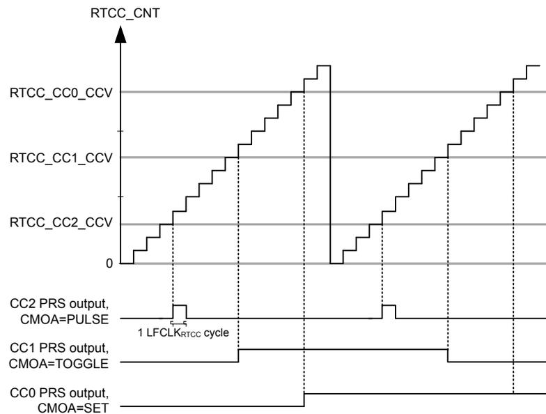
**Figure 12.3. RTCC Compare match and PRS output illustration**
