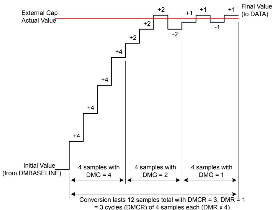
**Figure 33.2. Delta modulation conversion with gain reduction (DMGDIS = 0)**
