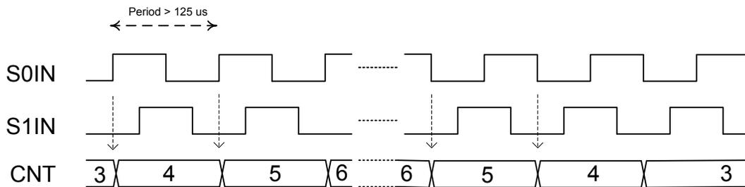
**Figure 15.4. PCNT Oversampling Quadrature Decoder 1X mode**
