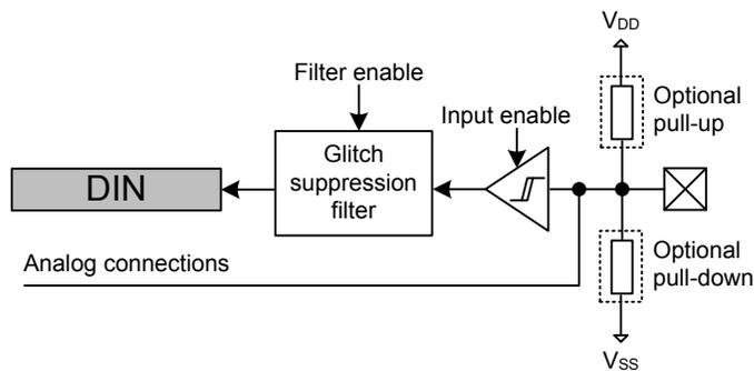
**Figure 31.2. Tristated Output with Optional Pull-up or Pull-down**
