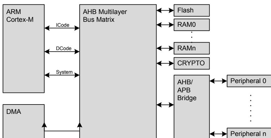
Figure 4.1. EFM32PG12 Pearl Gecko Bus System
