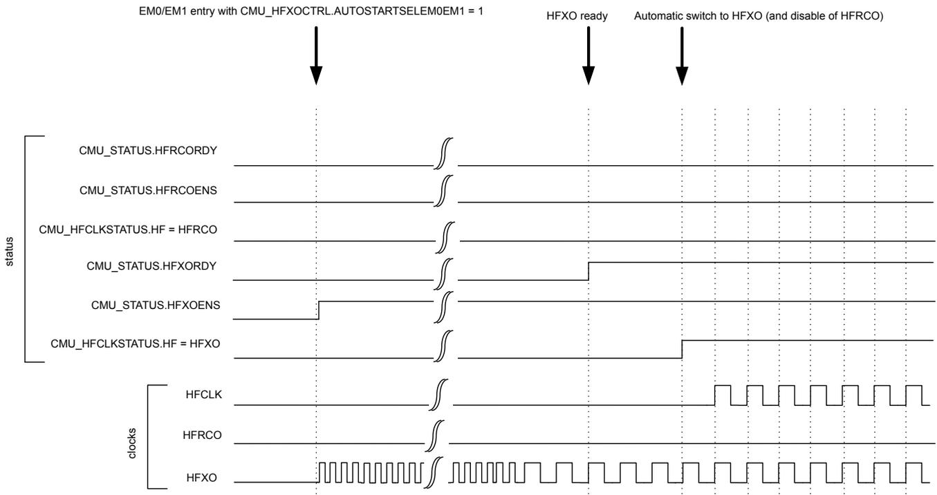
**Figure 10.13. CMU Automatic startup and selection of HFXO**
