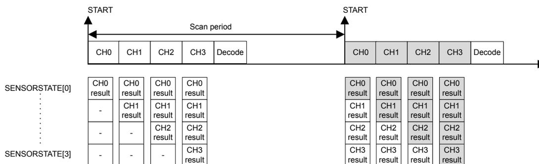
**Figure 27.10. Sensor scan and decode sequence**
