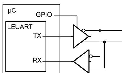
Figure 18.10. LEUART Half Duplex Communication with External Driver
