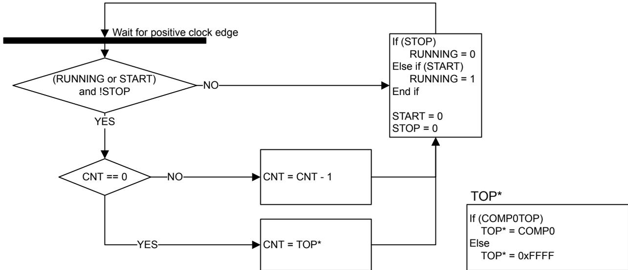
**Figure 20.2. LETIMER State Machine for Free-running Mode**
