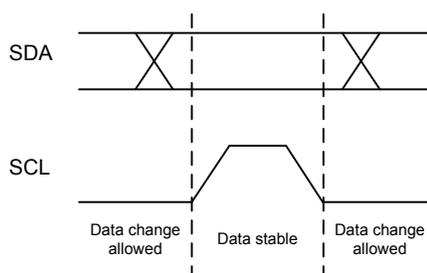
**Figure 16.5. I<sup>2</sup>C Bit Transfer on I<sup>2</sup>C-Bus**
