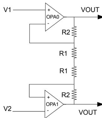
**Figure 23.11. Instrumentaion Amplifier Overview**
