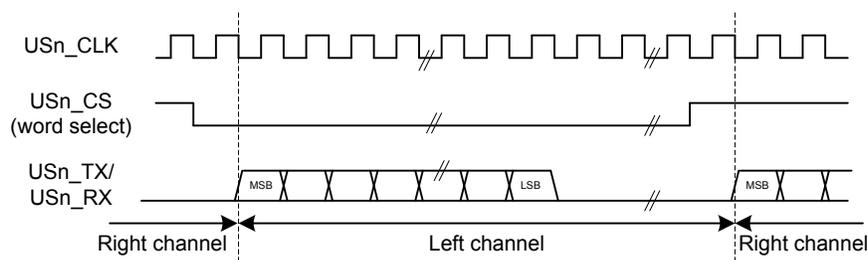
**Figure 17.22. USART Standard I2S waveform (reduced accuracy)**
