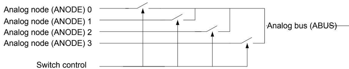
**Figure 32.1. Analog Bus (ABUS)**
