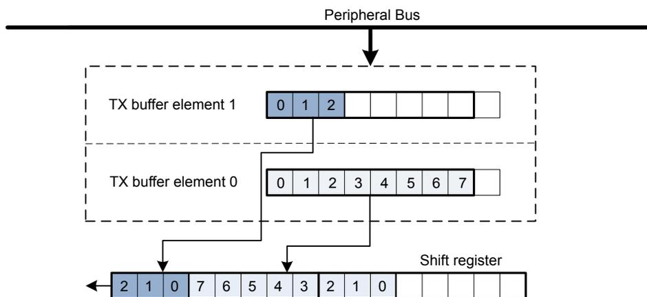
**Figure 17.12. USART Transmission of Large Frames, MSBF**
