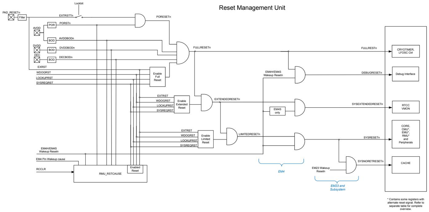
**Figure 8.1. RMU Reset Input Sources and Connections**
