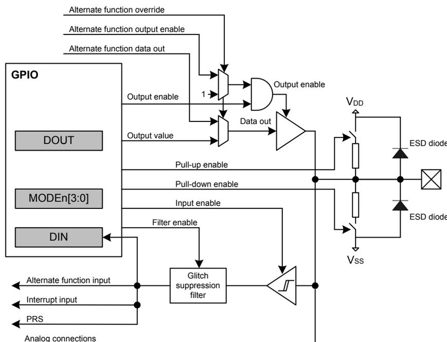
Figure 31.1. Pin Configuration
