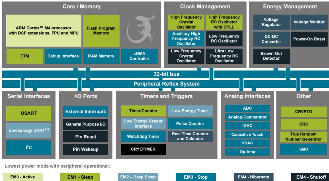
Figure 2.1. EFM32PG12 Pearl Gecko System-On-Chip Block Diagram
