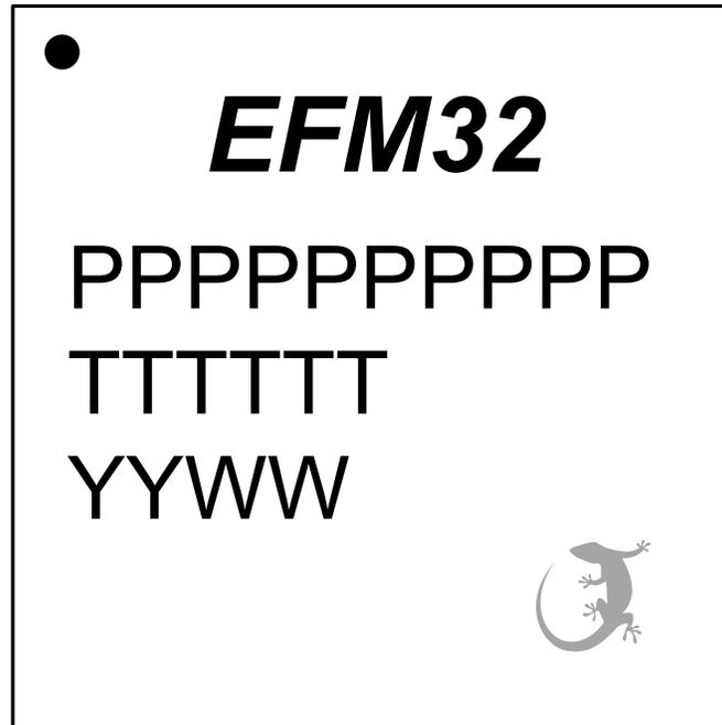
Figure 8.3. QFN48 Package Marking
