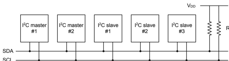
**Figure 16.2. I<sup>2</sup>C-Bus Example**
