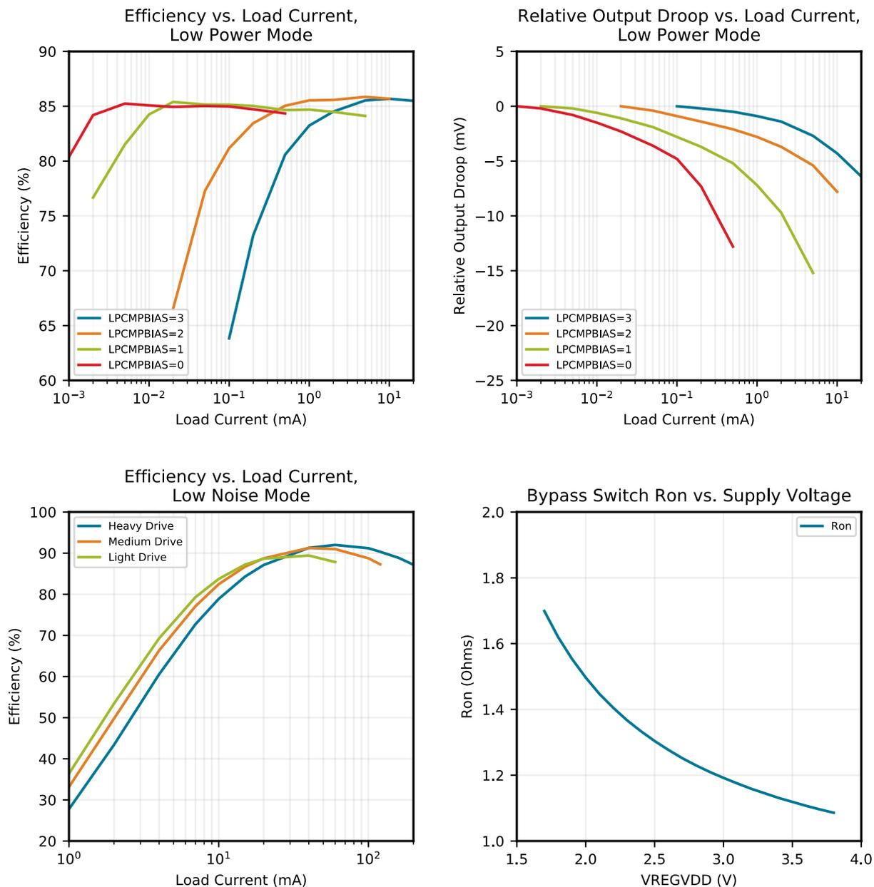
Figure 4.8. DC-DC Converter Typical Performance Characteristics
