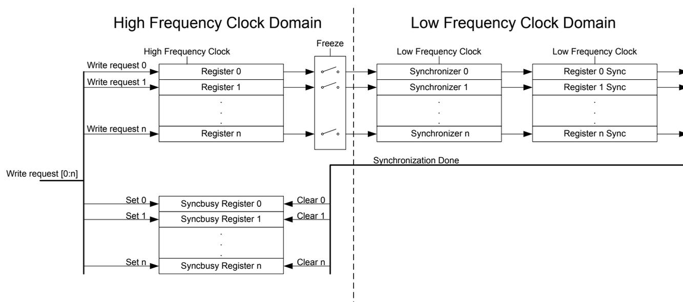
Figure 4.11. Write operation to Low Energy Peripherals
