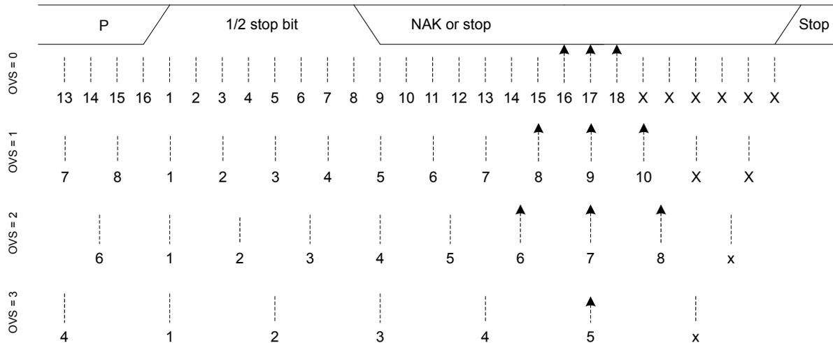
**Figure 17.17. USART SmartCard Stop Bit Sampling**
