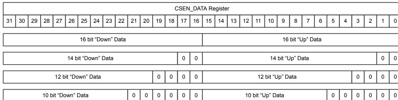
**Figure 33.8. Data encoding for delta modulation with chopping**
