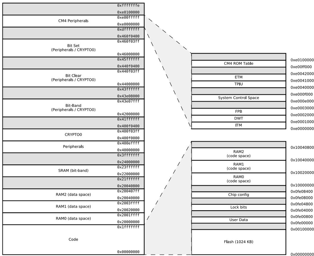
Figure 3.2. EFM32PG12 Memory Map — Core Peripherals and Code Space
