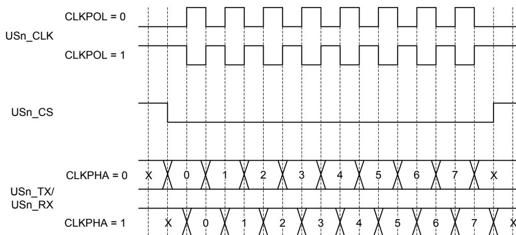
Figure 17.20. USART SPI Timing
