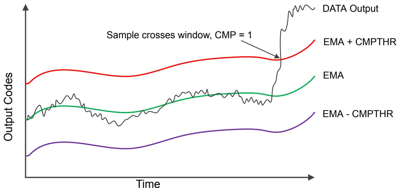
Figure 33.10. Wake on Threshold With Relative EMA
