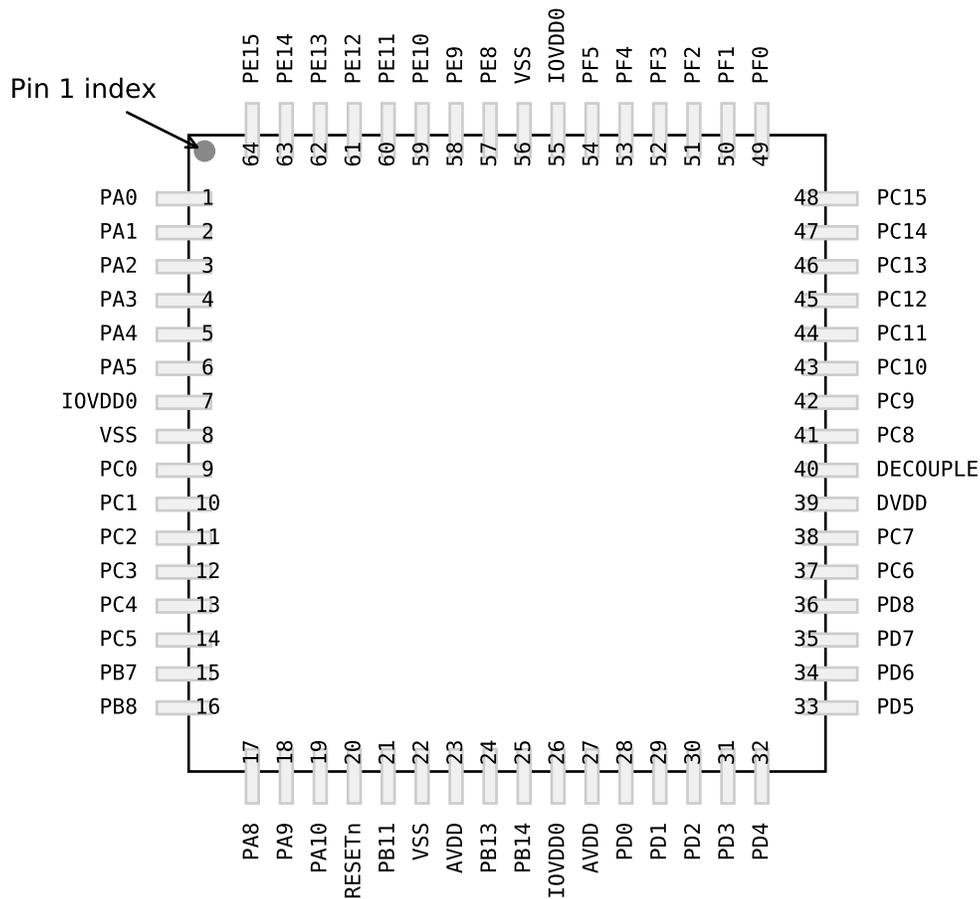
Figure 5.15. EFM32GG12B1xx in QFP64 Device Pinout
