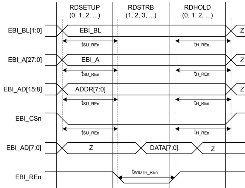
Figure 4.5. EBI Read Enable Output Timing Diagram
