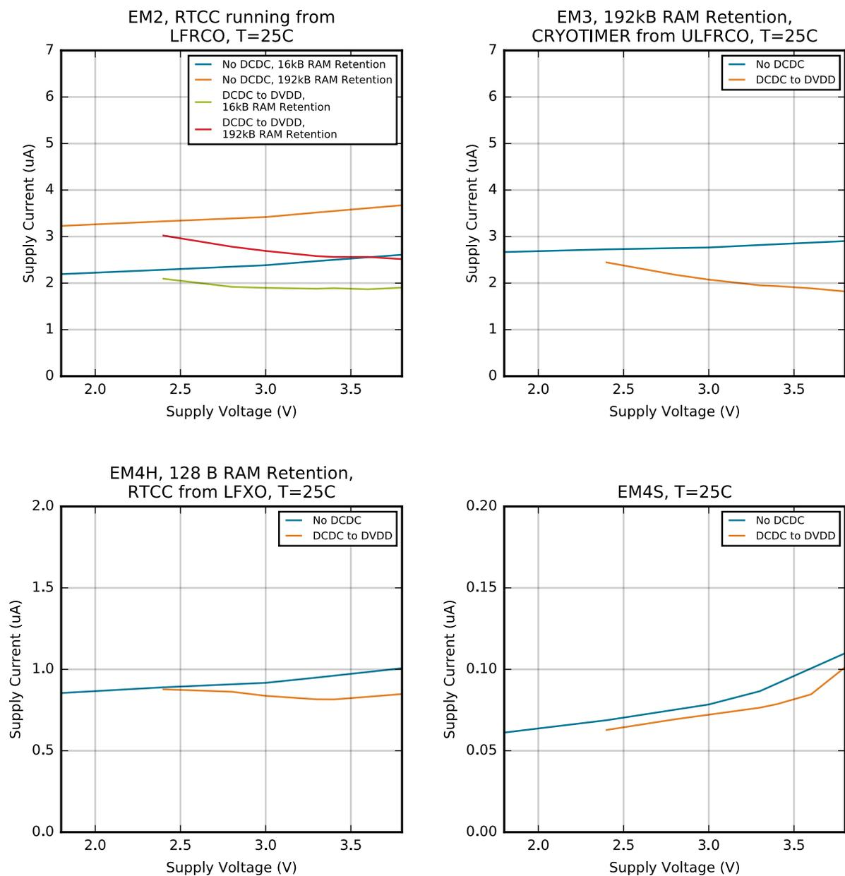
Figure 4.27. EM2, EM3, EM4H and EM4S Typical Supply Current vs. Supply
