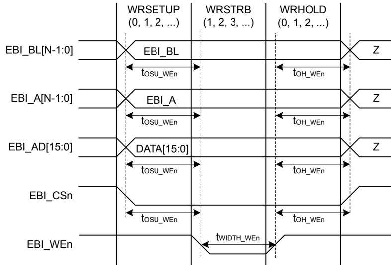
Figure 4.3. EBI Write Enable Output Timing Diagram
