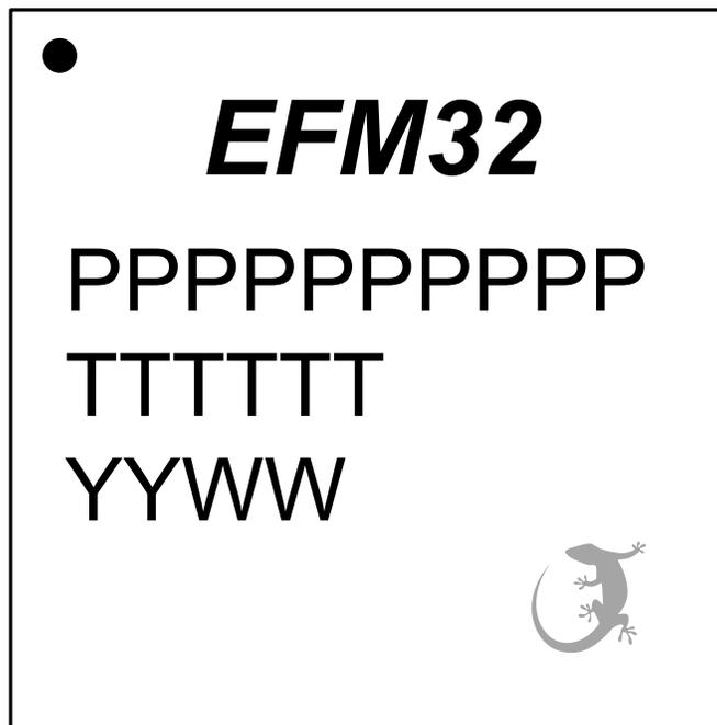
**Figure 8.3. TQFP100 Package Marking**
