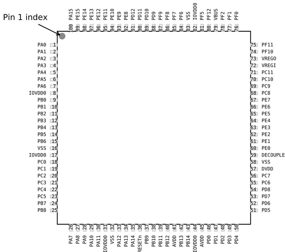
Figure 5.10. EFM32GG12B4xx in QFP100 Device Pinout
