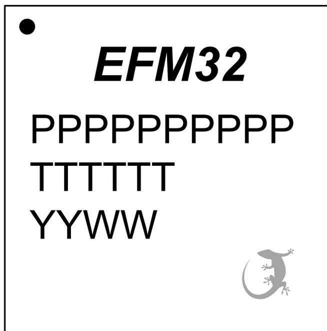
Figure 6.3. BGA120 Package Marking
