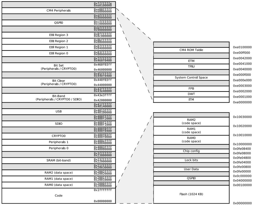
Figure 3.2. EFM32GG12 Memory Map — Core Peripherals and Code Space
