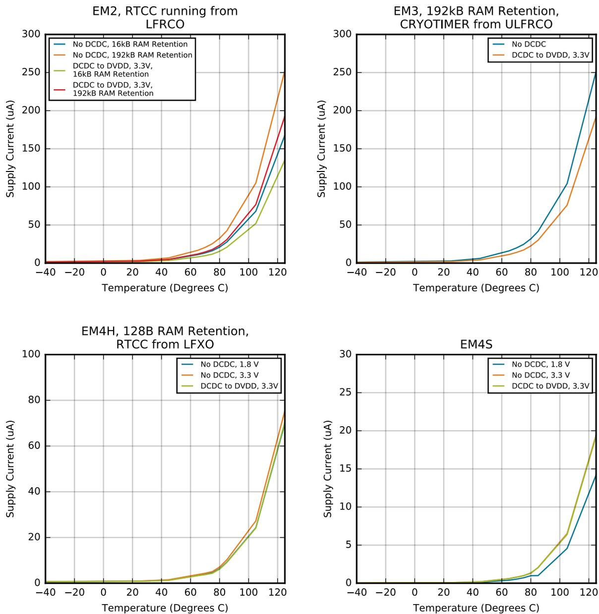
Figure 4.25. EM2, EM3, EM4H and EM4S Typical Supply Current vs. Temperature
