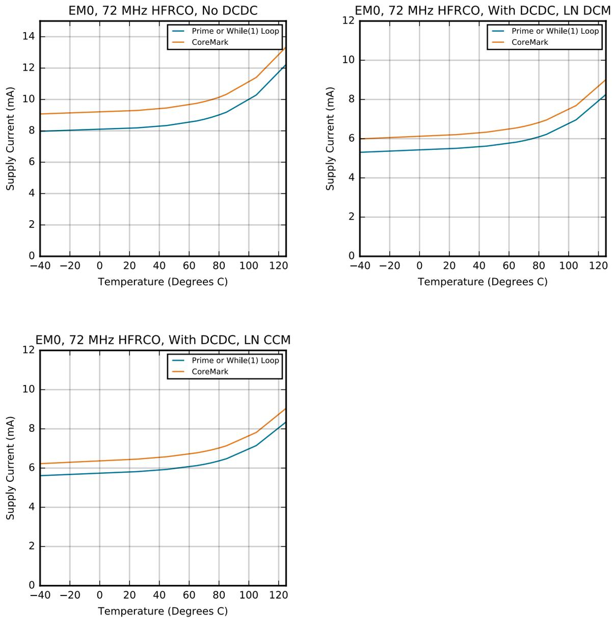
Figure 4.22. EM0 Full Speed Active Mode Typical Supply Current vs. Temperature
