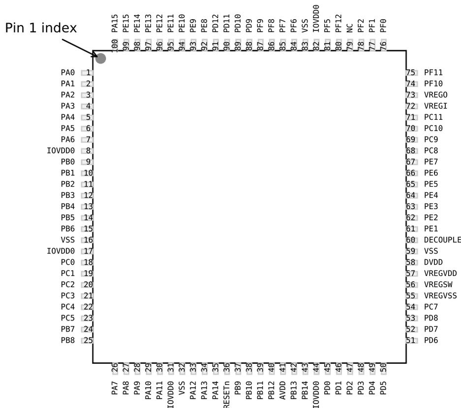
Figure 5.9. EFM32GG12B5xx in QFP100 Device Pinout
