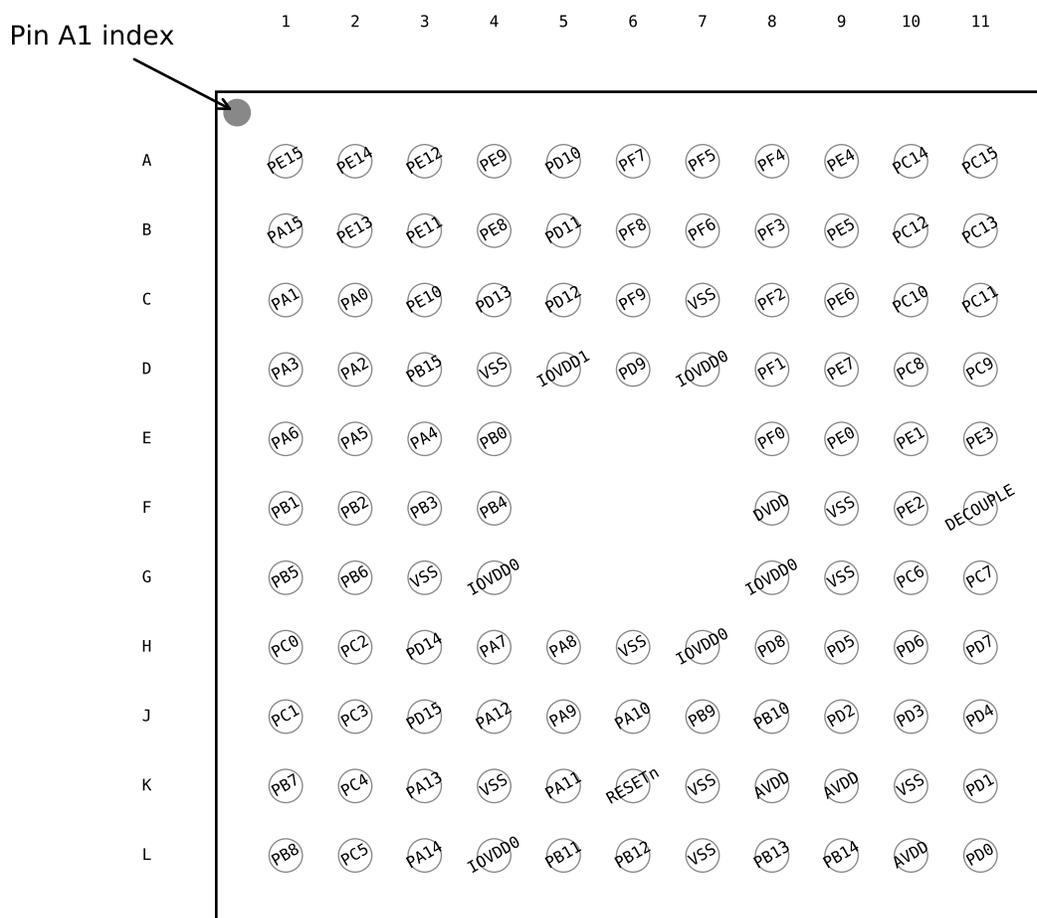
**Figure 5.7. EFM32GG12B3xx in BGA112 Device Pinout**
