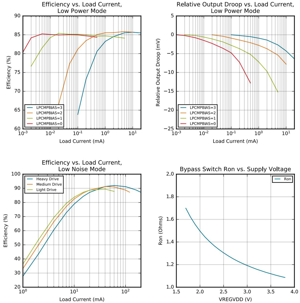
Figure 4.28. DC-DC Converter Typical Performance Characteristics
