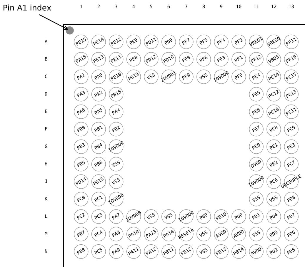
**Figure 5.3. EFM32GG12B4xx in BGA120 Device Pinout**
