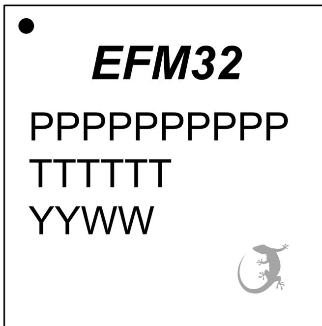
**Figure 9.3. TQFP64 Package Marking**
