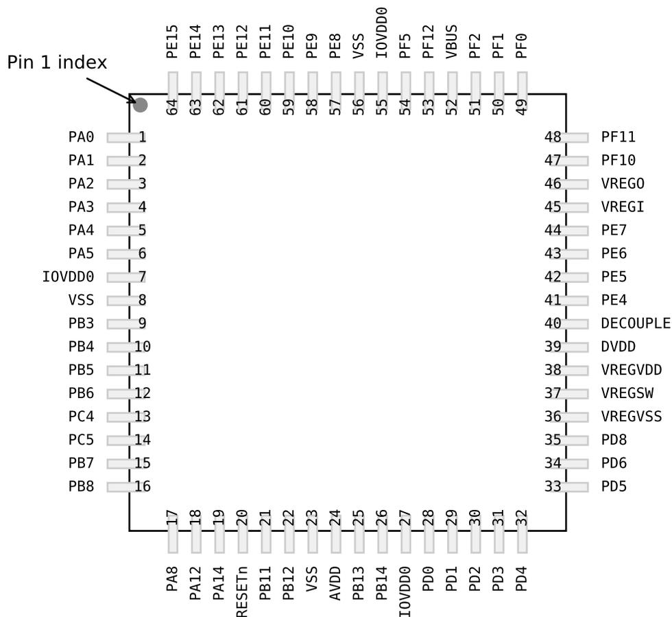
Figure 5.12. EFM32GG12B8xx in QFP64 Device Pinout
