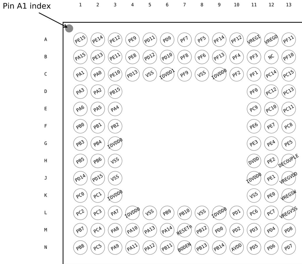
Figure 5.2. EFM32GG12B5xx in BGA120 Device Pinout
