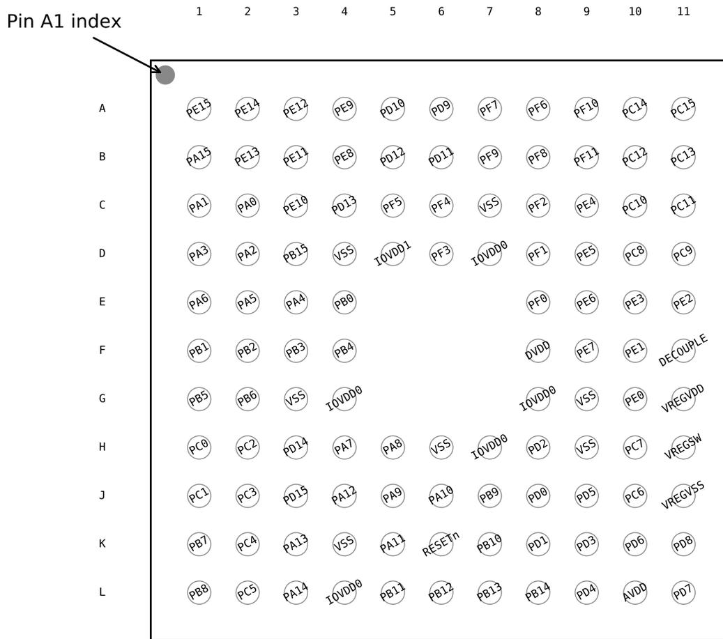
**Figure 5.5. EFM32GG12B5xx in BGA112 Device Pinout**
