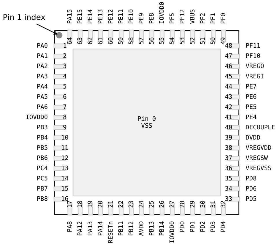
Figure 5.16. EFM32GG12B8xx in QFN64 Device Pinout
