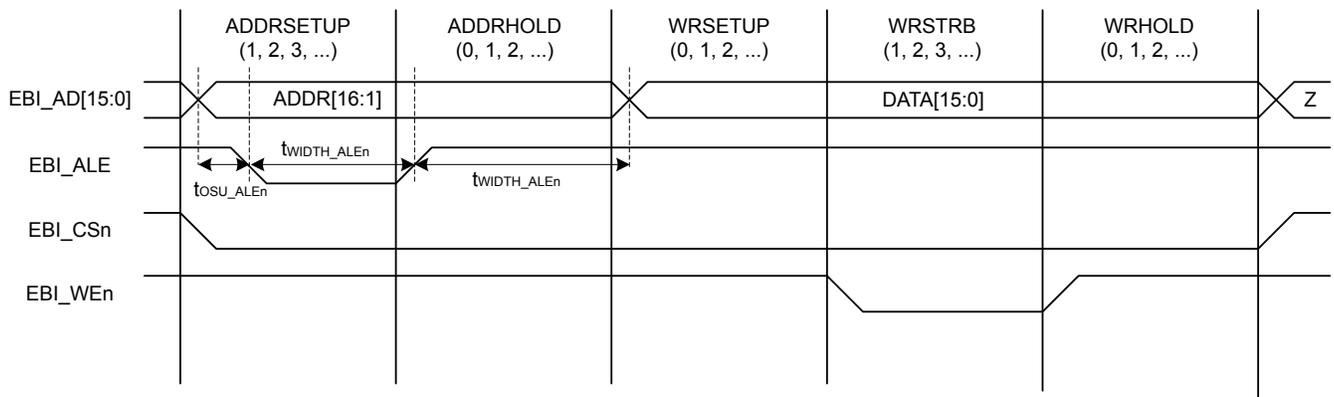
Figure 4.4. EBI Address Latch Enable Output Timing Diagram
