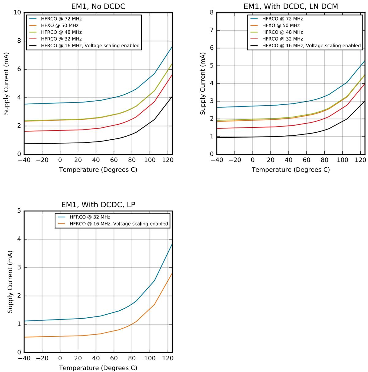
**Figure 4.24. EM1 Sleep Mode Typical Supply Current vs. Temperature**
