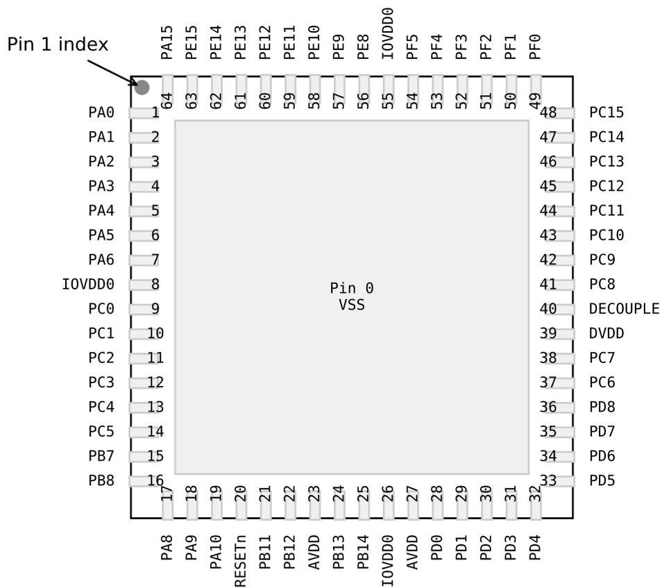
**Figure 5.19. EFM32GG12B1xx in QFN64 Device Pinout**
