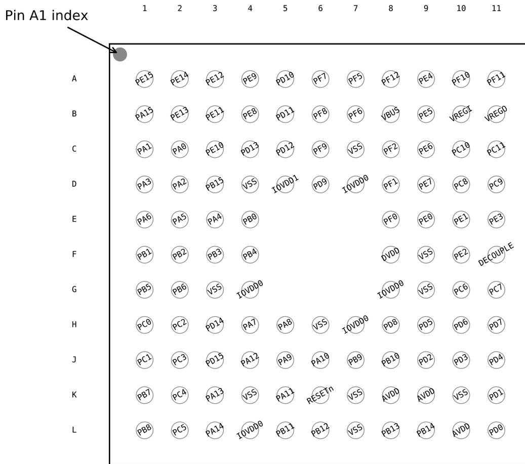
**Figure 5.6. EFM32GG12B4xx in BGA112 Device Pinout**
