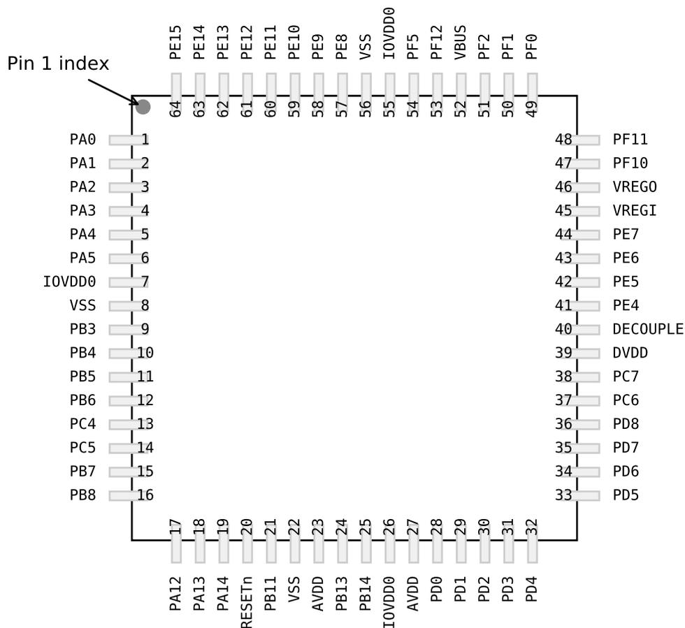
Figure 5.14. EFM32GG12B4xx in QFP64 Device Pinout
