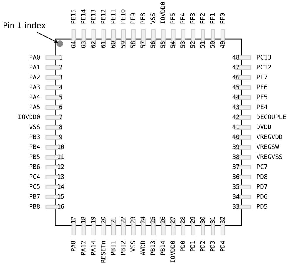
Figure 5.13. EFM32GG12B5xx in QFP64 Device Pinout
