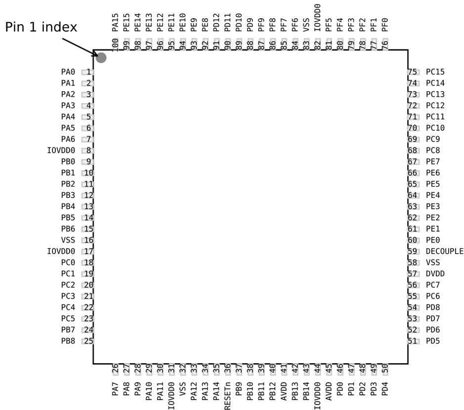
Figure 5.11. EFM32GG12B3xx in QFP100 Device Pinout
