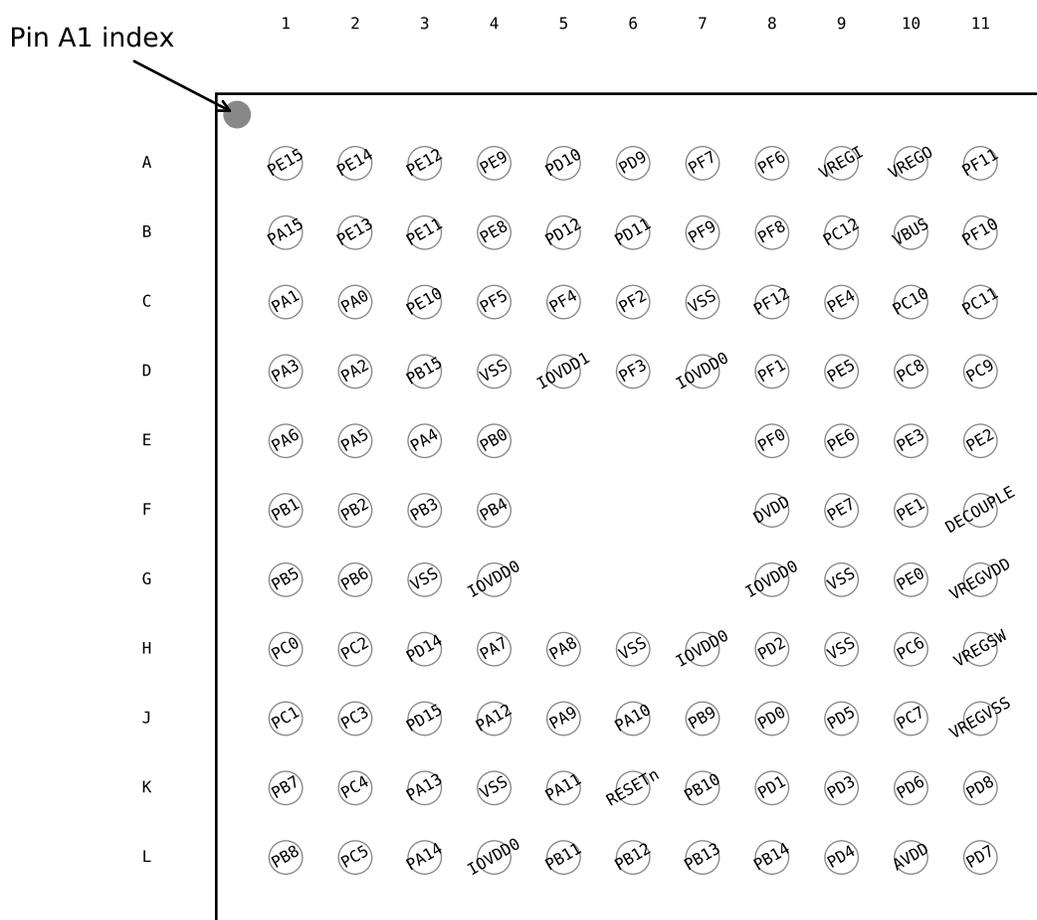
**Figure 5.4. EFM32GG12B8xx in BGA112 Device Pinout**
