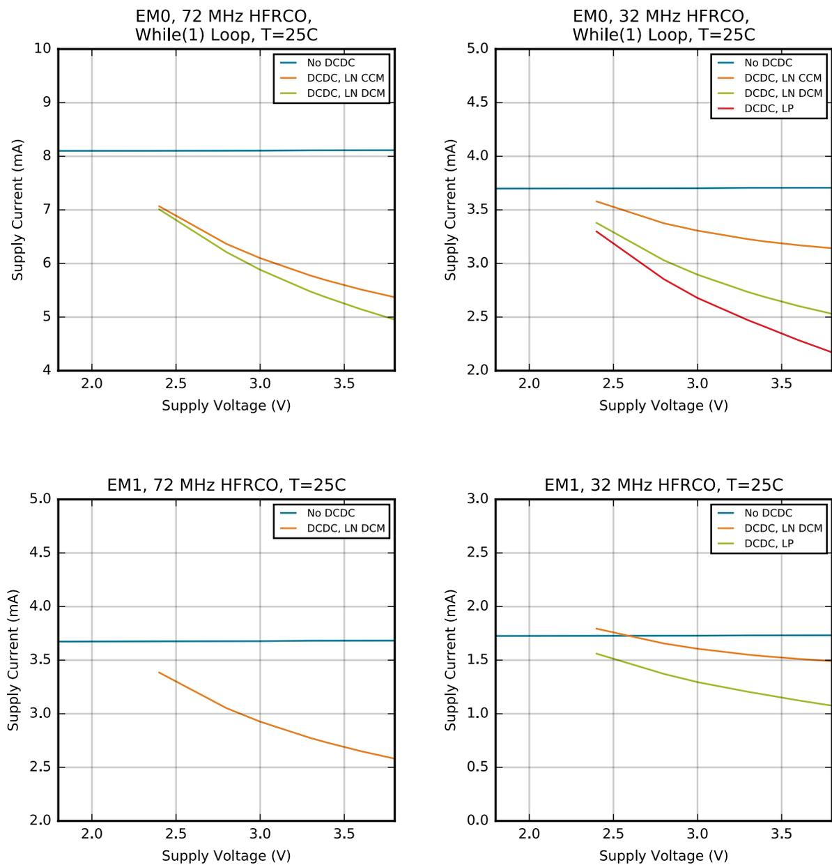
Figure 4.26. EM0 and EM1 Mode Typical Supply Current vs. Supply
