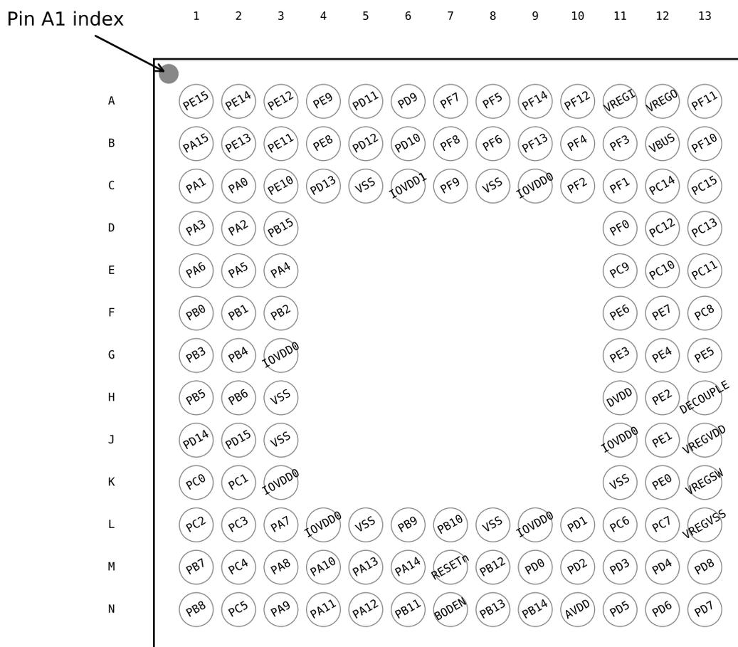
Figure 5.1. EFM32GG12B8xx in BGA120 Device Pinout
