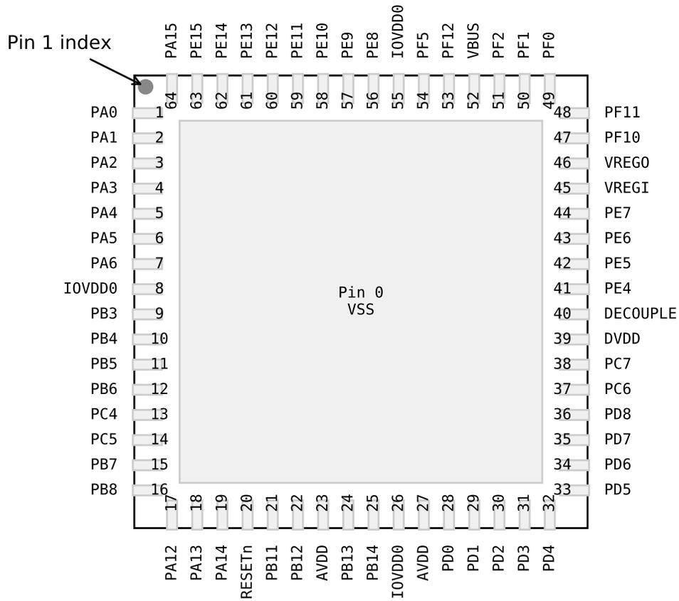
Figure 5.18. EFM32GG12B4xx in QFN64 Device Pinout
