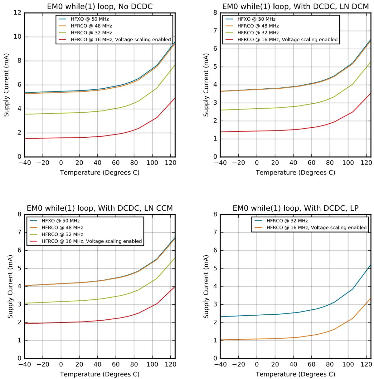
Figure 4.23. EM0 Active Mode Typical Supply Current vs. Temperature
