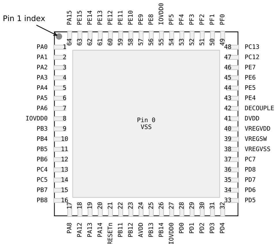
Figure 5.17. EFM32GG12B5xx in QFN64 Device Pinout
