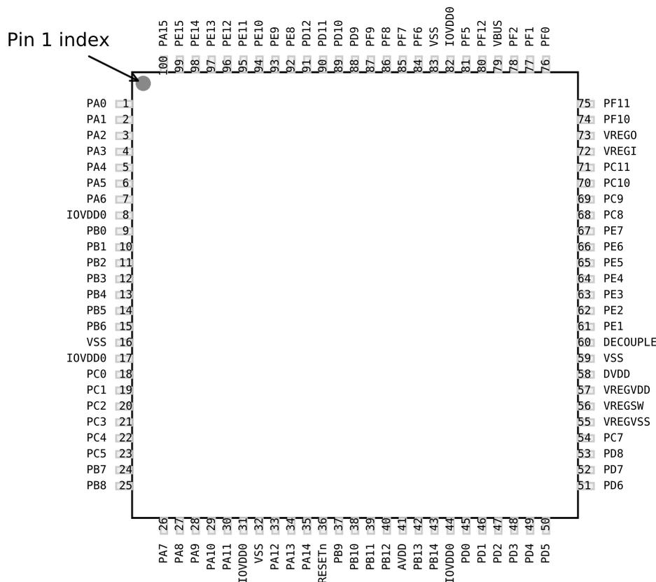
Figure 5.8. EFM32GG12B8xx in QFP100 Device Pinout
