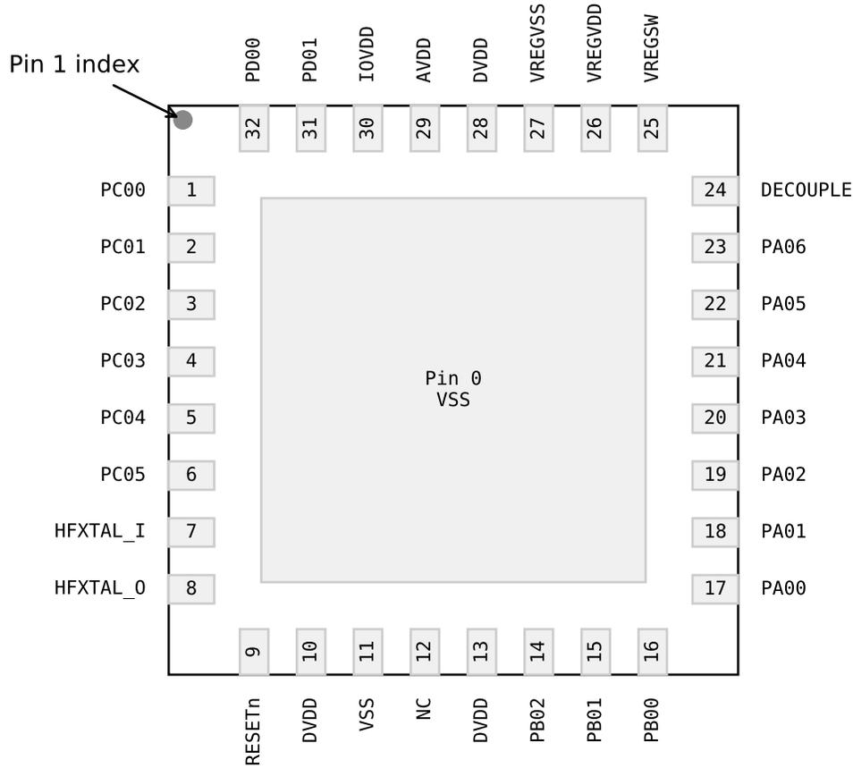
Figure 6.1. QFN32 Device Pinout
