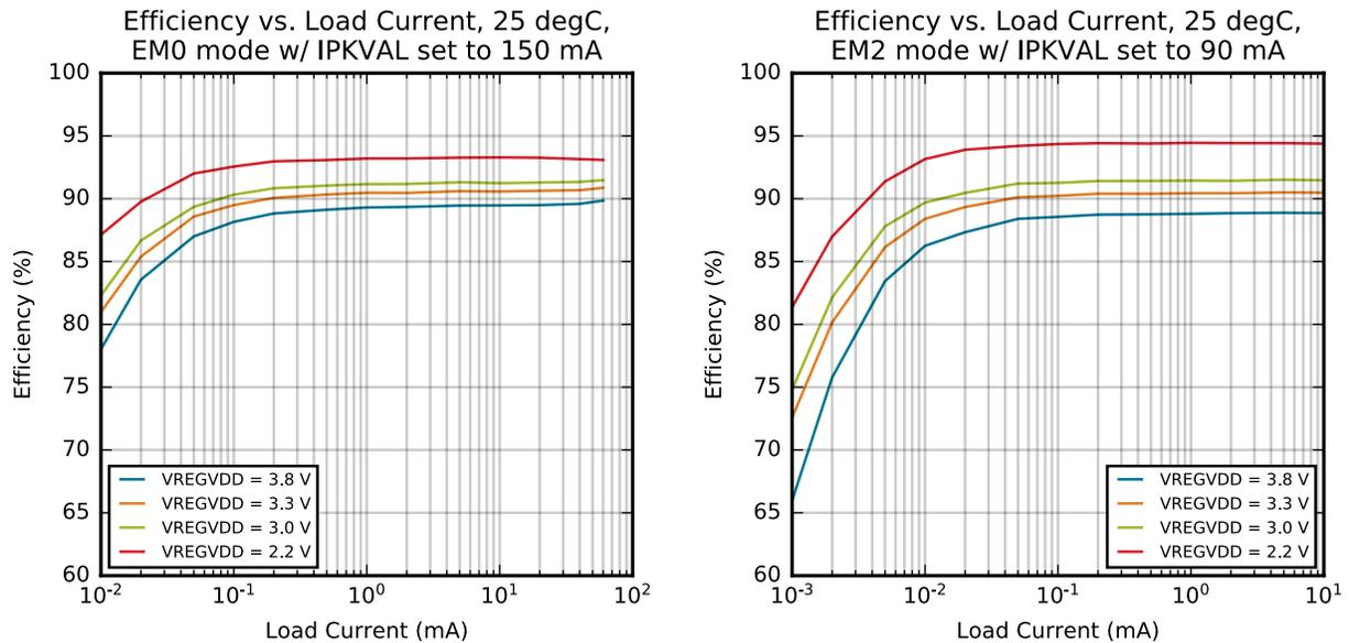
Figure 4.9. DC-DC Efficiency
