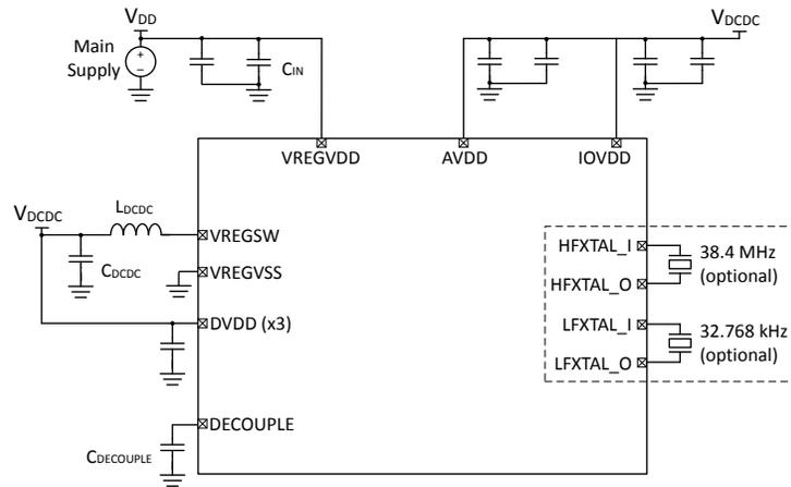
Figure 5.3. EFM32PG22 Typical Application Circuit: DCDC Configuration, AVDD and IOVDD from DCDC output
