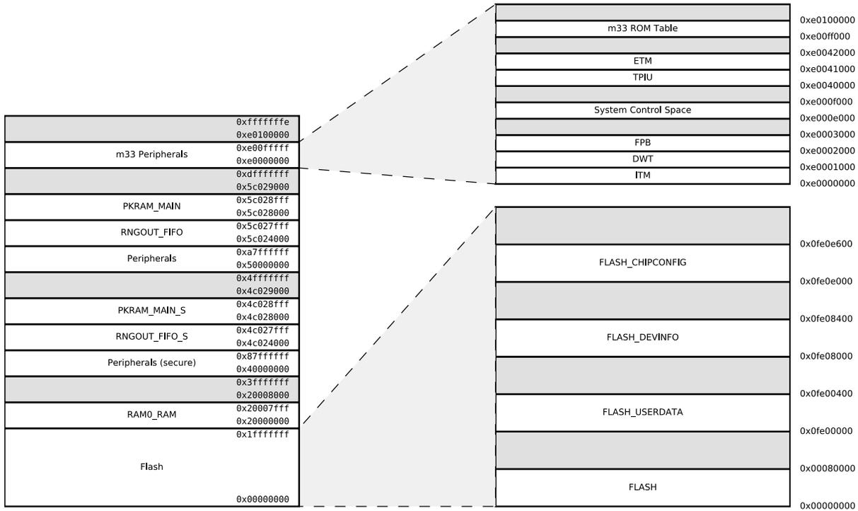
Figure 3.2. EFM32PG22 Memory Map — Core Peripherals and Code Space
