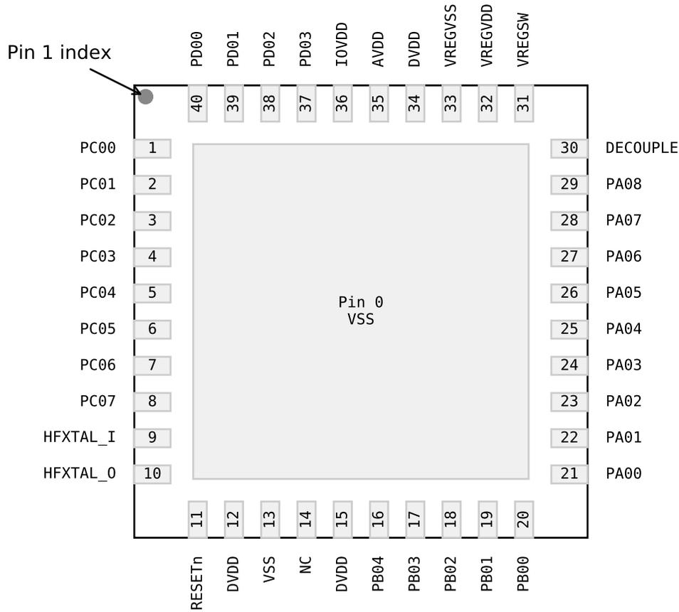
Figure 6.2. QFN40 Device Pinout
