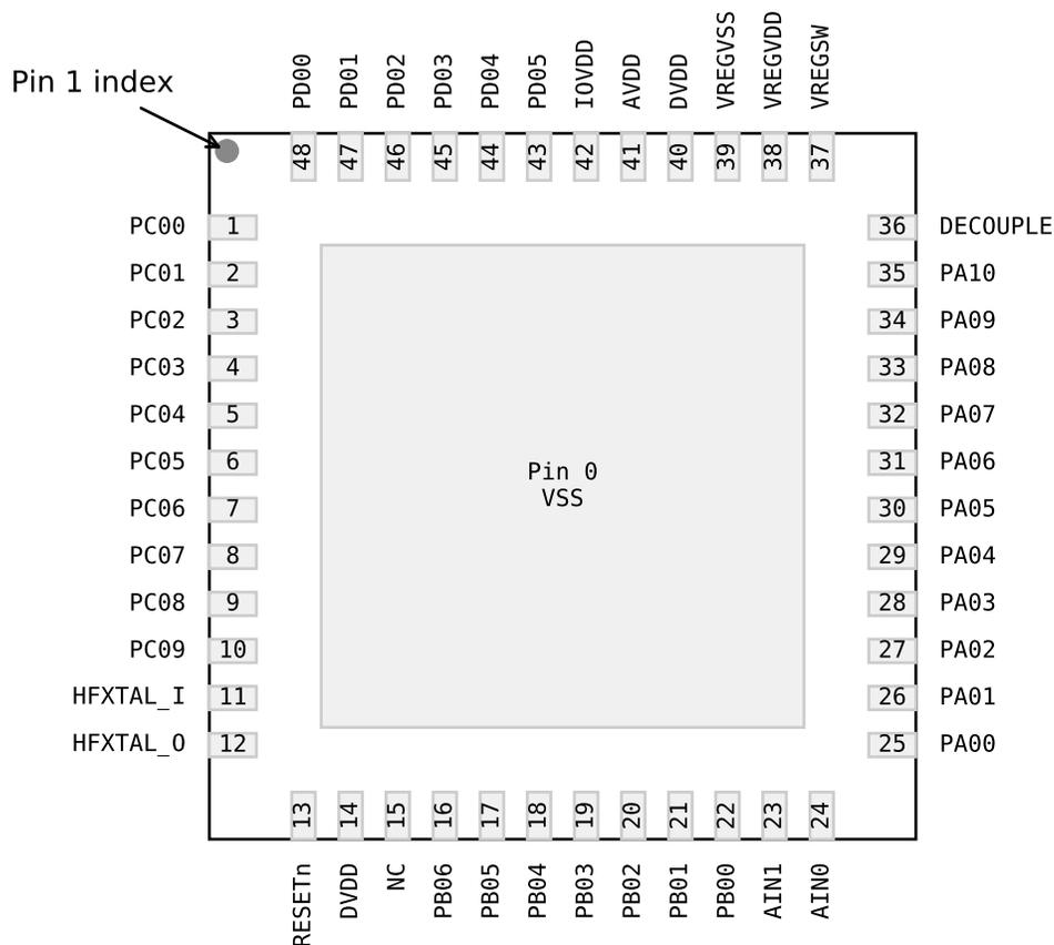
**Figure 6.1. QFN48 Device Pinout**
