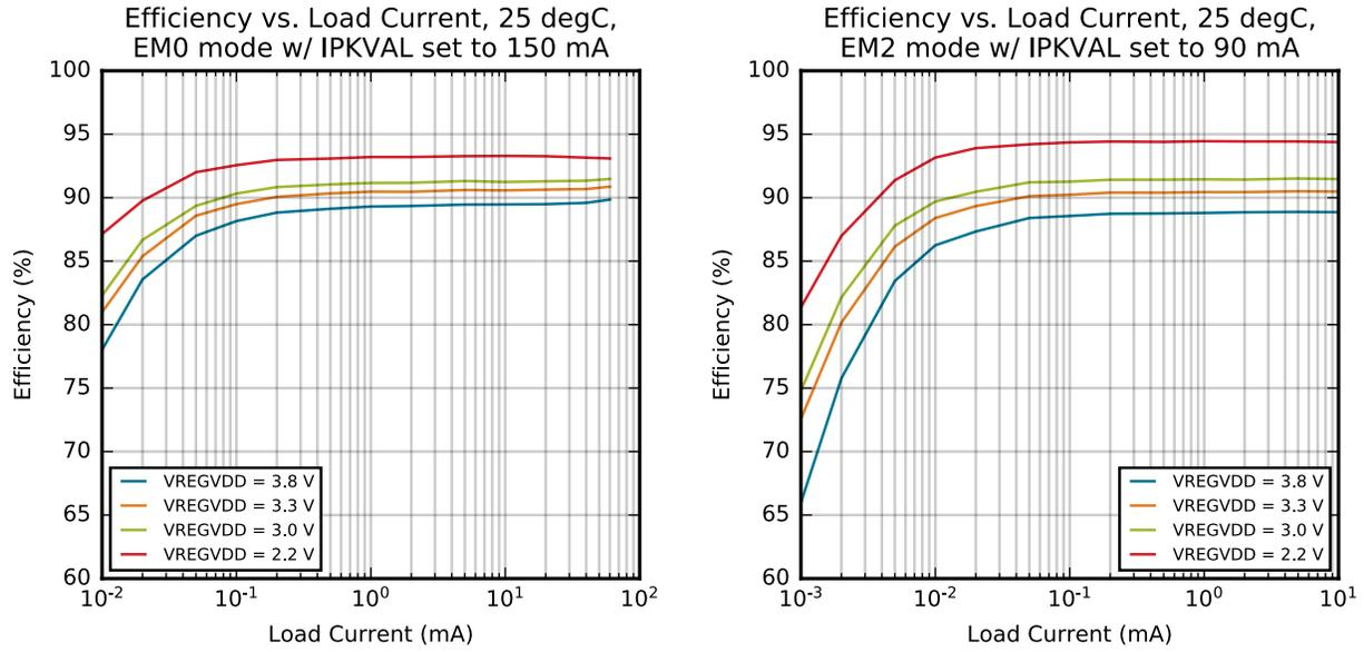
Figure 4.9. DC-DC Efficiency
