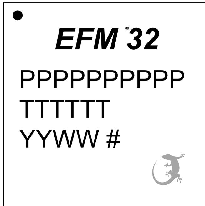
Figure 8.3. QFN48 Package Marking
