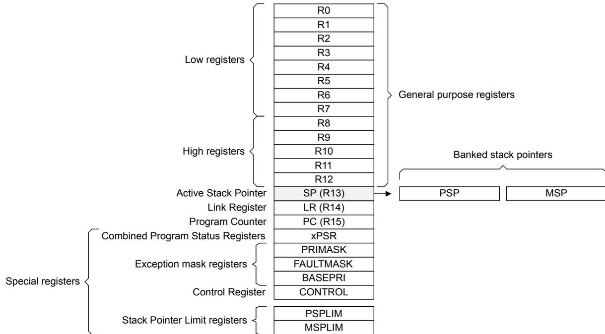
Figure 2-1 Core registers without the Security Extension
