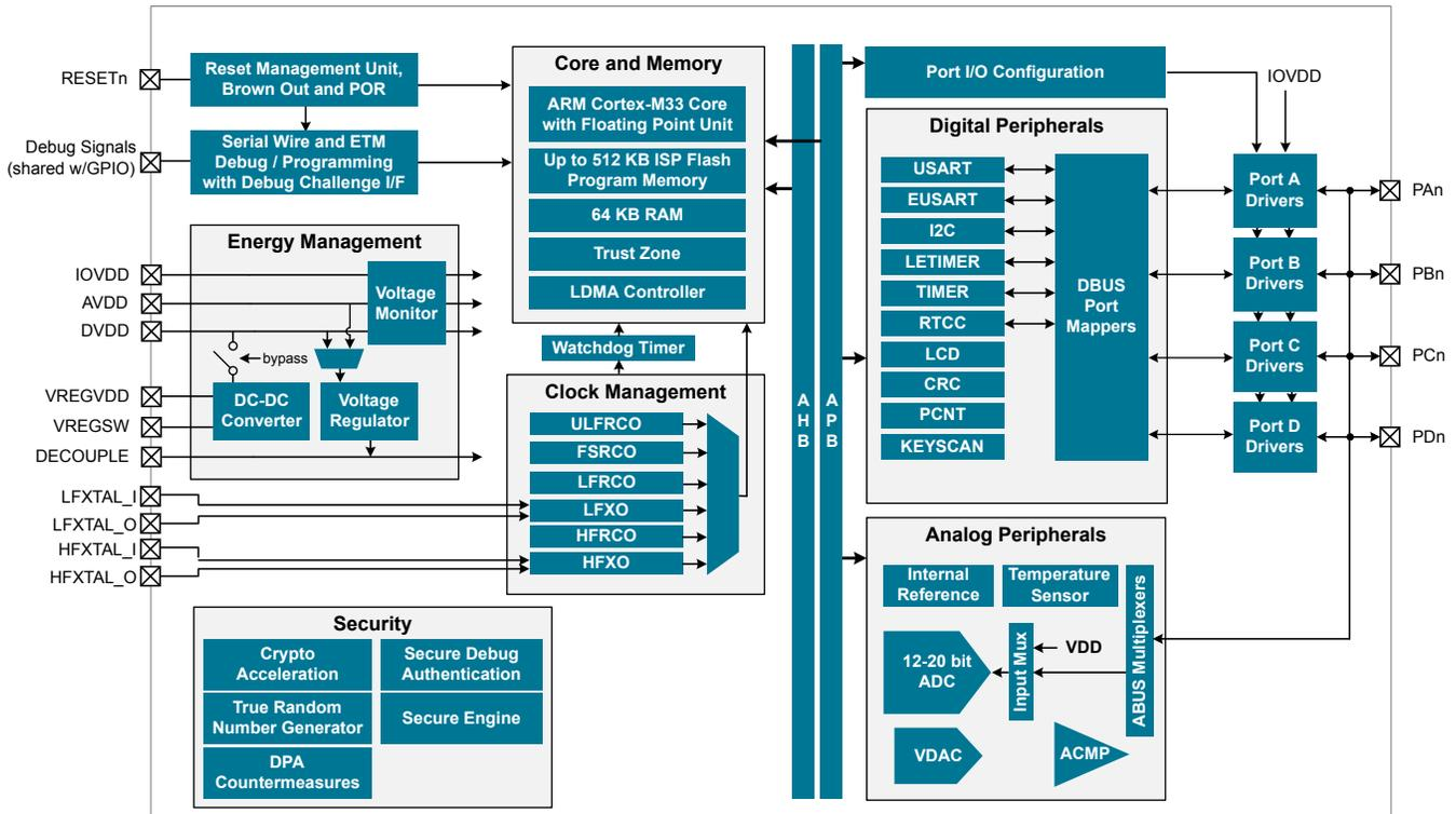
Figure 3.1. Detailed EFM32PG23 Block Diagram
