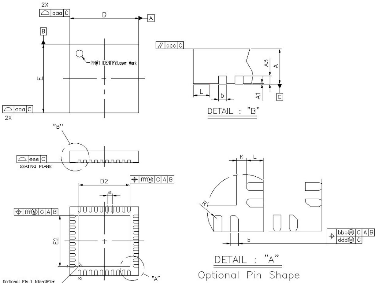
Figure 7.1. QFN40 Package Drawing
