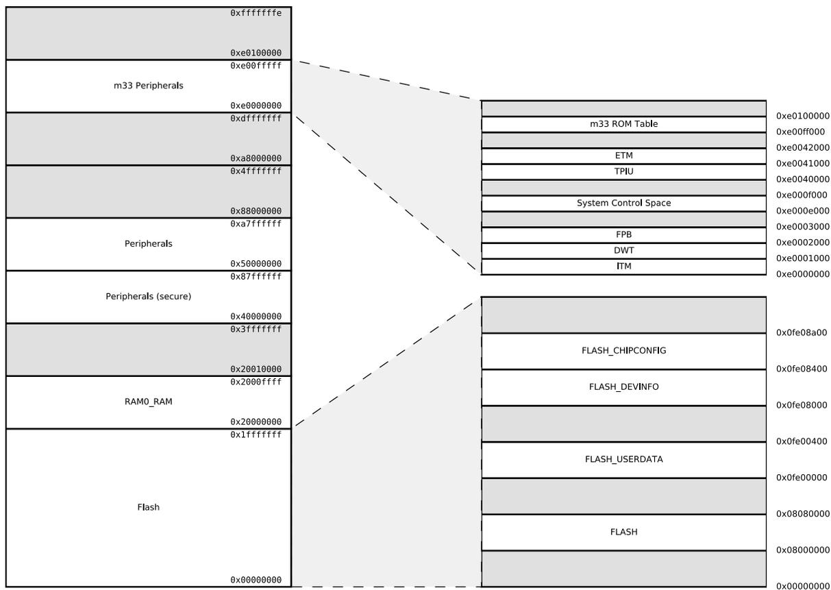
Figure 3.2. EFM32PG23 Memory Map — Core Peripherals and Code Space
