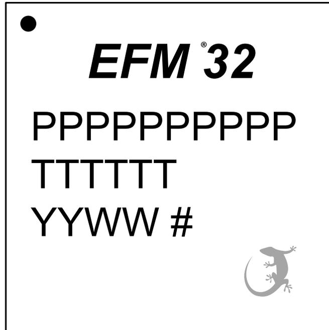
**Figure 7.3. QFN40 Package Marking**
