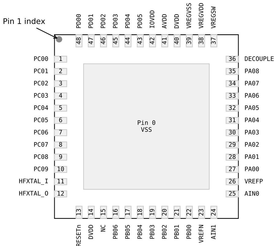
**Figure 6.2. QFN48 with VREF Inputs Device Pinout**
