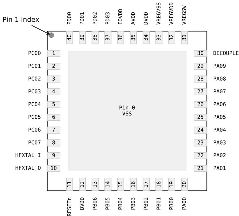
**Figure 6.3. QFN40 Device Pinout**
