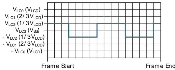
1/3 bias and quadruplex multiplexing - LCD\_SEG0-LCD\_COM2
