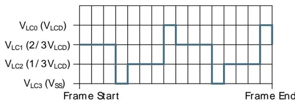
1/3 bias and quadruplex multiplexing - LCD\_SEG0
