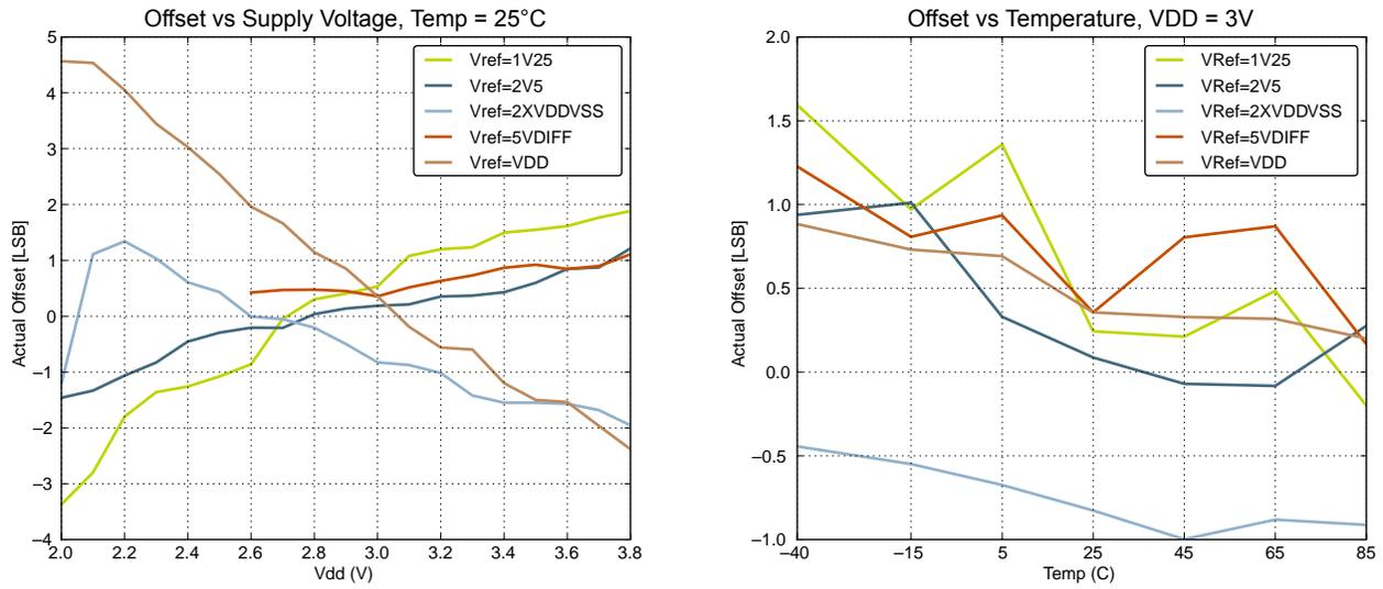
Figure 4.22. ADC Absolute Offset, Common Mode = VDD/2
