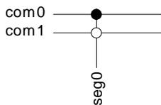
1/3 bias and duplex multiplexing - LCD\_SEG0-LCD\_COM0
