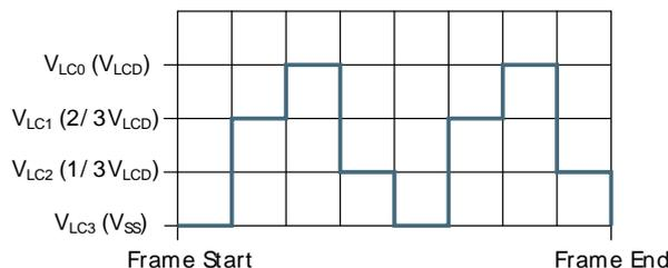
**Figure 29.12. LCD 1/3 Bias and Duplex Multiplexing - LCD\_COM1**
