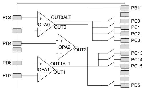
Figure 5.9. Opamp Pinout
