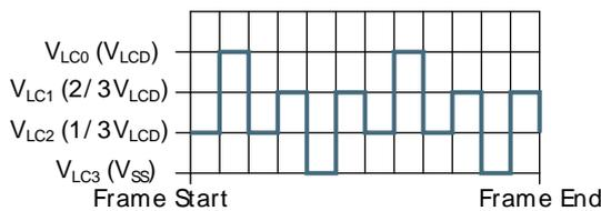
**Figure 29.29. LCD 1/3 Bias and Triplex Multiplexing - LCD\_SEG0 Connection**
