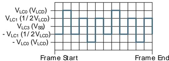
1/2 bias and triplex multiplexing - LCD\_SEG0-LCD\_COM2
