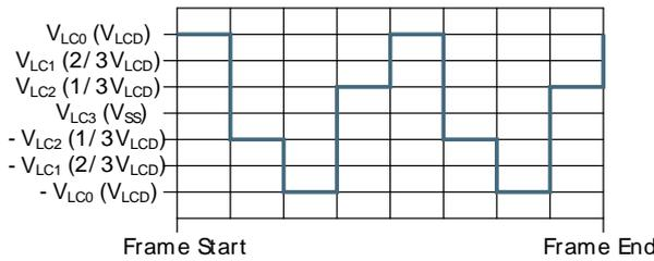
1/3 bias and duplex multiplexing - LCD\_SEG0-LCD\_COM0
