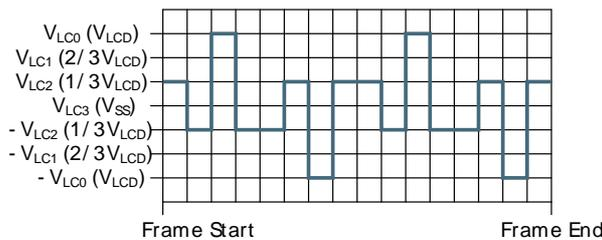
1/3 bias and quadruplex multiplexing - LCD\_SEG0-LCD\_COM2
