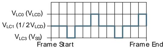
1/2 bias and triplex multiplexing - LCD\_SEG0
