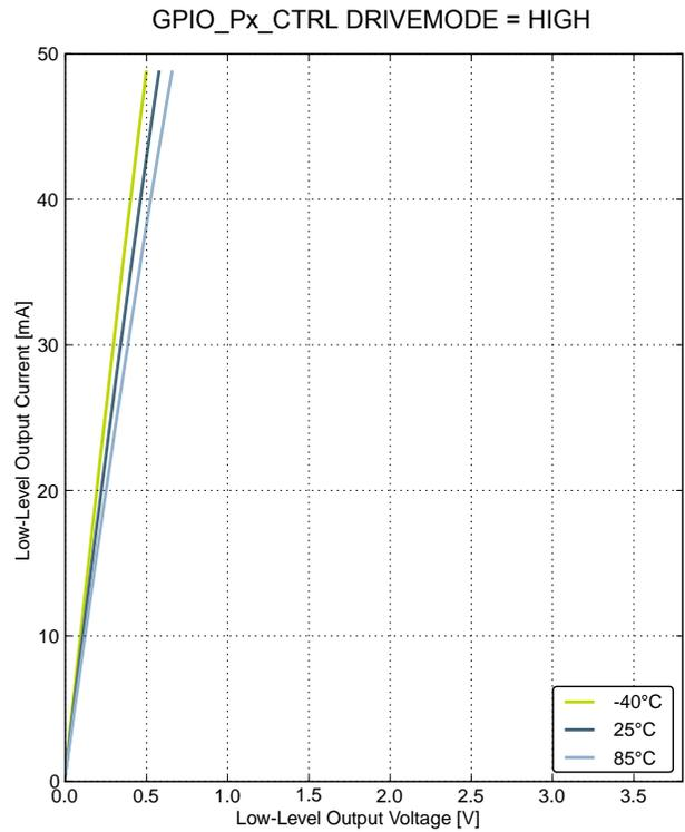
Figure 4.8. Typical Low-Level Output Current, 3.8 V Supply Voltage
