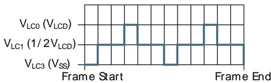
**Figure 29.18. LCD 1/2 Bias and Triplex Multiplexing - LCD\_COM1**
