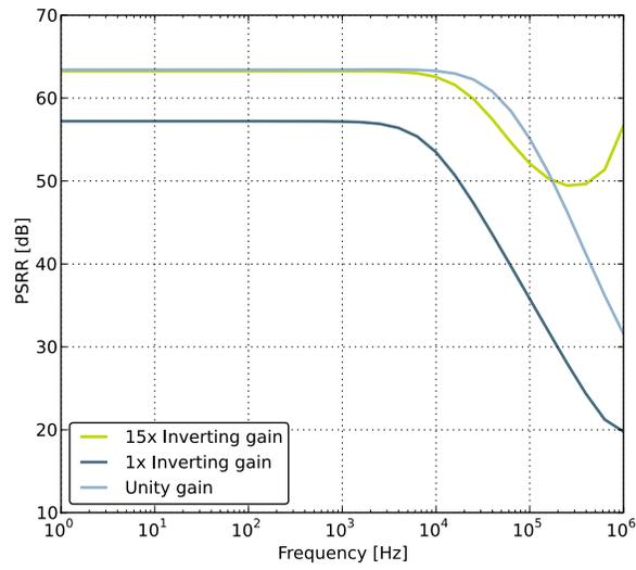
Figure 4.26. OPAMP Negative Power Supply Rejection Ratio
