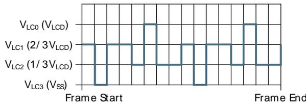
**Figure 29.35. LCD 1/3 Bias and Quadruplex Multiplexing - LCD\_COM2**
