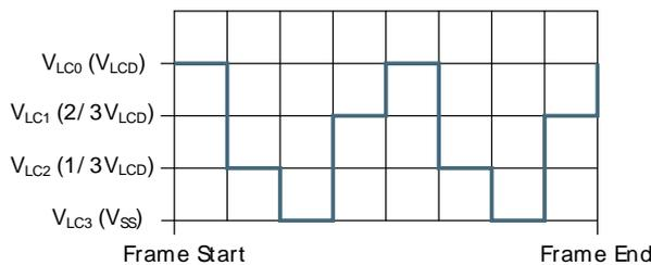
**Figure 29.14. LCD 1/3 Bias and Duplex Multiplexing - LCD\_SEG0 Connection**
