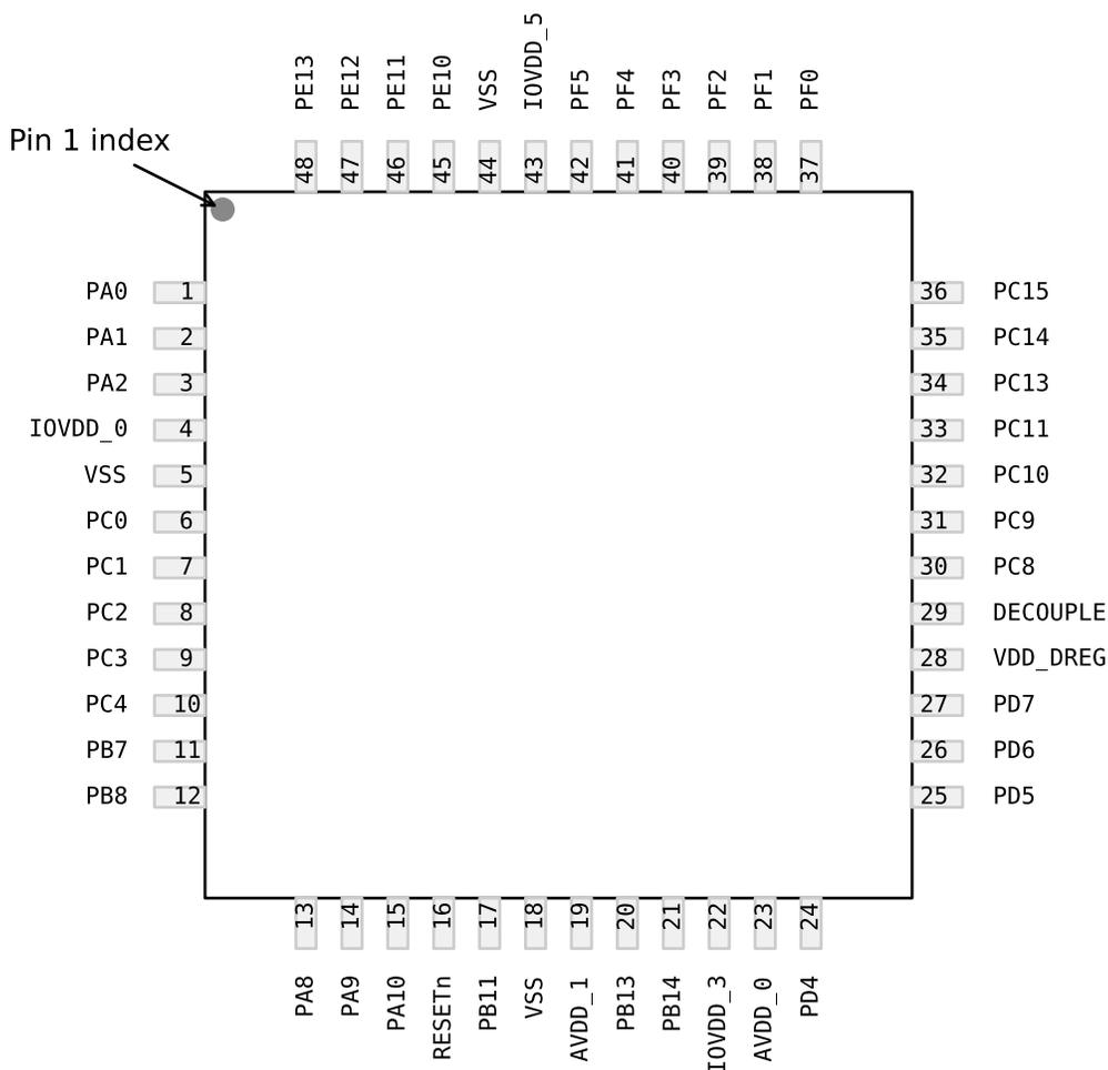
Figure 5.6. EFM32TG222 Pinout (top view, not to scale)
