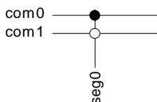
1/2 bias and duplex multiplexing - LCD\_SEG0-LCD\_COM0
