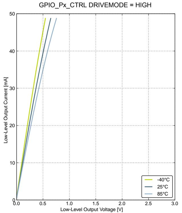
Figure 4.6. Typical Low-Level Output Current, 3 V Supply Voltage
