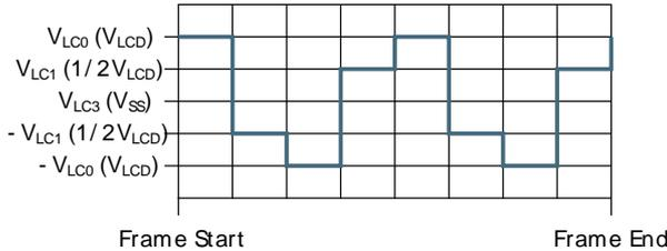
1/2 bias and duplex multiplexing - LCD\_SEG0-LCD\_COM1
