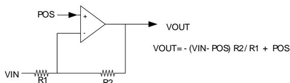
**Table 26.3. Inverting input PGA Configuration**
