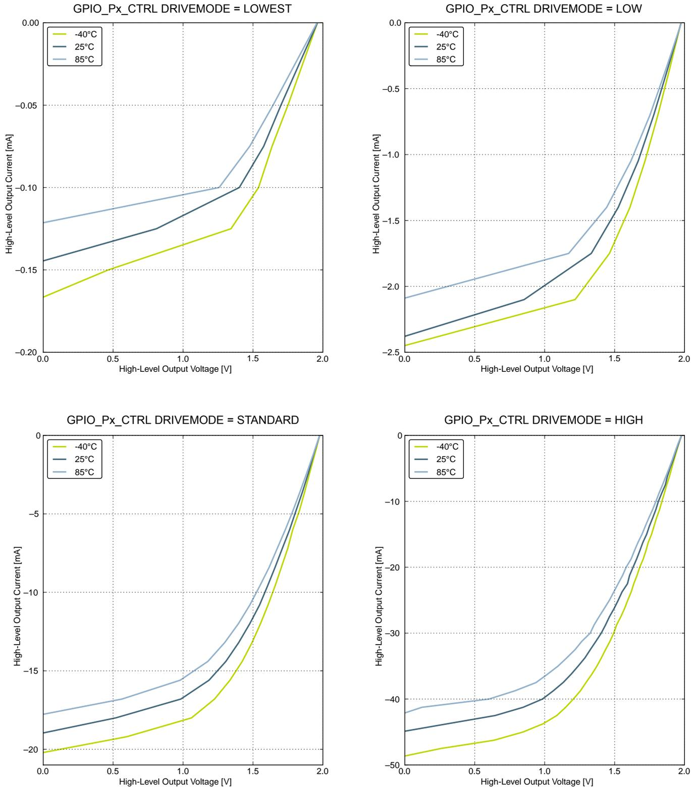
Figure 4.5. Typical High-Level Output Current, 2 V Supply Voltage
