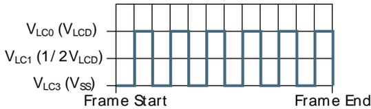
**Figure 29.21. LCD 1/2 Bias and Triplex Multiplexing - LCD\_SEG0 Connection**
