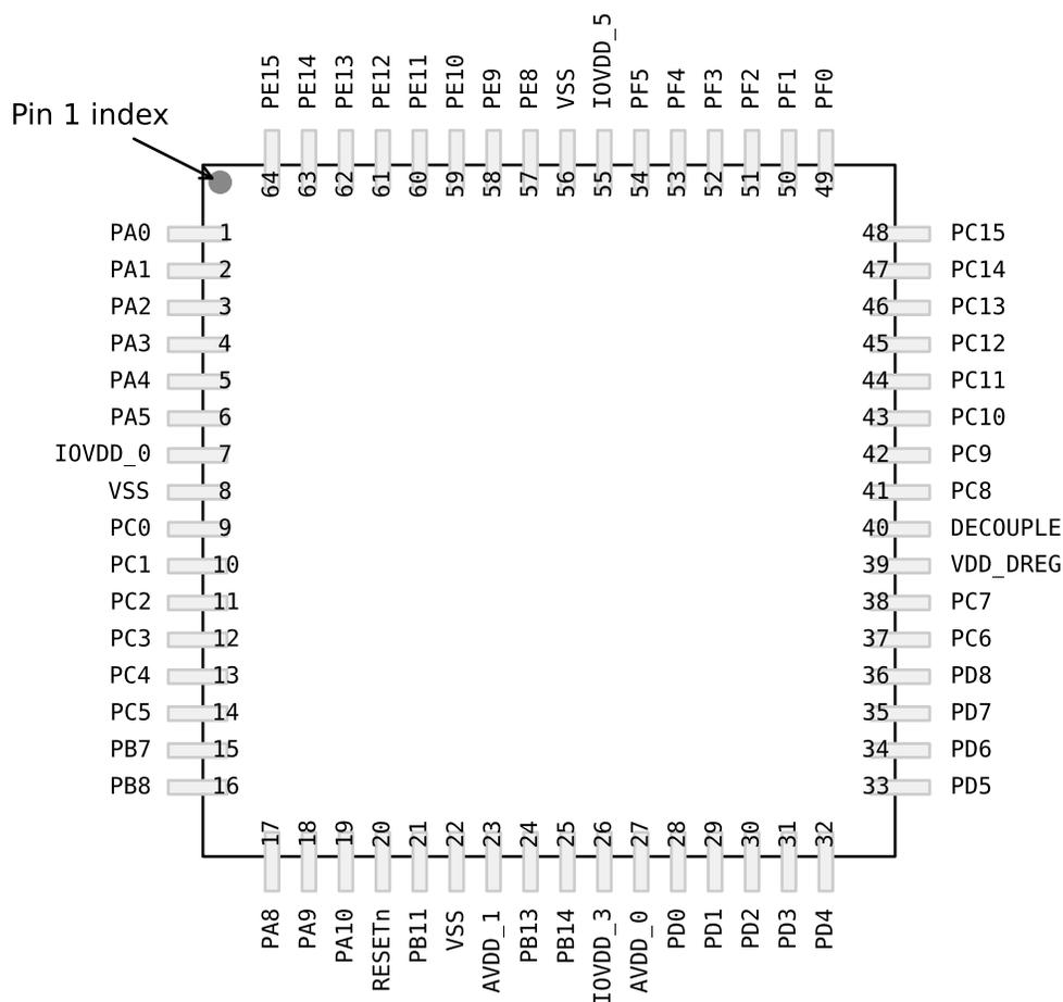
Figure 5.12. EFM32TG232 Pinout (top view, not to scale)
