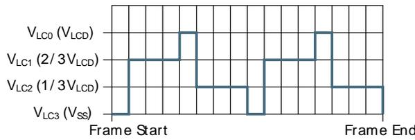
**Figure 29.34. LCD 1/3 Bias and Quadruplex Multiplexing - LCD\_COM1**
