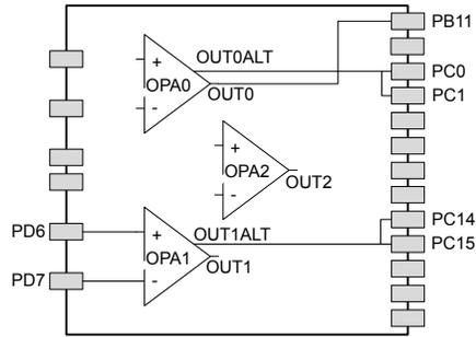
**Figure 5.3. Opamp Pinout**
