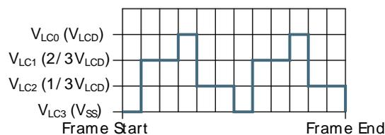
**Figure 29.26. LCD 1/3 Bias and Triplex Multiplexing - LCD\_COM1**
