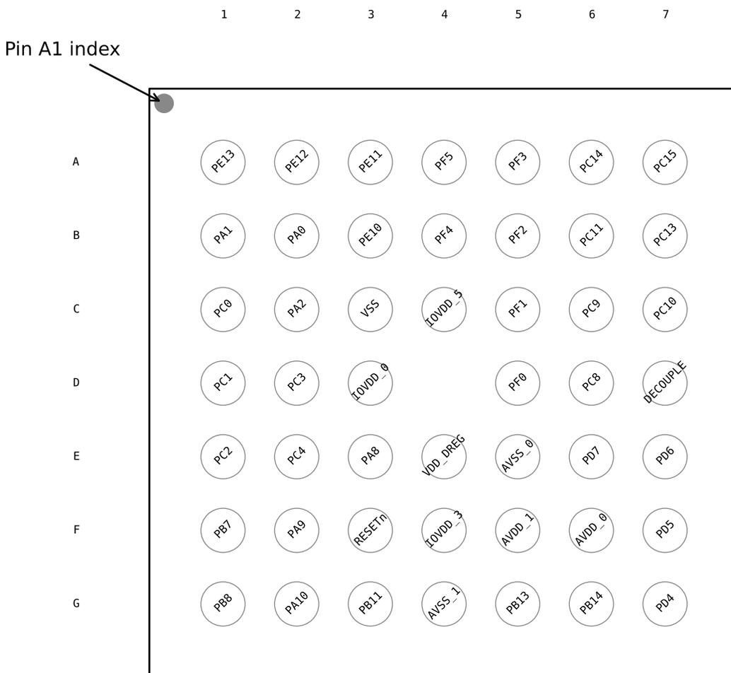
Figure 5.8. EFM32TG225 Pinout (top view, not to scale)
