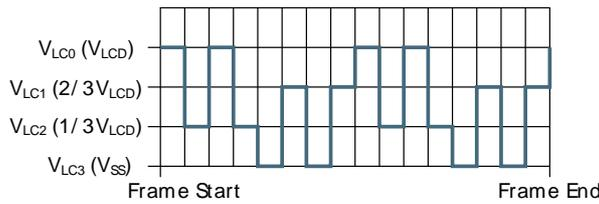
**Figure 29.38. LCD 1/3 Bias and Quadruplex Multiplexing - LCD\_SEG0 Connection**
