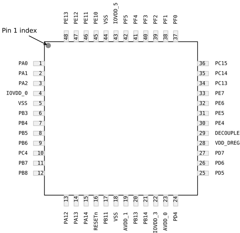
Figure 5.14. EFM32TG822 Pinout (top view, not to scale)
