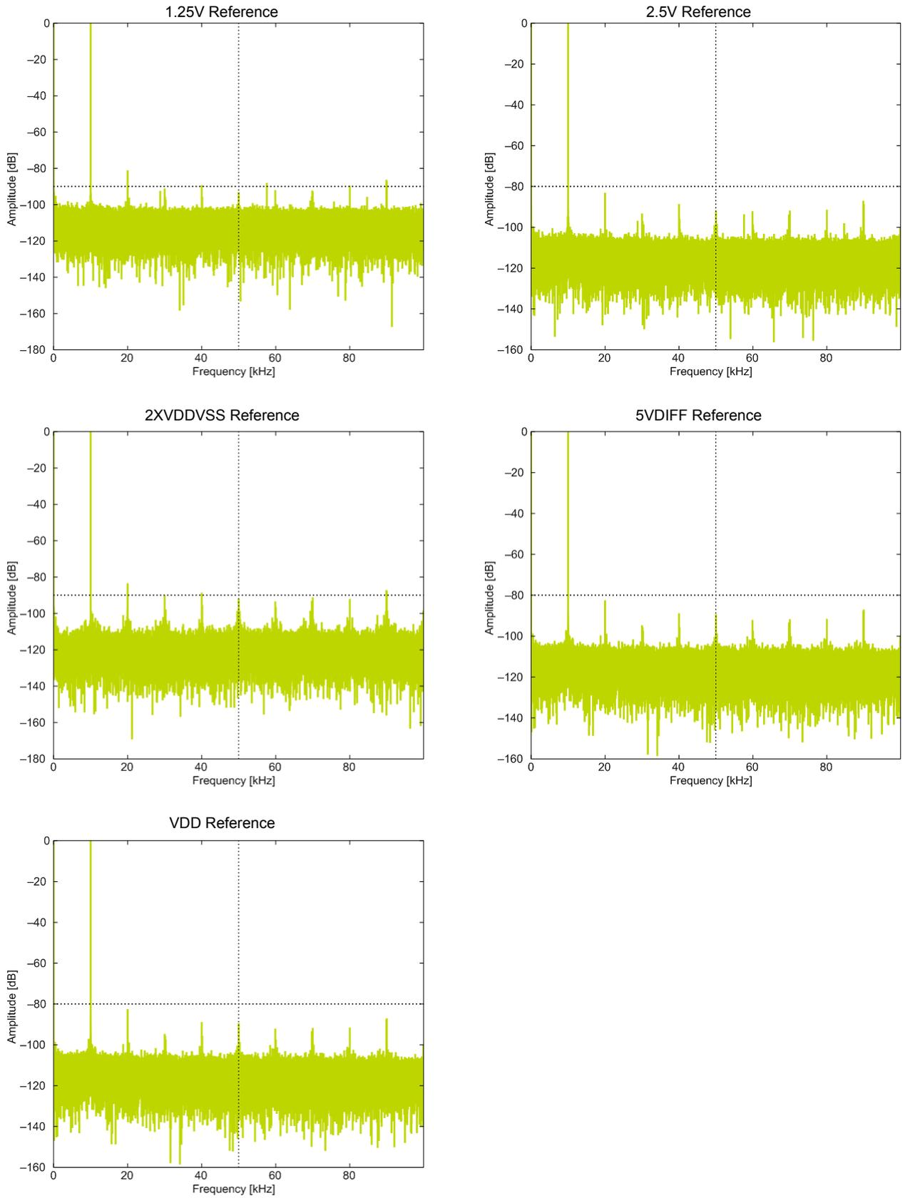
Figure 4.19. ADC Frequency Spectrum, VDD = 3 V, Temp = 25 °C
