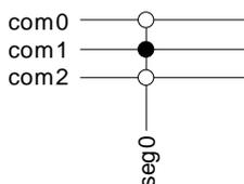
1/3 bias and triplex multiplexing - LCD\_SEG0-LCD\_COM0
