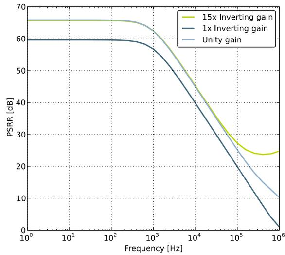
Figure 4.25. OPAMP Positive Power Supply Rejection Ratio
