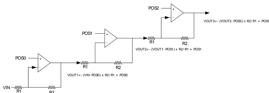
**Table 26.5. Cascaded Inverting PGA Configuration**
