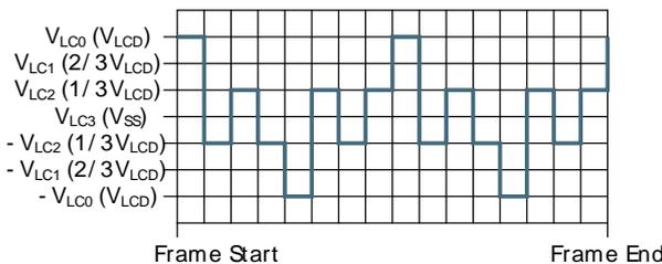
1/3 bias and quadruplex multiplexing - LCD\_SEG0-LCD\_COM1
