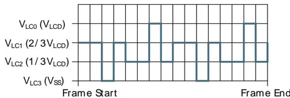
**Figure 29.36. LCD 1/3 Bias and Quadruplex Multiplexing - LCD\_COM3**
