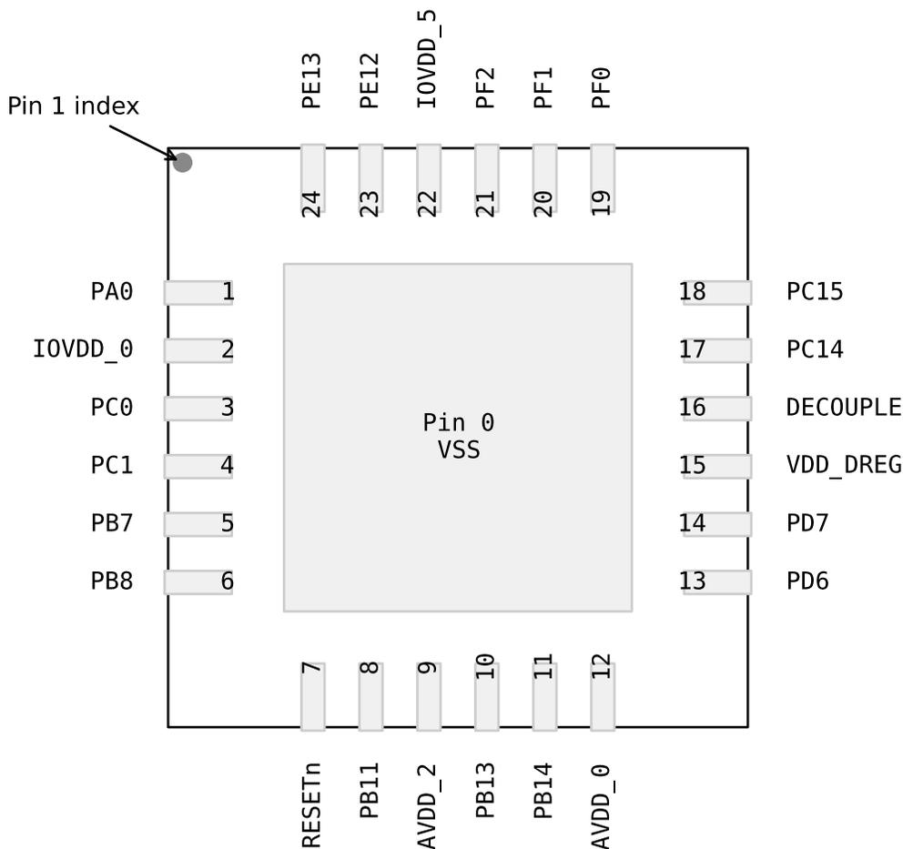
Figure 5.2. EFM32TG110 Pinout (top view, not to scale)
