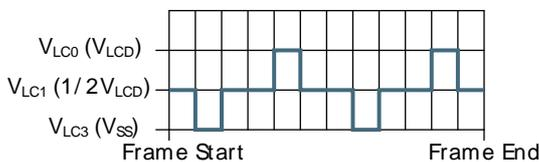
**Figure 29.19. LCD 1/2 Bias and Triplex Multiplexing - LCD\_COM2**
