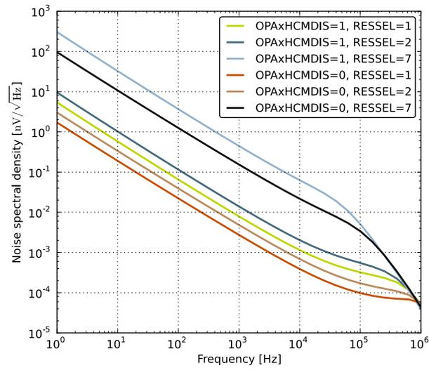
Figure 4.28. OPAMP Voltage Noise Spectral Density (Non-Unity Gain)
