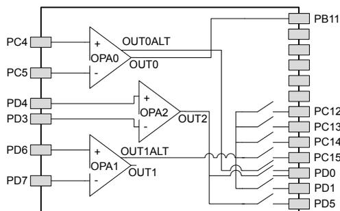
**Figure 5.21. Opamp Pinout**
