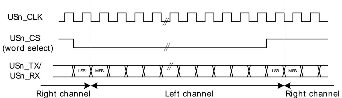
**Figure 15.17. USART Standard I2S waveform (reduced accuracy)**
