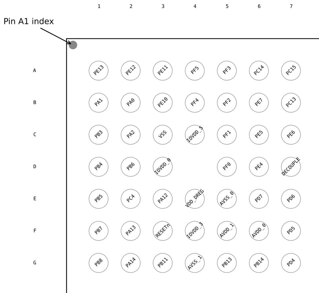
Figure 5.16. EFM32TG825 Pinout (top view, not to scale)
