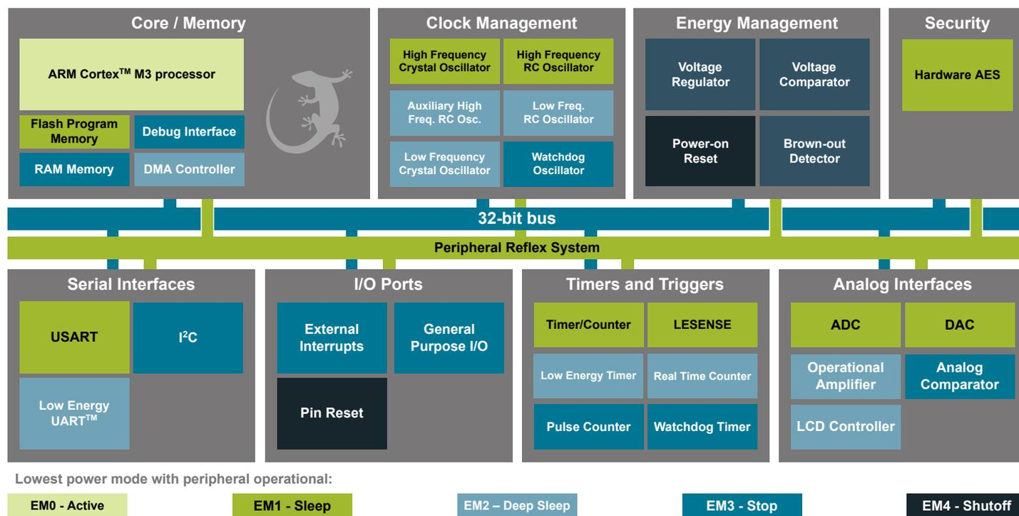
Figure 3.1. Block Diagram
