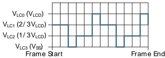
1/3 bias and triplex multiplexing - LCD\_SEG0
