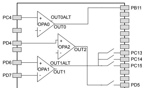
**Figure 5.17. Opamp Pinout**
