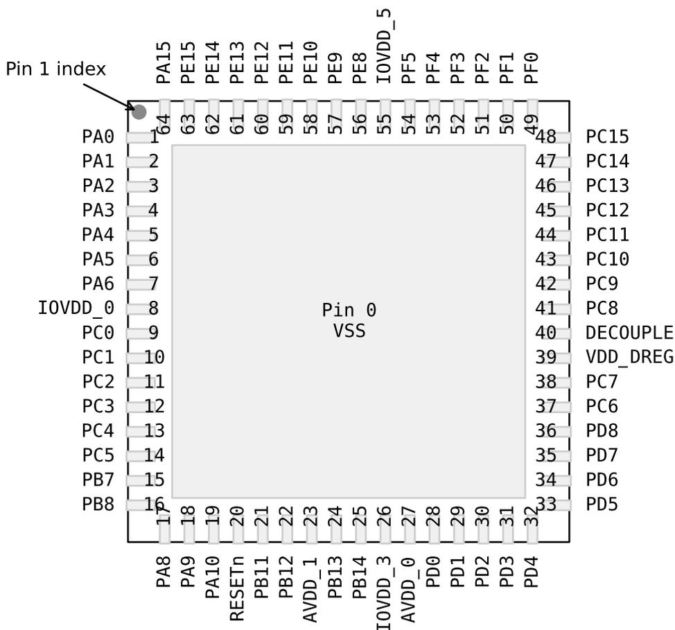
Figure 5.10. EFM32TG230 Pinout (top view, not to scale)
