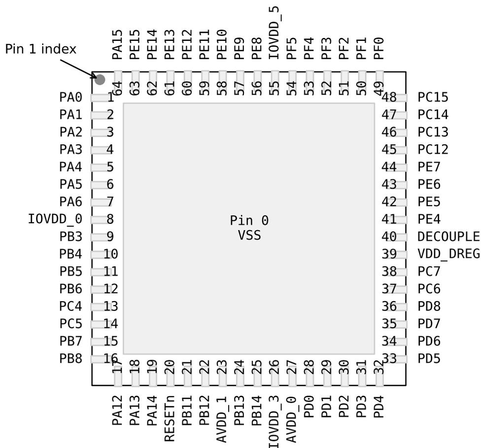
Figure 5.18. EFM32TG840 Pinout (top view, not to scale)
