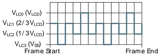
**Figure 29.27. LCD 1/3 Bias and Triplex Multiplexing - LCD\_COM2**
