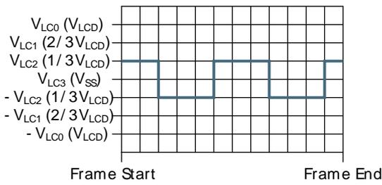
1/3 bias and triplex multiplexing - LCD\_SEG0-LCD\_COM1
