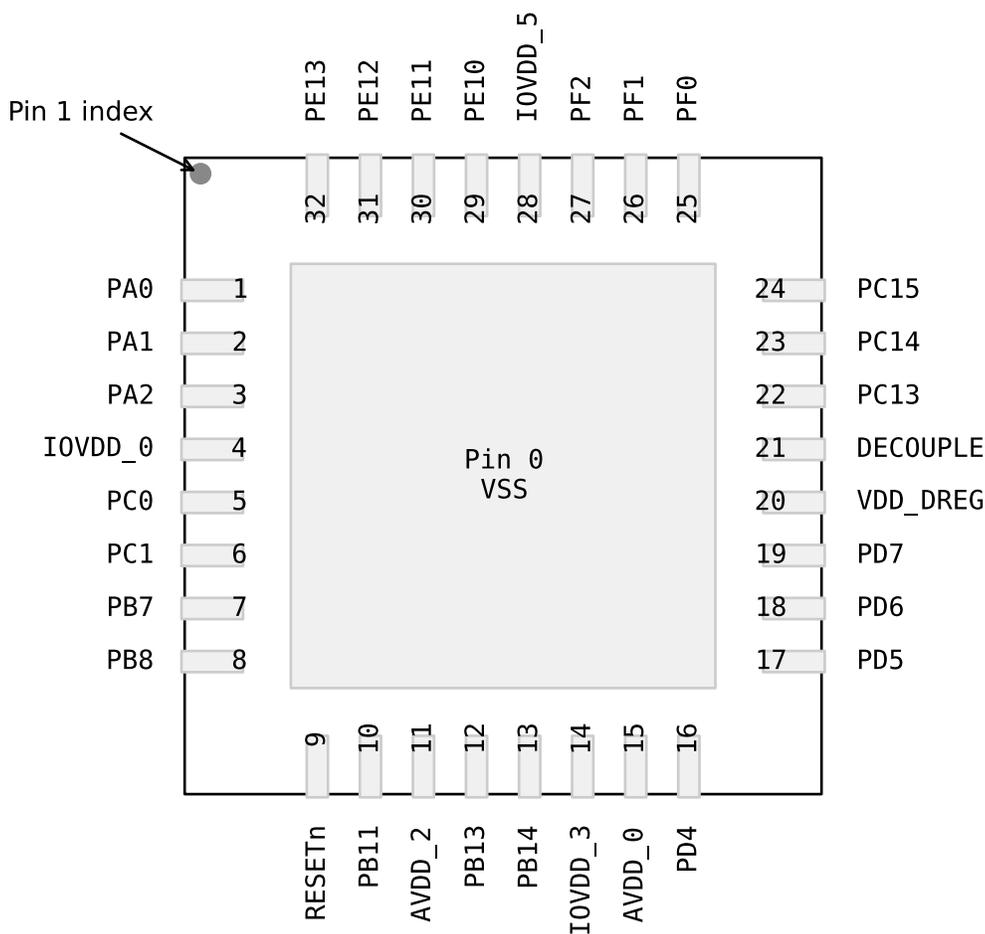
Figure 5.4. EFM32TG210 Pinout (top view, not to scale)
