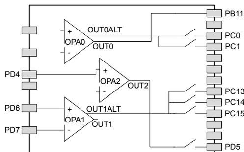
**Figure 5.5. Opamp Pinout**
