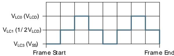
**Figure 29.6. LCD 1/2 Bias and Duplex Multiplexing - LCD\_COM1**
