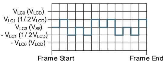
1/2 bias and triplex multiplexing - LCD\_SEG0-LCD\_COM1
