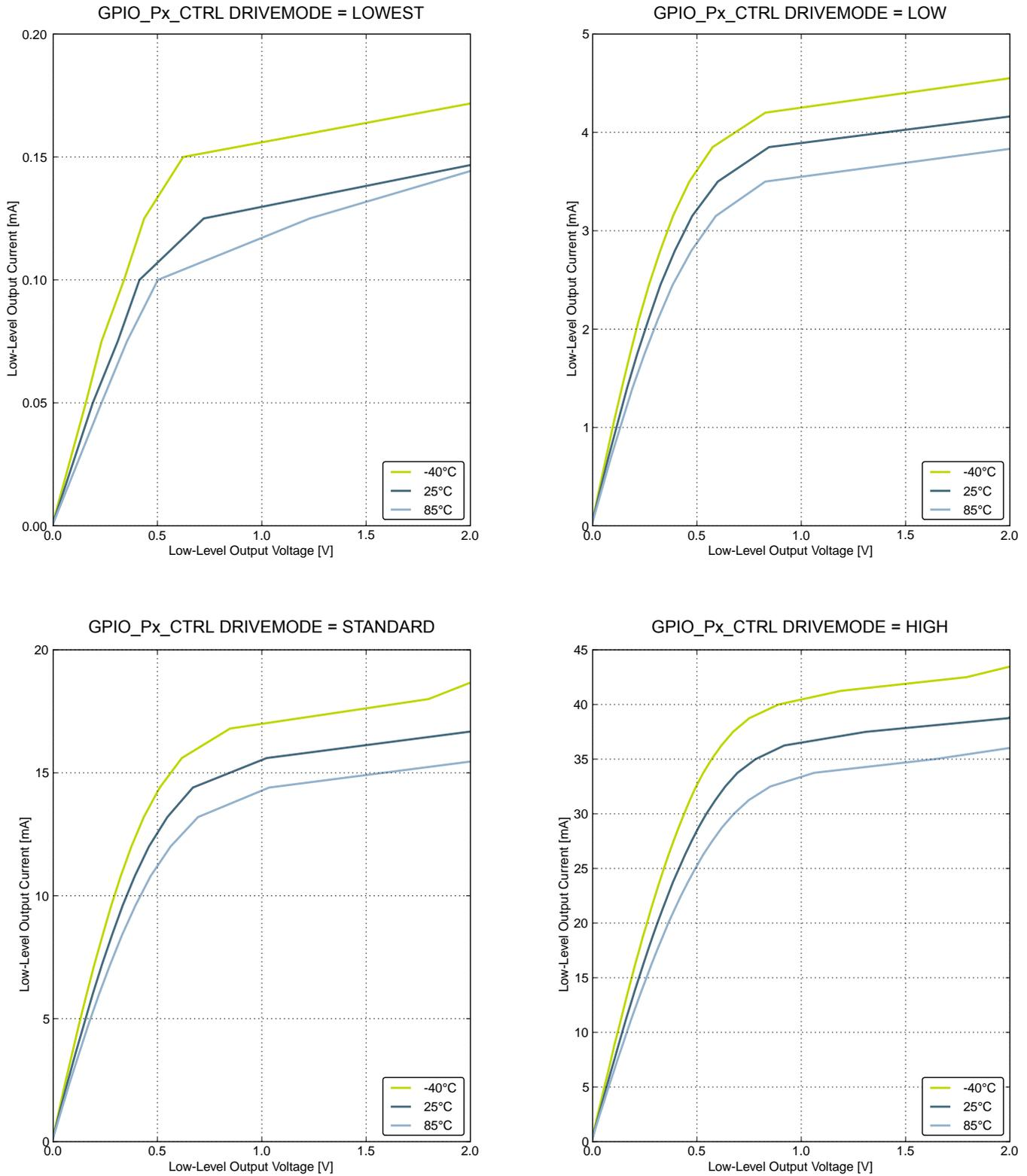
Figure 4.4. Typical Low-Level Output Current, 2V Supply Voltage
