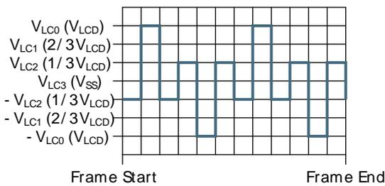
1/3 bias and triplex multiplexing - LCD\_SEG0-LCD\_COM2
