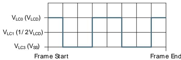
**Figure 29.8. LCD 1/2 Bias and Duplex Multiplexing - LCD\_SEG0 Connection**
