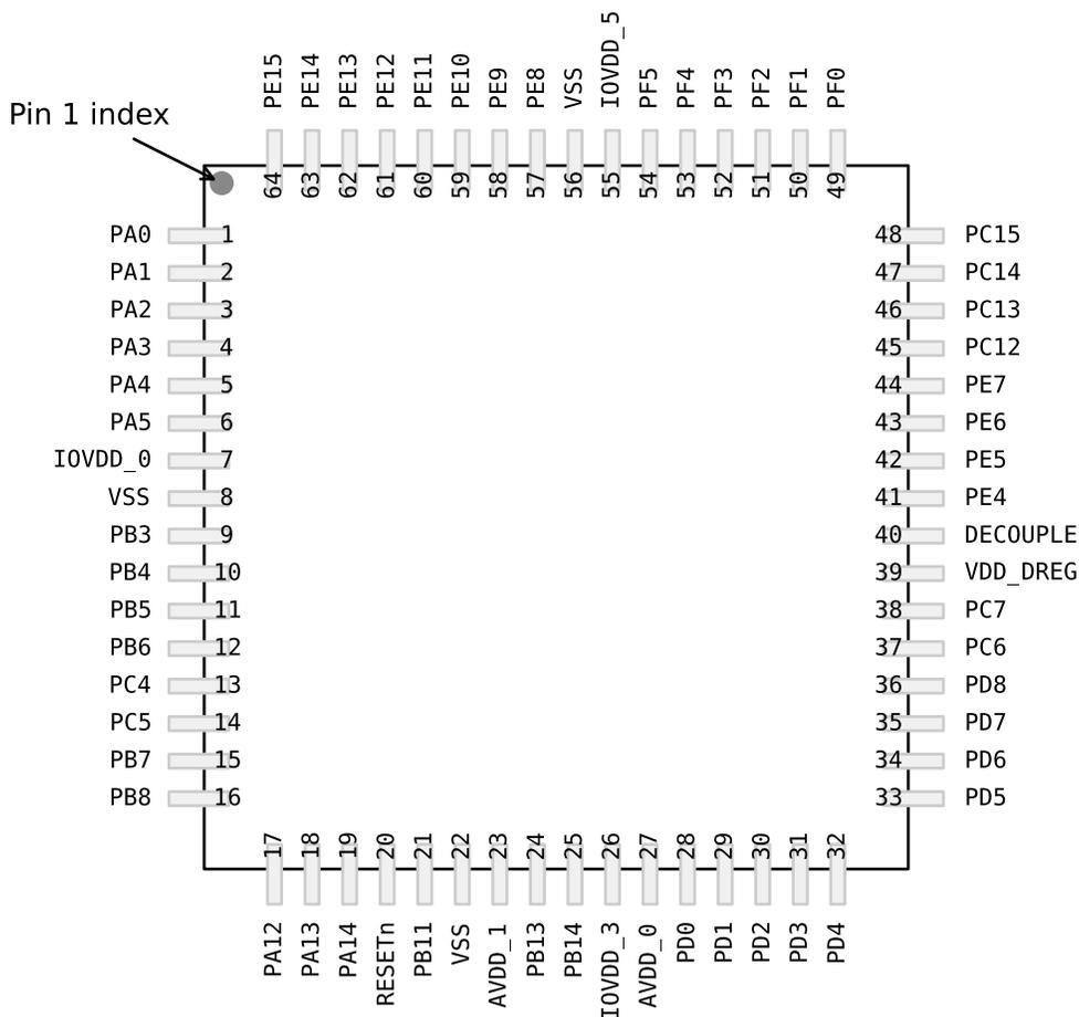
Figure 5.20. EFM32TG842 Pinout (top view, not to scale)
