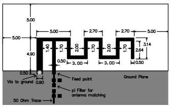
Figure 8 - Trace Antenna (dimensions in mm)
