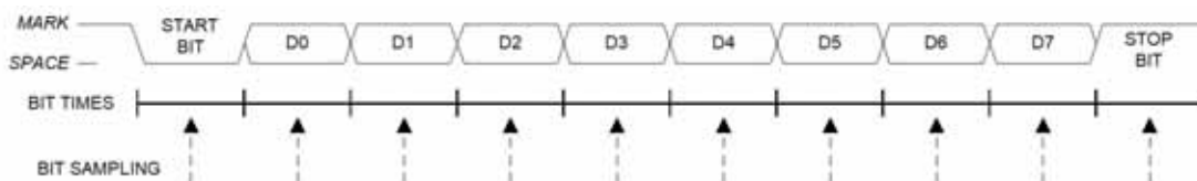
Figure 22.4. UART0 Mode 1 Timing Diagram
