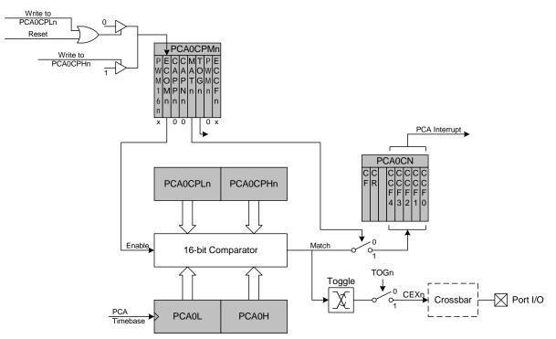
Figure 20.6. PCA High Speed Output Mode Diagram
