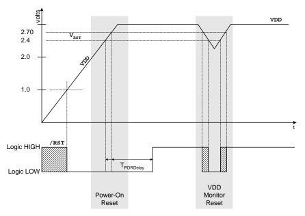
Figure 10.2. Power-On and VDD Monitor Reset Timing
