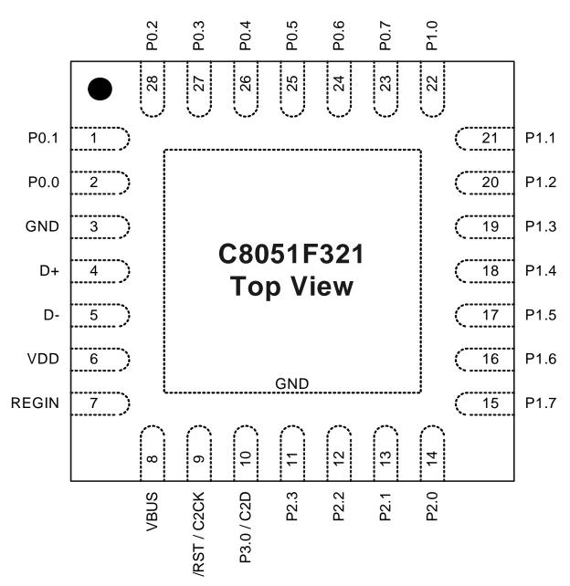
Figure 4.4. QFN-28 Pinout Diagram (Top View)
