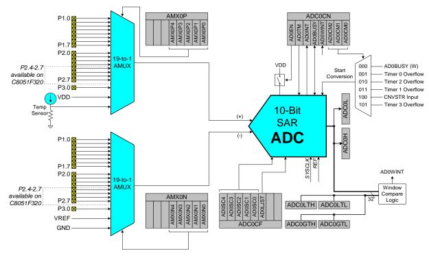
Figure 5.1. ADC0 Functional Block Diagram
