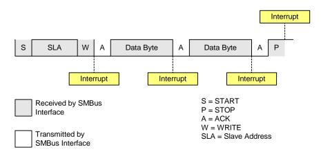
Figure 16.7. Typical Slave Receiver Sequence
