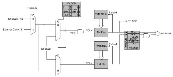
Figure 19.9. Timer 3 8-Bit Mode Block Diagram
