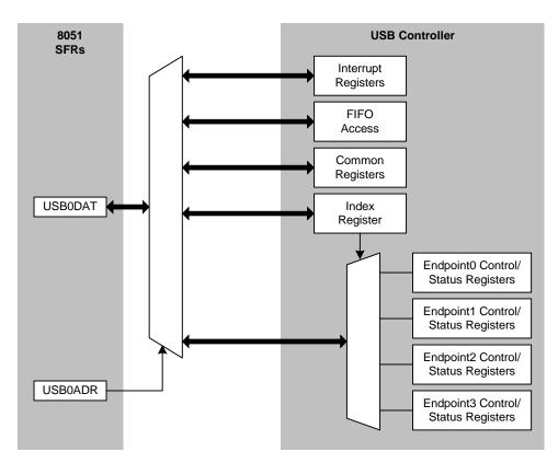
Figure 15.2. USB0 Register Access Scheme
