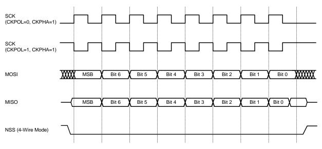
Figure 18.7. Slave Mode Data/Clock Timing (CKPHA = 1)
