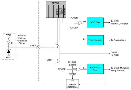
Figure 6.1. Voltage Reference Functional Block Diagram
