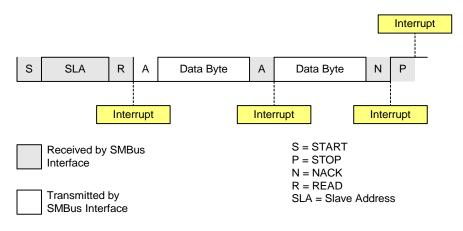
Figure 16.8. Typical Slave Transmitter Sequence
