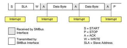
Figure 16.5. Typical Master Transmitter Sequence
