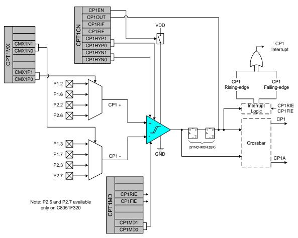
Figure 7.2. Comparator1 Functional Block Diagram
