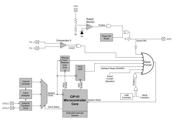
Figure 1.3. On-Chip Clock and Reset
