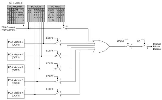
Figure 20.3. PCA Interrupt Block Diagram
