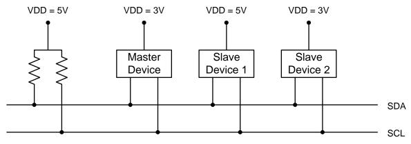
Figure 16.2. Typical SMBus Configuration
