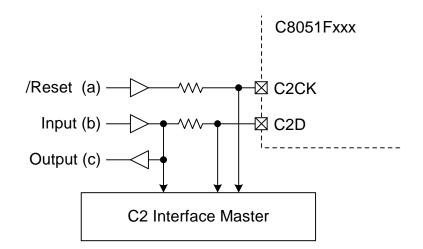
Figure 21.1. Typical C2 Pin Sharing
