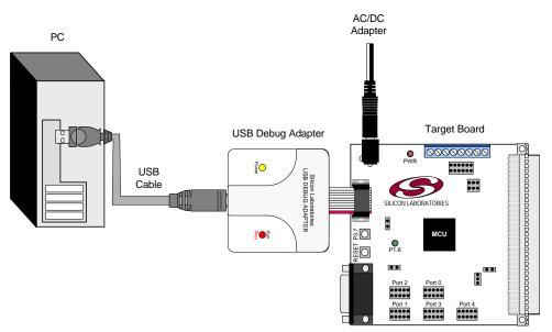
Figure 1.6. Development/In-System Debug Diagram
