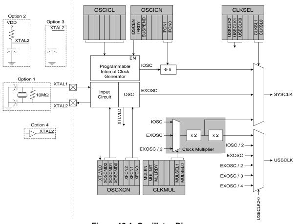
Figure 13.1. Oscillator Diagram
