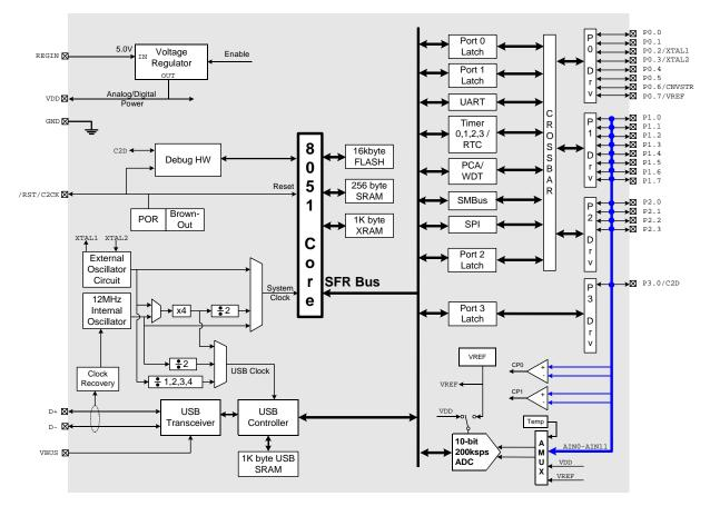
Figure 1.2. C8051F321 Block Diagram
