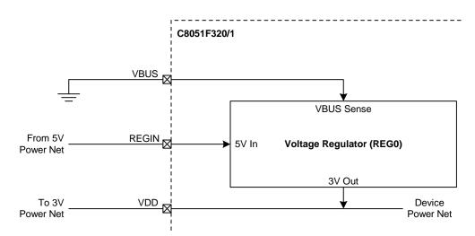
Figure 8.5. REG0 Configuration: No USB Connection
