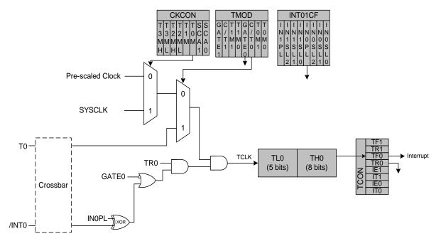
Figure 19.1. T0 Mode 0 Block Diagram
