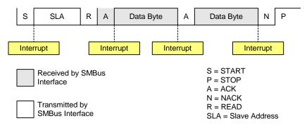
Figure 16.6. Typical Master Receiver Sequence
