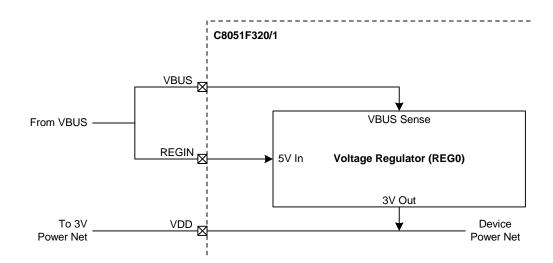
Figure 8.2. REG0 Configuration: USB Bus-Powered
