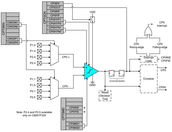
Figure 7.1. Comparator0 Functional Block Diagram
