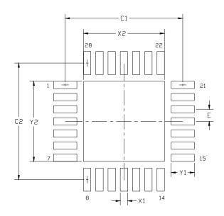
Figure 4.6. QFN-28 Recommended PCB Land Pattern
