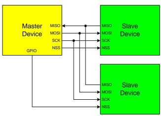
Figure 18.4. 4-Wire Single Master Mode and 4-Wire Slave Mode Connection Diagram
