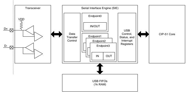
Figure 15.1. USB0 Block Diagram
