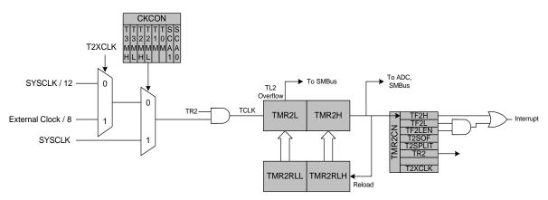
Figure 19.4. Timer 2 16-Bit Mode Block Diagram
