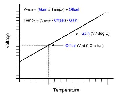
Figure 5.2. Temperature Sensor Transfer Function
