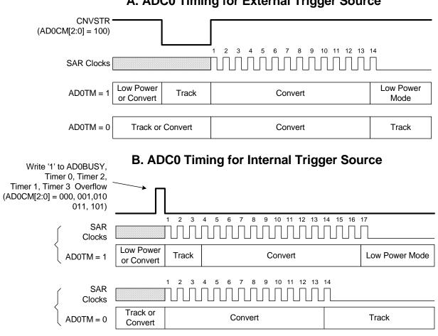
A. ADC0 Timing for External Trigger Source
