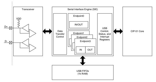
Figure 1.5. USB Controller Block Diagram
