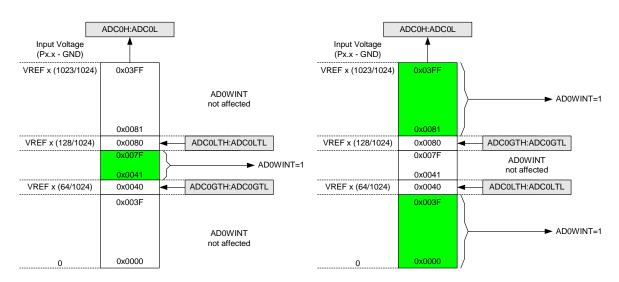
Figure 5.6. ADC Window Compare Example: Right-Justified Single-Ended Data
