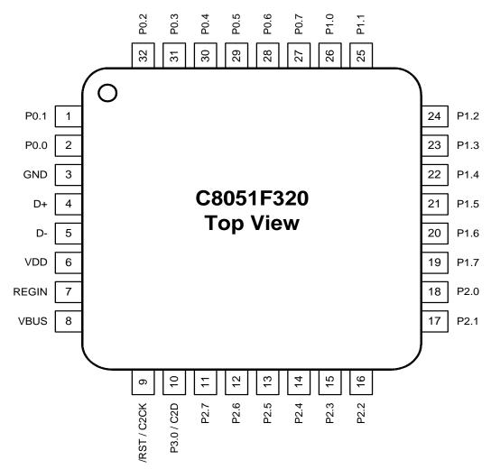
Figure 4.1. LQFP-32 Pinout Diagram (Top View)
