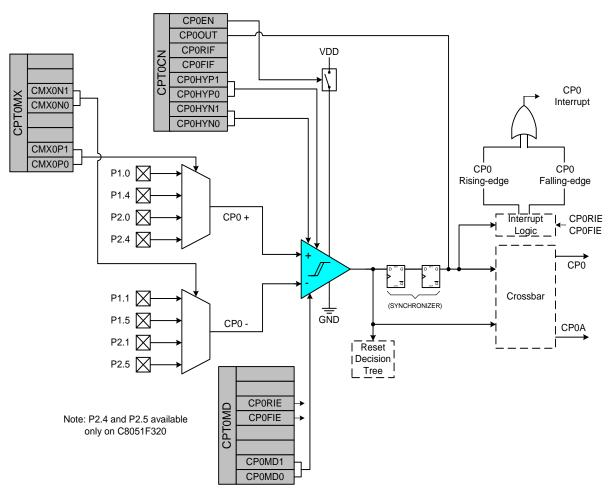
Figure 1.11. Comparator0 Block Diagram
