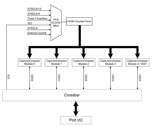
Figure 1.9. PCA Block Diagram
