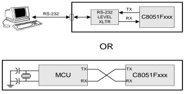
Figure 17.3. UART Interconnect Diagram
