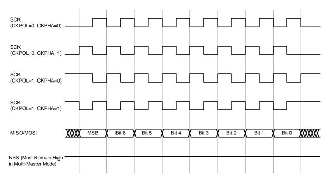
Figure 18.5. Master Mode Data/Clock Timing
