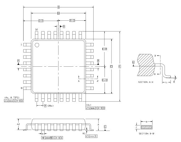
Figure 4.2. LQFP-32 Package Drawing
