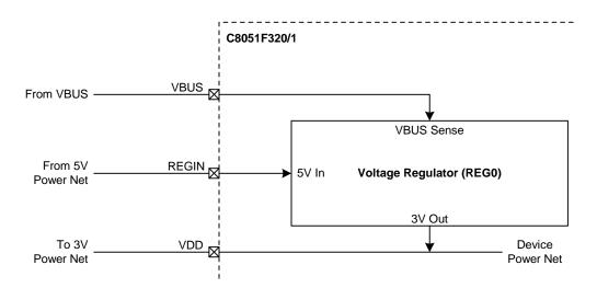
Figure 8.3. REG0 Configuration: USB Self-Powered
