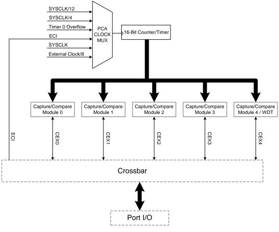
Figure 20.1. PCA Block Diagram
