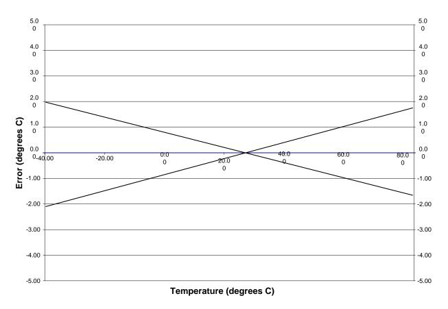
Figure 5.3. Temperature Sensor Error with 1-Point Calibration (VREF = 2.40 V)
