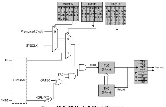
Figure 19.2. T0 Mode 2 Block Diagram
