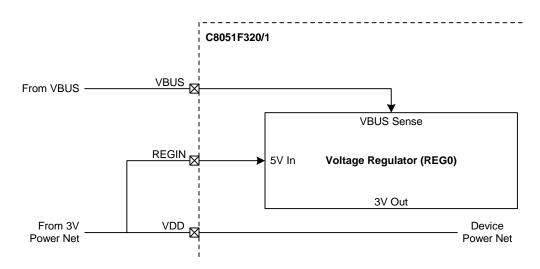
Figure 8.4. REG0 Configuration: USB Self-Powered, Regulator Disabled
