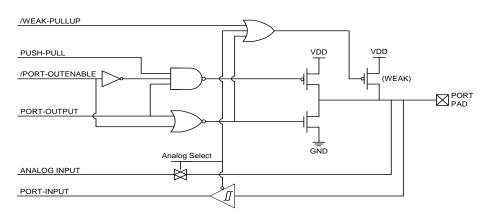
Figure 14.2. Port I/O Cell Block Diagram
