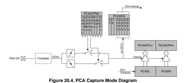
**Note:** The CEXn input signal must remain high or low for at least 2 system clock cycles to be recognized by the hardware.
