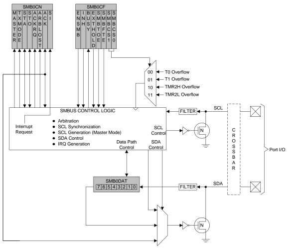
Figure 16.1. SMBus Block Diagram
