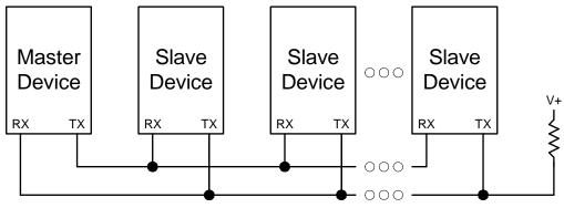
Figure 17.6. UART Multi-Processor Mode Interconnect Diagram
