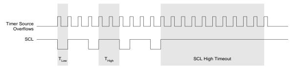
Figure 16.4. Typical SMBus SCL Generation
