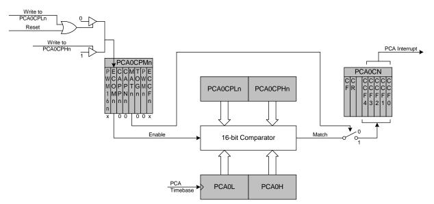
Figure 20.5. PCA Software Timer Mode Diagram
