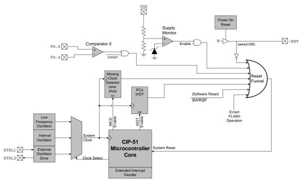
Figure 1.8. On-Chip Clock and Reset
