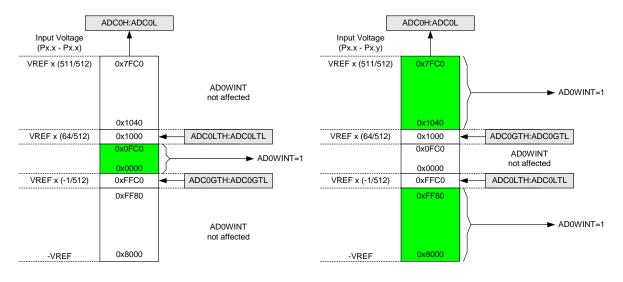
Figure 5.8. ADC Window Compare Example: Left-Justified Differential Data
