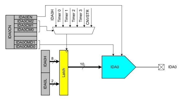
Figure 6.1. IDA0 Functional Block Diagram
