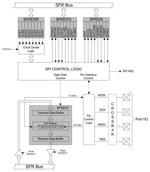
Figure 17.1. SPI Block Diagram
