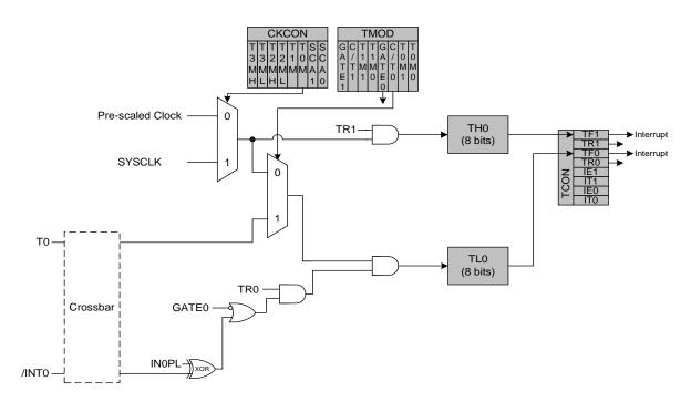
Figure 18.3. T0 Mode 3 Block Diagram
