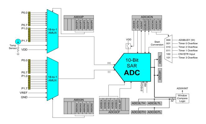
Figure 5.1. ADC0 Functional Block Diagram
