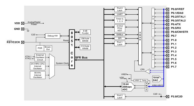
Figure 1.1. C8051F330 Block Diagram
