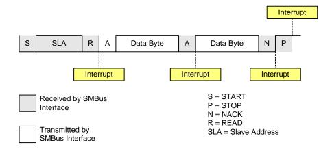
Figure 15.8. Typical Slave Transmitter Sequence
