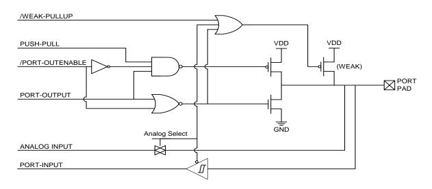
Figure 14.2. Port I/O Cell Block Diagram
