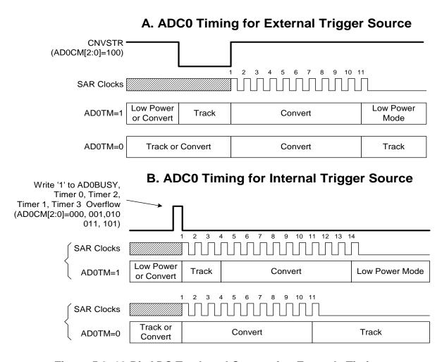
Figure 5.3. 10-Bit ADC Track and Conversion Example Timing
