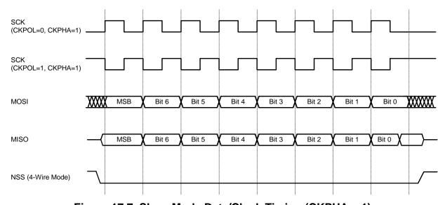
Figure 17.7. Slave Mode Data/Clock Timing (CKPHA = 1)
