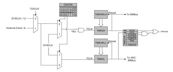
Figure 18.5. Timer 2 8-Bit Mode Block Diagram
