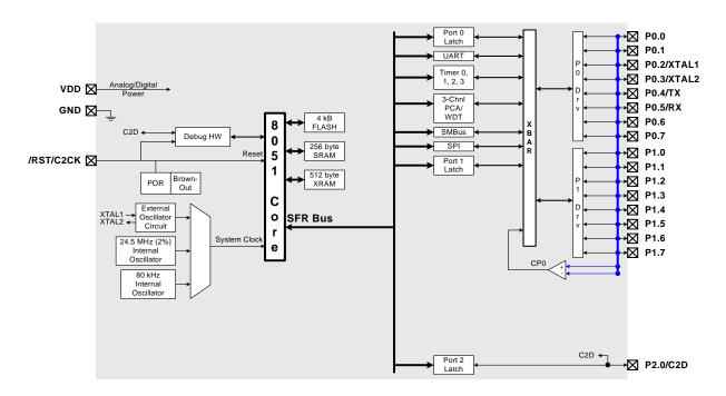
Figure 1.4. C8051F333 Block Diagram
