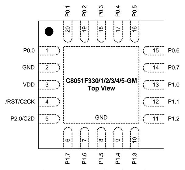
Figure 4.1. QFN-20 Pinout Diagram (Top View)
