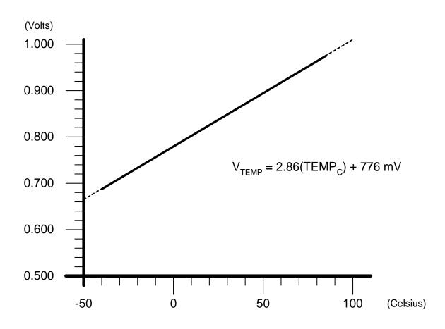
Figure 5.2. Typical Temperature Sensor Transfer Function
