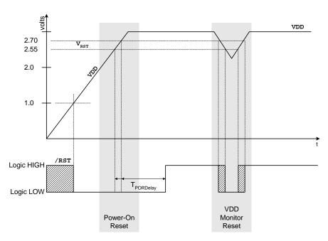
Figure 10.2. Power-On and V<sub>DD</sub> Monitor Reset Timing
