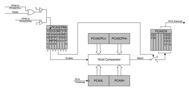
Figure 19.5. PCA Software Timer Mode Diagram
