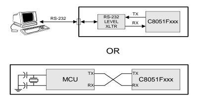
Figure 16.3. UART Interconnect Diagram
