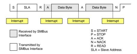
Figure 15.6. Typical Master Receiver Sequence
