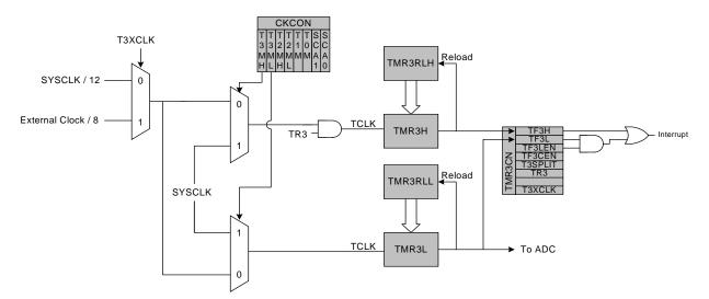
Figure 18.7. Timer 3 8-Bit Mode Block Diagram
