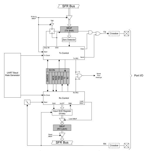
Figure 16.1. UARTO Block Diagram
