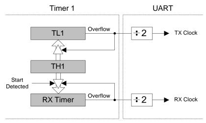
Figure 16.2. UARTO Baud Rate Logic
