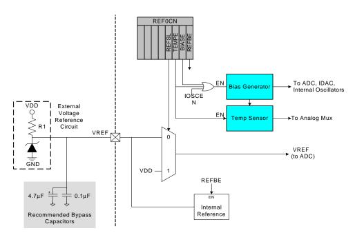
Figure 7.1. Voltage Reference Functional Block Diagram
