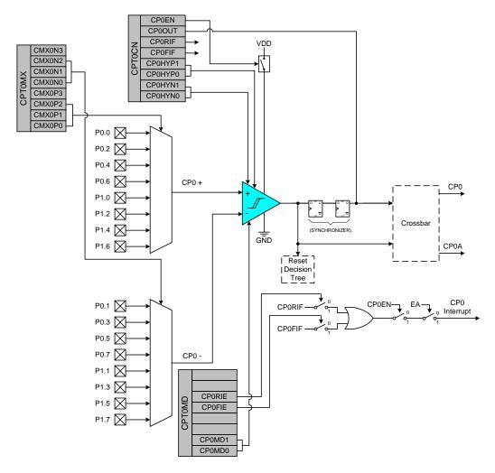
Figure 1.15. Comparator Block Diagram
