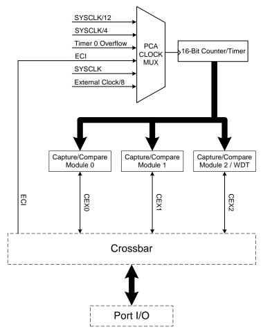
Figure 19.1. PCA Block Diagram
