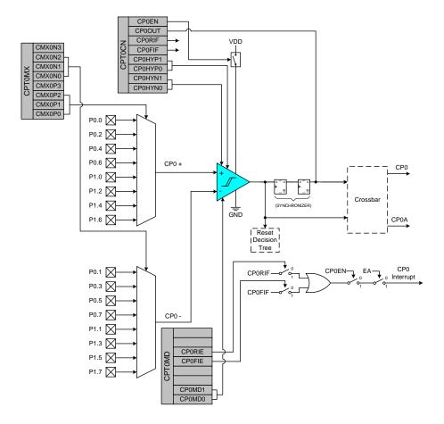
Figure 8.1. Comparator Functional Block Diagram
