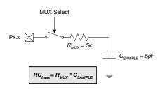
Figure 5.4. ADC0 Equivalent Input Circuits
