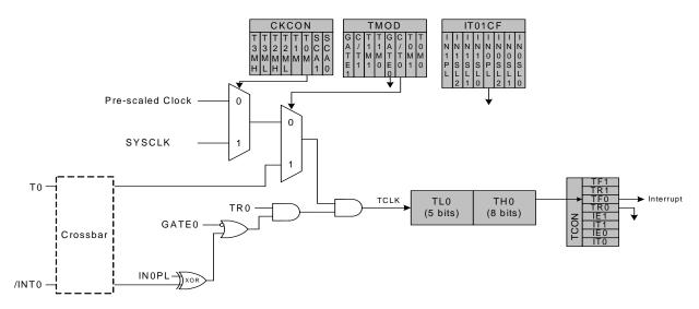
Figure 18.1. T0 Mode 0 Block Diagram
