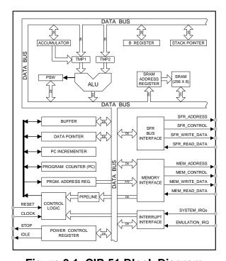
Figure 9.1. CIP-51 Block Diagram
