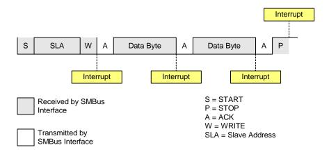
Figure 15.7. Typical Slave Receiver Sequence
