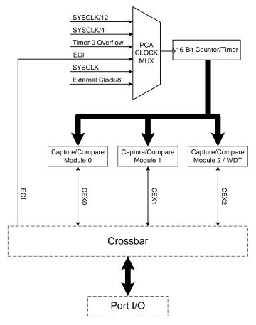
Figure 1.13. PCA Block Diagram
