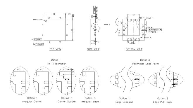
Figure 4.2. QFN-20 Package Drawing
