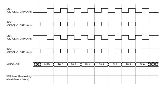
Figure 17.5. Master Mode Data/Clock Timing
