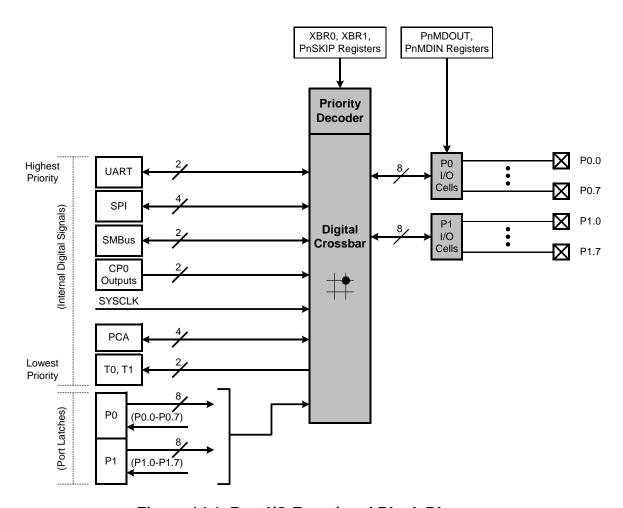
Figure 14.1. Port I/O Functional Block Diagram
