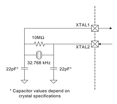
Figure 13.2. External 32.768 kHz Quartz Crystal Oscillator Connection Diagram
