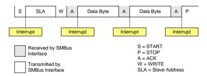
**Figure 15.5. Typical Master Transmitter Sequence**
