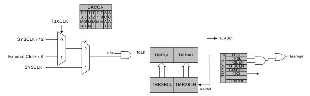
Figure 18.6. Timer 3 16-Bit Mode Block Diagram
