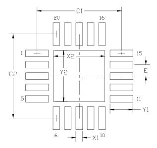
Figure 4.3. QFN-20 Recommended PCB Land Pattern
