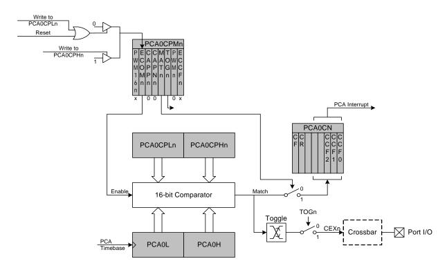
Figure 19.6. PCA High-Speed Output Mode Diagram
