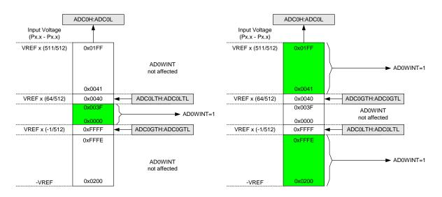
Figure 5.7. ADC Window Compare Example: Right-Justified Differential Data
