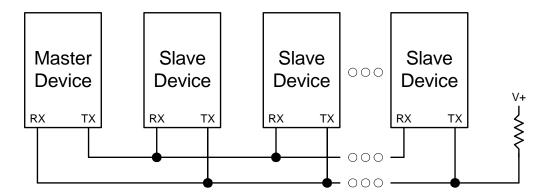
Figure 16.6. UART Multi-Processor Mode Interconnect Diagram
