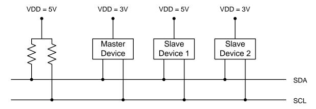
Figure 15.2. Typical SMBus Configuration
