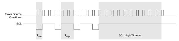
Figure 15.4. Typical SMBus SCL Generation
