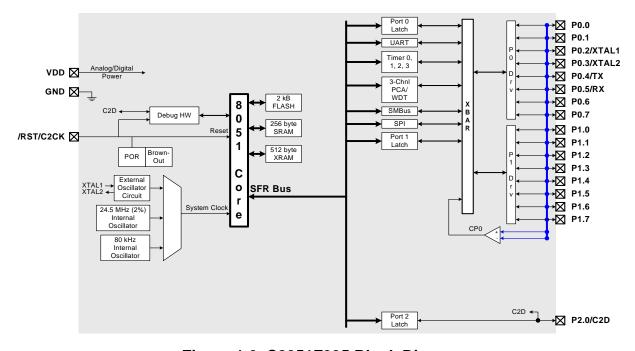
Figure 1.6. C8051F335 Block Diagram
