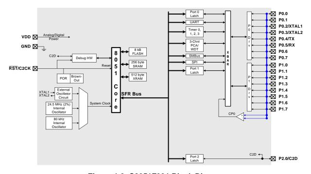
Figure 1.2. C8051F331 Block Diagram
