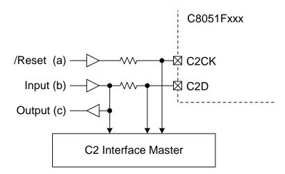
Figure 20.1. Typical C2 Pin Sharing
