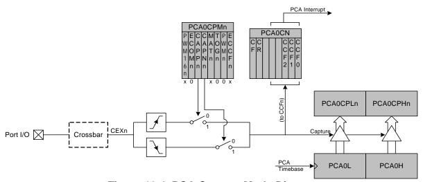
Figure 19.4. PCA Capture Mode Diagram
