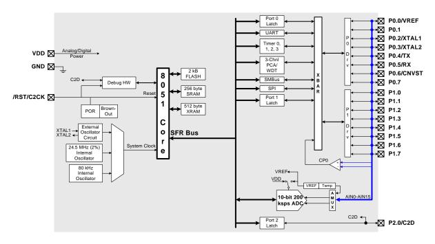
Figure 1.5. C8051F334 Block Diagram
