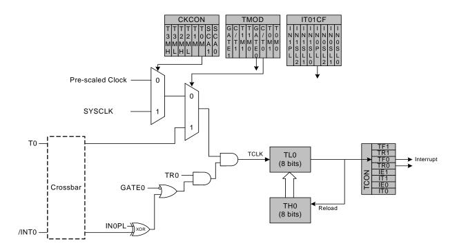
Figure 18.2. T0 Mode 2 Block Diagram
