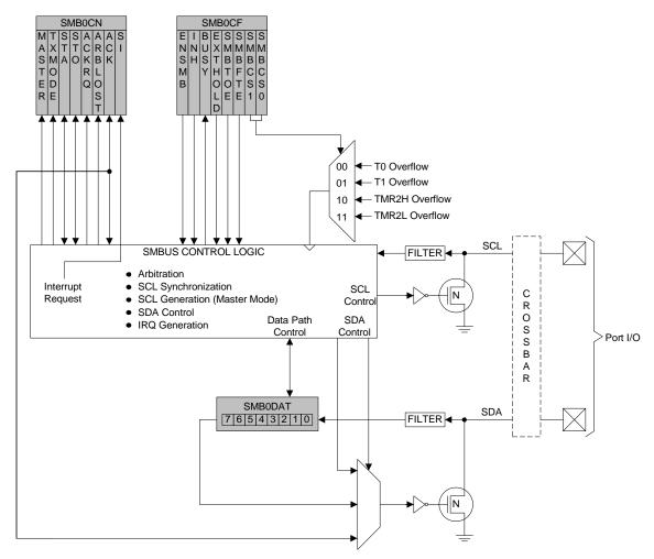
Figure 15.1. SMBus Block Diagram
