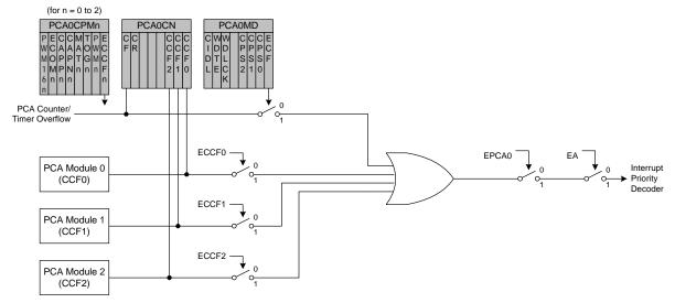
Figure 19.3. PCA Interrupt Block Diagram
