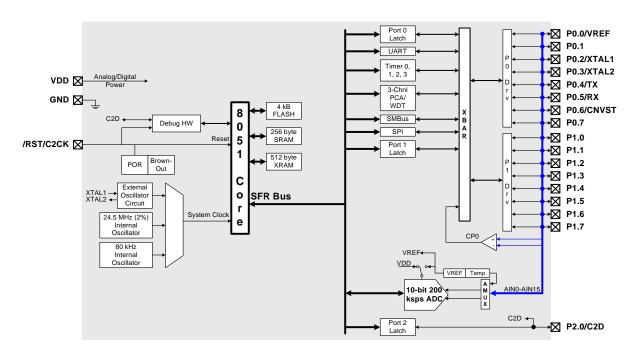
Figure 1.3. C8051F332 Block Diagram
