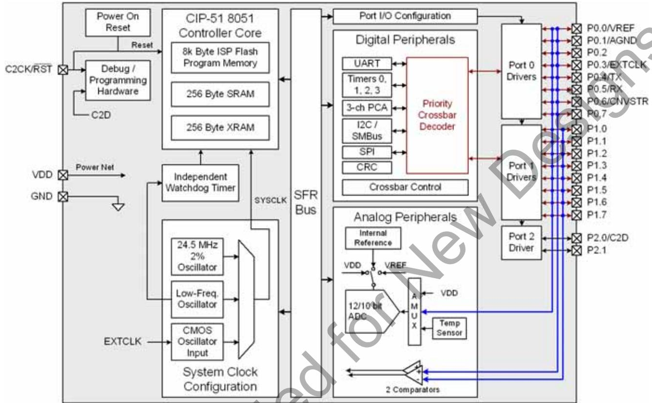
Figure 2.1. C8051F85x/86x Family Block Diagram (QSOP-24 Shown)
