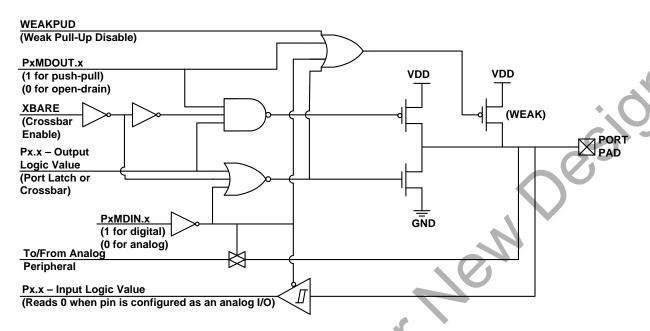
Figure 21.2. Port I/O Cell Block Diagram
