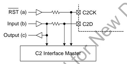
Figure 27.1. Typical C2 Pin Sharing
