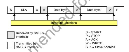
Figure 22.5. Typical Master Write Sequence
