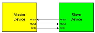
Figure 24.3. 3-Wire Single Master and 3-Wire Single Slave Mode Connection
