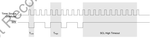
Figure 22.4. Typical SMBus SCL Generation
