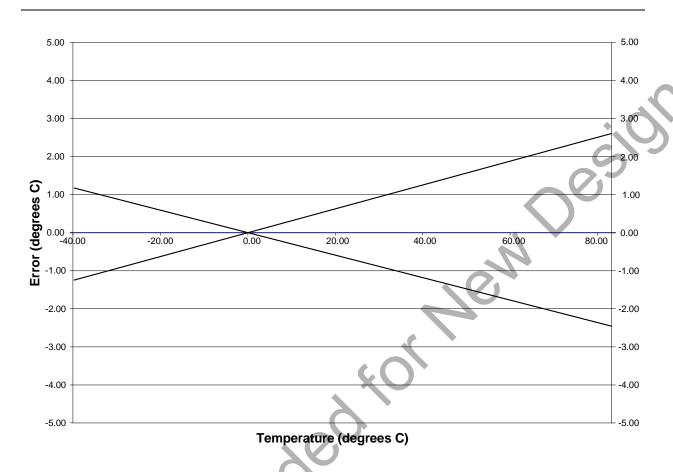
Figure 9.2. Temperature Sensor Error with 1-Point Calibration at 0 Celsius
