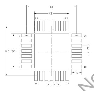
Figure 5.2. QFN-28 Recommended PCB Land Pattern
