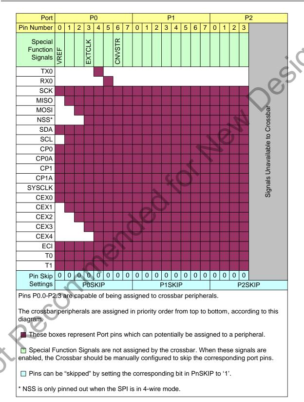
Figure 21.3. Priority Crossbar Decoder Potential Pin Assignments
