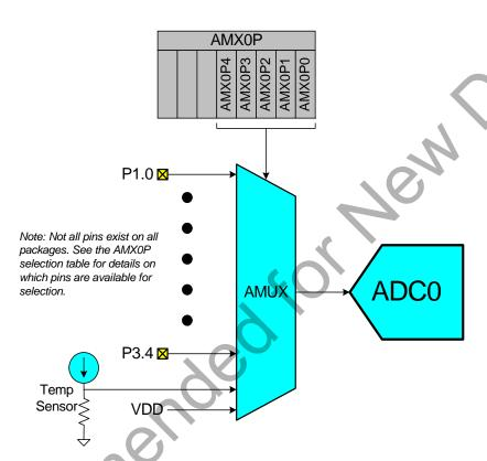
Figure 8.6. ADC0 Multiplexer Block Diagram
