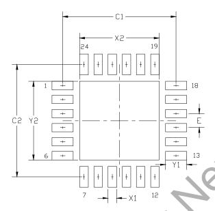
Figure 6.2. QFN-24 Recommended PCB Land Pattern
