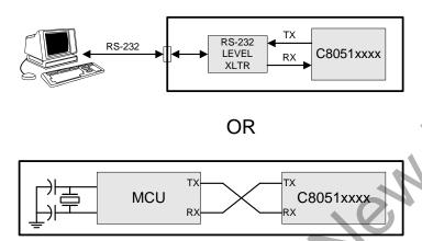
Figure 23.3. UART Interconnect Diagram
