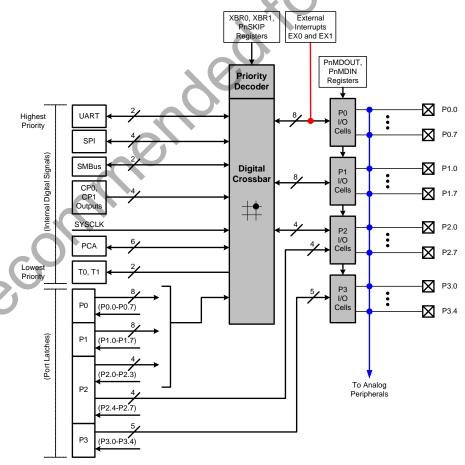
Figure 21.1. Port I/O Functional Block Diagram
