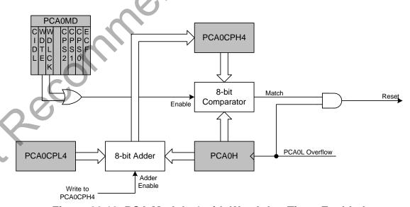
Figure 26.10. PCA Module 4 with Watchdog Timer Enabled
