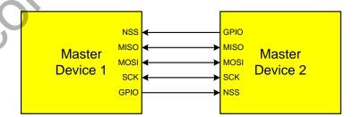
Figure 24.2. Multiple-Master Mode Connection Diagram
