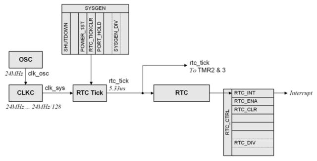
Figure 33.1. RTC Timer Block Diagram
