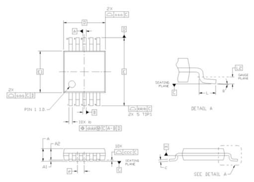
Figure 7.1. 10-Pin MSOP Package
