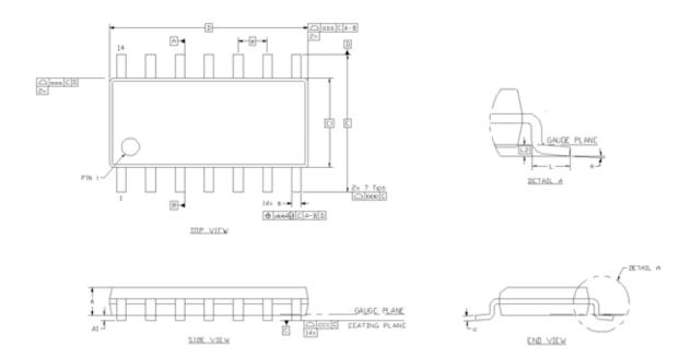
Figure 7.2. 14-Pin SOIC Package
