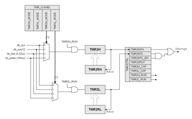
Figure 34.4. Two 8-bit Timers in Timer/Timer Configuration (Split Mode)
