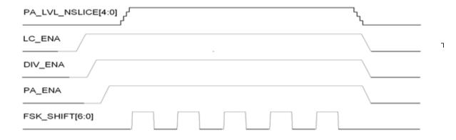
Figure 13.2. FSK Timing Example
