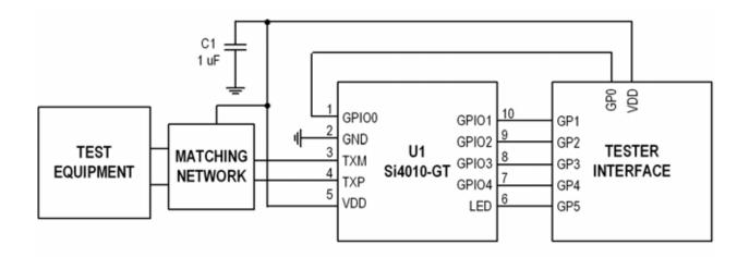
Figure 2.1. Test Block Diagram with 10-Pin MSOP
