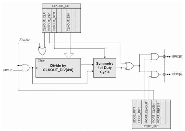
Figure 31.1. Output Clock Generator Block Diagram
