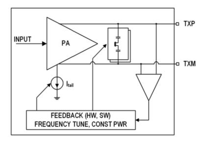
Figure 12.1. Simplified PA block Diagram
