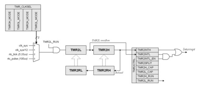
Figure 34.2. Timer 16-bit Mode Block Diagram (Wide Mode)
