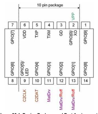
Figure 30.1. Device Package and Port Assignments
