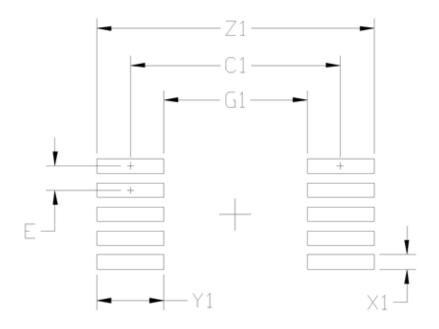
Figure 8.1. 10-Pin MSOP Recommended PCB Land Pattern
