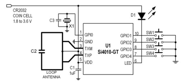
Figure 3.2. Si4010 with an External Crystal in a 4-button RKE System with LED Indicator
