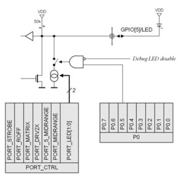
Figure 30.5. GPIO[5] LED Driver Block Diagram
