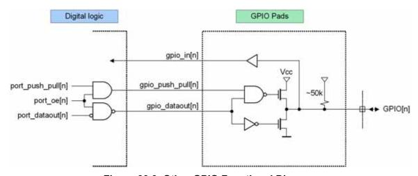
Figure 30.3. Other GPIO Functional Diagram
