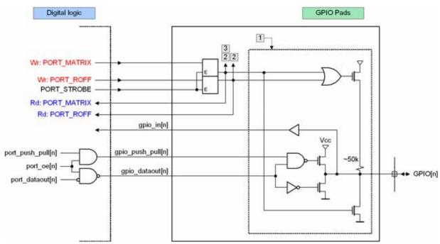
Figure 30.2. GPIO[3:1] Functional Diagram
