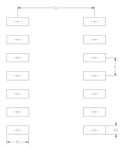
Figure 9.1. 14-Pin SOIC Recommended PCB Land Pattern
