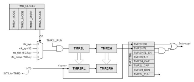
Figure 34.3. Capture 16-bit Mode Block Diagram (Wide Mode)
