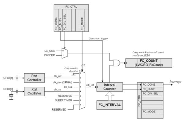
Figure 17.1. Frequency Counter Block Diagram
