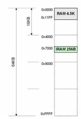
Figure 24.3. Boot Routine Destination CPU Address Space for Copy from NVM
