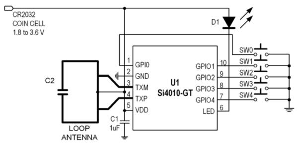
Figure 3.1. Si4010 Used in a 5-button RKE System with LED Indicator
