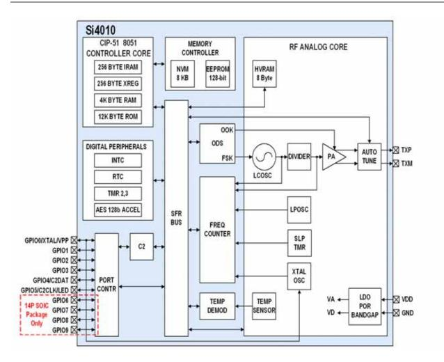
Figure 1.1. Si4010 Block Diagram
