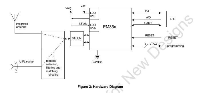
The ETRX351, ETRX351HR, ETRX357 and ETRX357HR are based on the Ember EM351 and EM357 respectively. The EM351 and EM357 are fully integrated 2.4GHz Zigbee transceivers with a 32-bit ARM<sup>®</sup> Cortex M3<sup>™</sup> microprocessor, flash and RAM memory, and peripherals.
