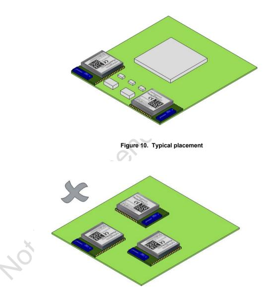
Figure 11. How to not place the Module
