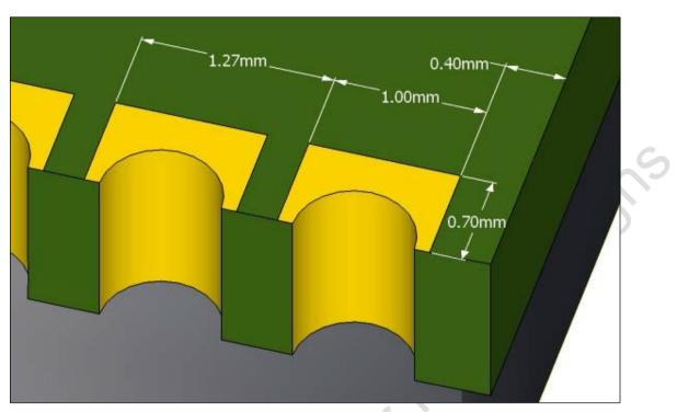
Figure 6. Typical pad dimensions
