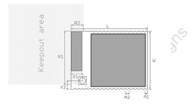
Figure 5: ETRX3 Physical Dimensions
