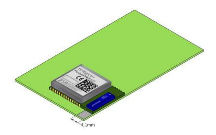
Figure 12. Adding a no copper / no component area
