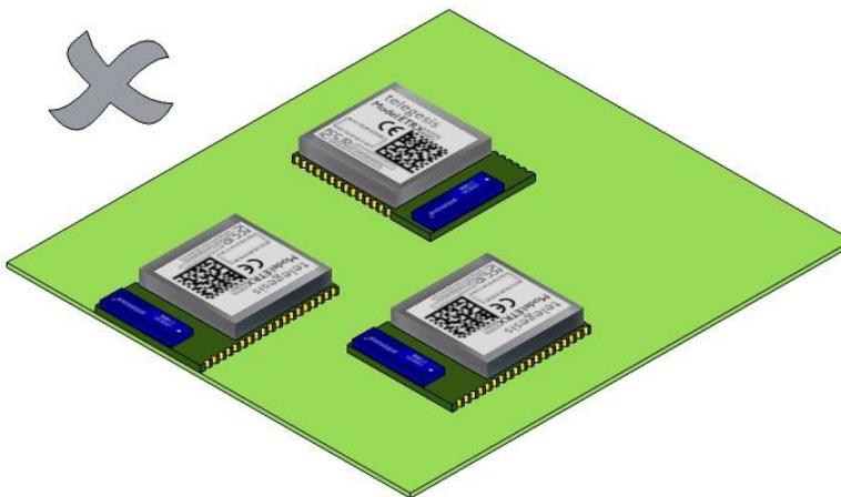
Figure 13. How to not place the Module
