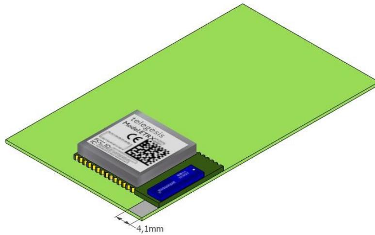
Figure 14. Adding a no copper / no component area
