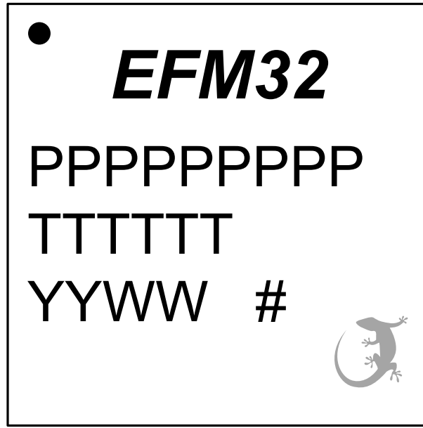
Figure 8.3. QFN32 Package Marking
