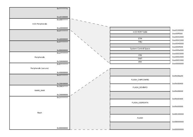
Figure 3.2. EFM32PG28 Memory Map — Core Peripherals and Code Space
