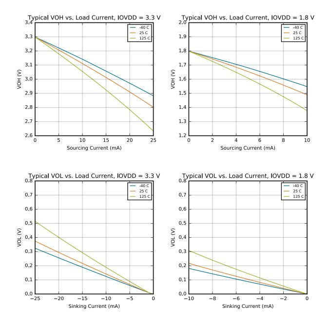
Figure 4.11. VOH and VOL vs. Load Current
