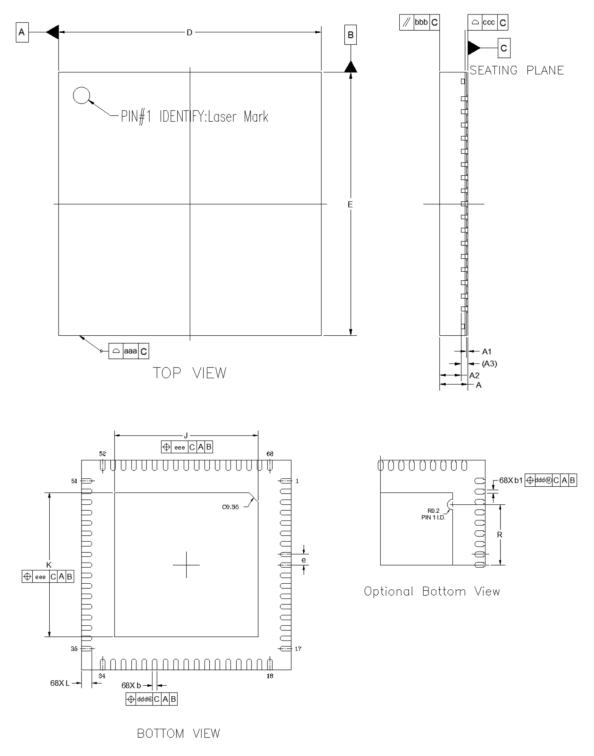
Figure 7.1. QFN68 Package Drawing
