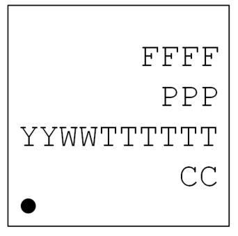
Figure 7.3. QFN68 Package Marking
