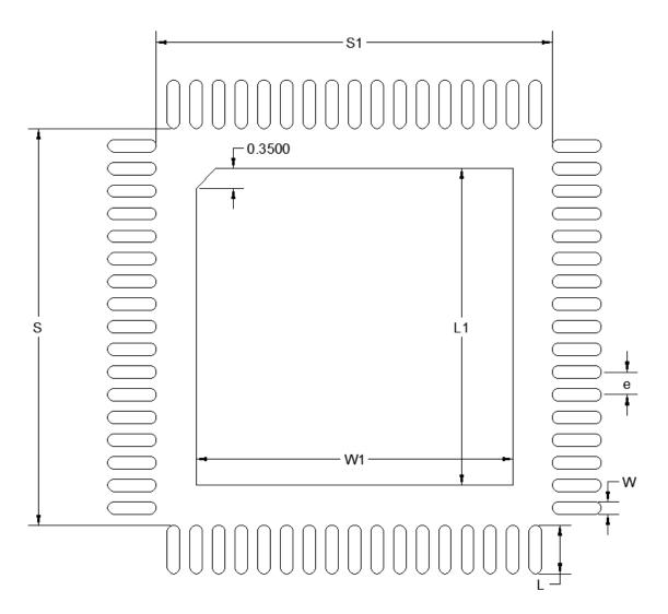
Figure 7.2. QFN68 PCB Land Pattern Drawing
