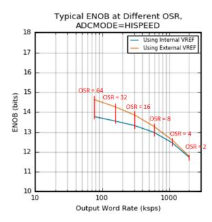
Figure 4.10. Typical ENOB vs. Oversampling Ratio
