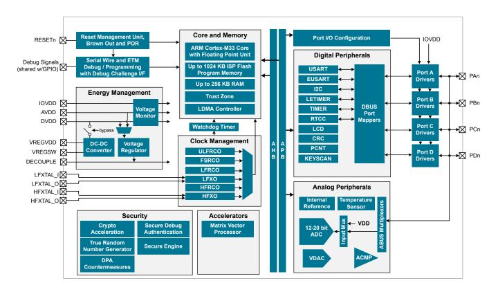
Figure 3.1. Detailed EFM32PG28 Block Diagram
