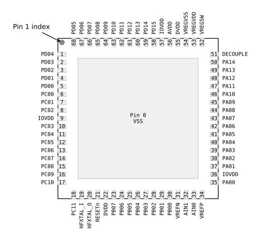
Figure 6.1. QFN68 Device Pinout
