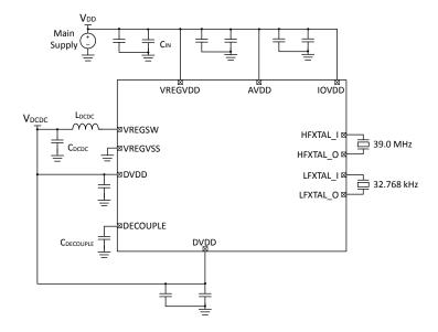
Figure 5.2. EFM32PG28 Typical Application Circuit: DCDC Configuration
