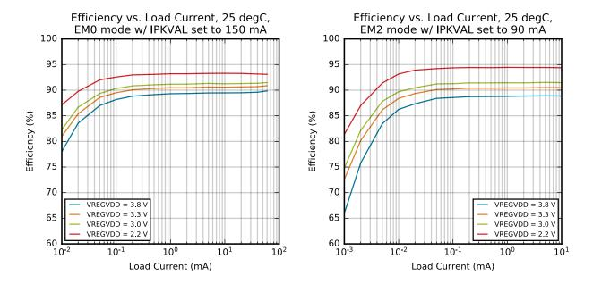
Figure 4.9. DC-DC Efficiency
