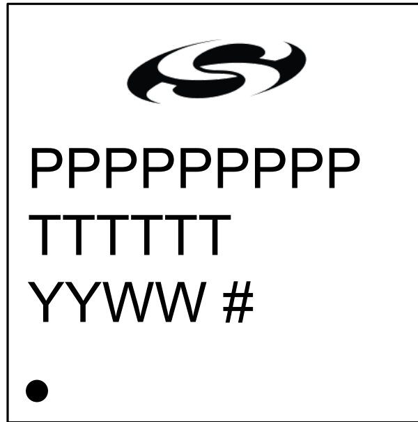
Figure 7.3. CSP Package Marking
