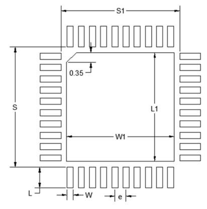
Figure 7.2. QFN40 PCB Land Pattern Drawing
