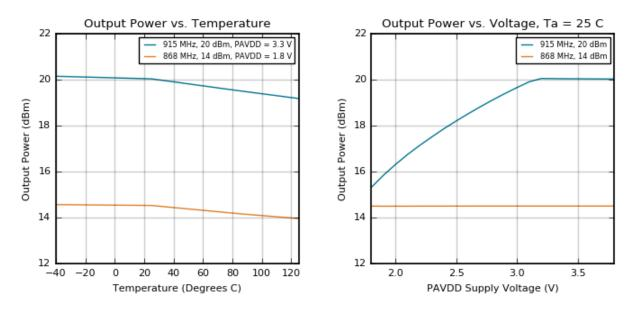
Figure 4.9. Transmitter Output Power
