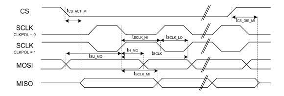
Figure 4.4. SPI Secondary Timing (SSSEARLY = 1)
