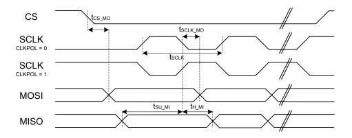
Figure 4.2. SPI Main Timing (SMSDELAY = 1)
