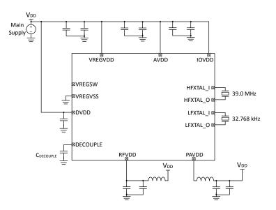
Figure 5.1. EFR32FG23 Typical Application Circuit: Direct Supply Configuration without DCDC
