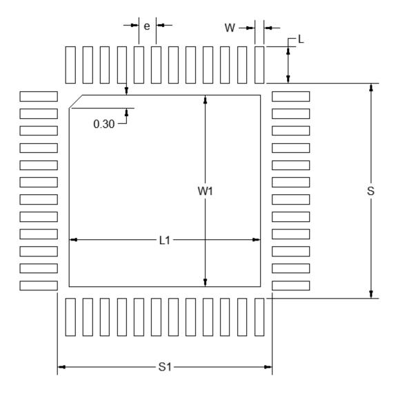
Figure 8.2. QFN48 PCB Land Pattern Drawing
