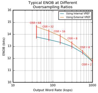
Figure 4.11. Typical ENOB vs. Oversampling Ratio
