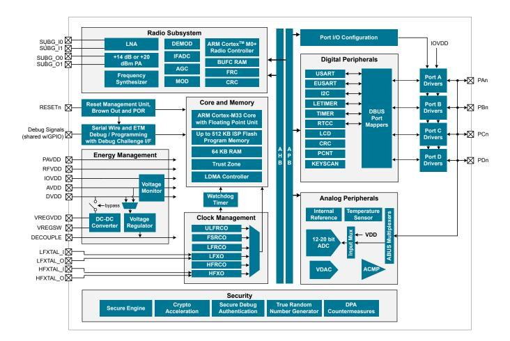
Figure 3.1. Detailed EFR32FG23 Block Diagram
