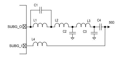
Figure 5.5. Typical 868/915/920 MHz RF impedance-matching network circuit, +20 dBm
