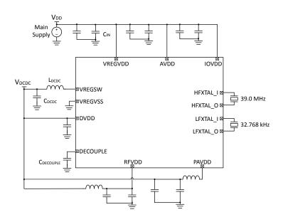
Figure 5.2. EFR32FG23 Typical Application Circuit: DCDC Configuration
