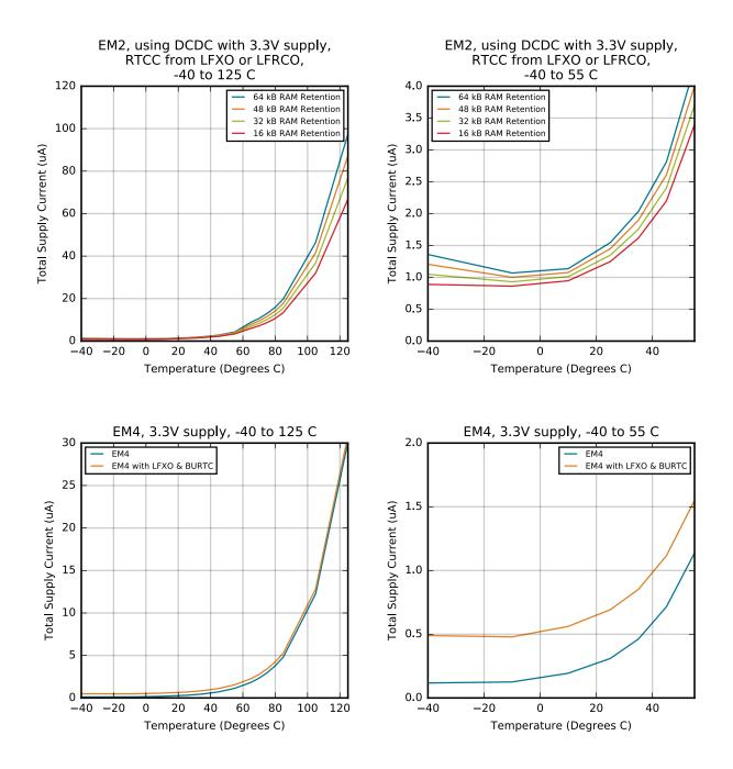
Figure 4.8. EM2 and EM4 Typical Supply Current vs. Temperature
