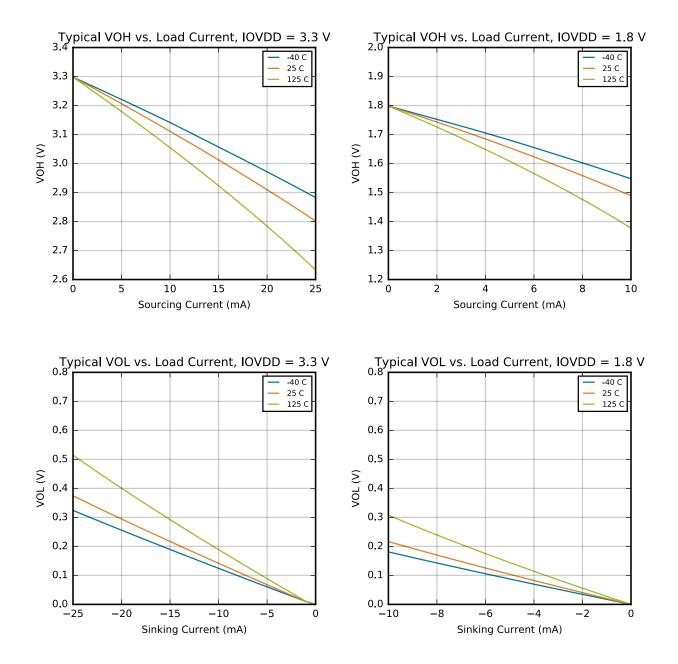
Figure 4.12. VOH and VOL vs. Load Current
