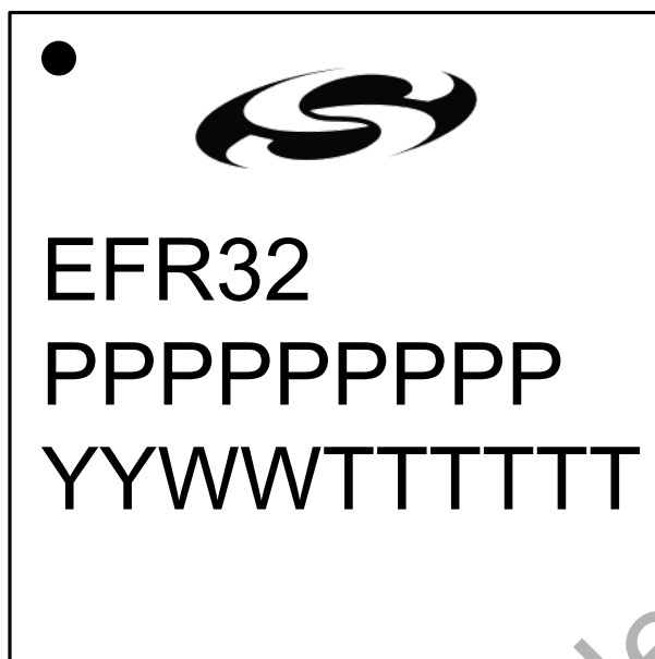
Figure 8.3. QFN32 Package Marking
