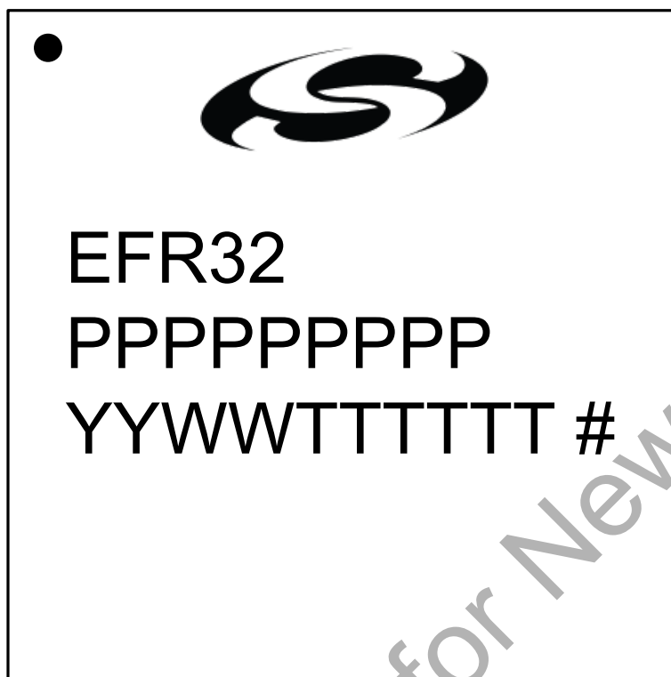
Figure 7.3. QFN48 Package Marking
