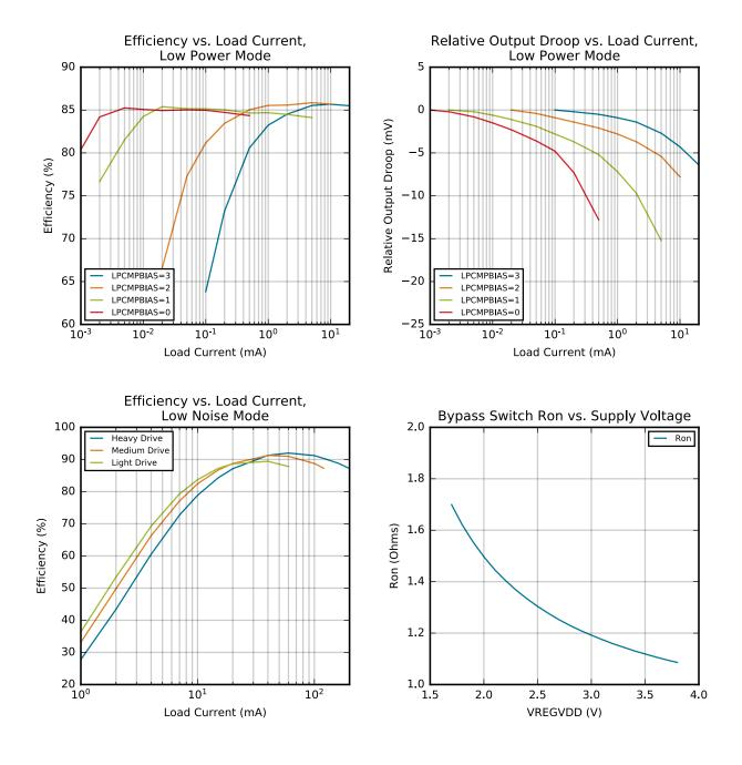
Figure 4.9. DC-DC Converter Typical Performance Characteristics
