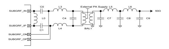
Figure 5.5. Typical Sub-GHz RF impedance-matching network circuits
