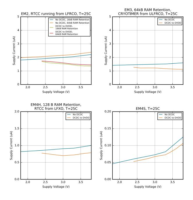
Figure 4.8. EM2, EM3, EM4H and EM4S Typical Supply Current vs. Supply
