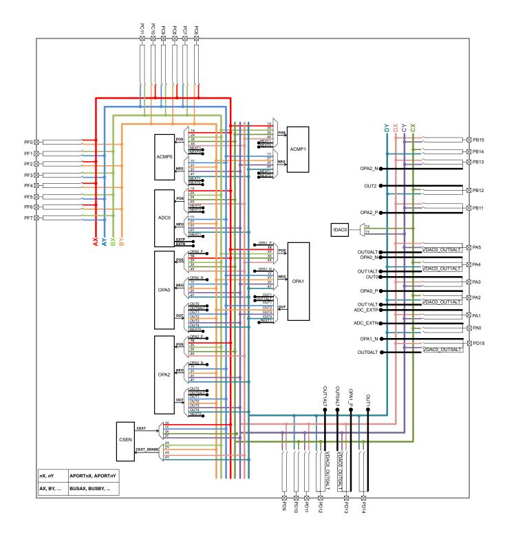
Figure 6.4. APORT Connection Diagram
