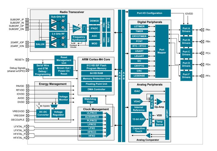
Figure 3.1. Detailed EFR32MG13 Block Diagram
