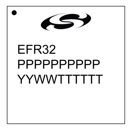
Figure 7.3. QFN48 Package Marking
