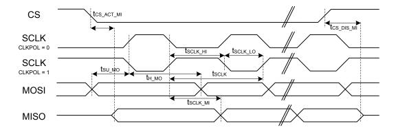
Figure 4.2. SPI Slave Timing Diagram
