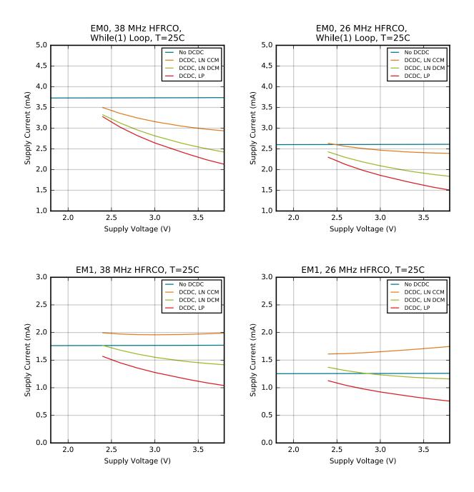
Figure 4.7. EM0 and EM1 Mode Typical Supply Current vs. Supply
