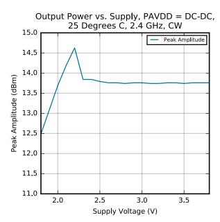
Figure 4.11. 2.4 GHz RF Transmitter Output Power
