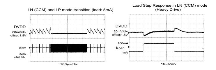
Figure 4.10. DC-DC Converter Transition Waveforms
