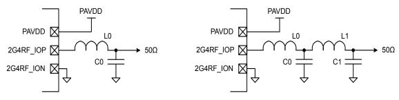
Figure 5.4. Typical 2.4 GHz RF impedance-matching network circuits
