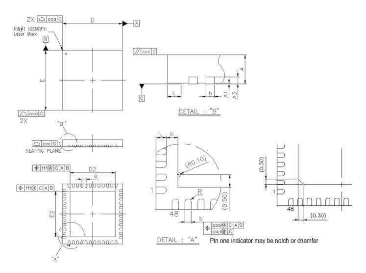
Figure 7.1. QFN48 Package Drawing
