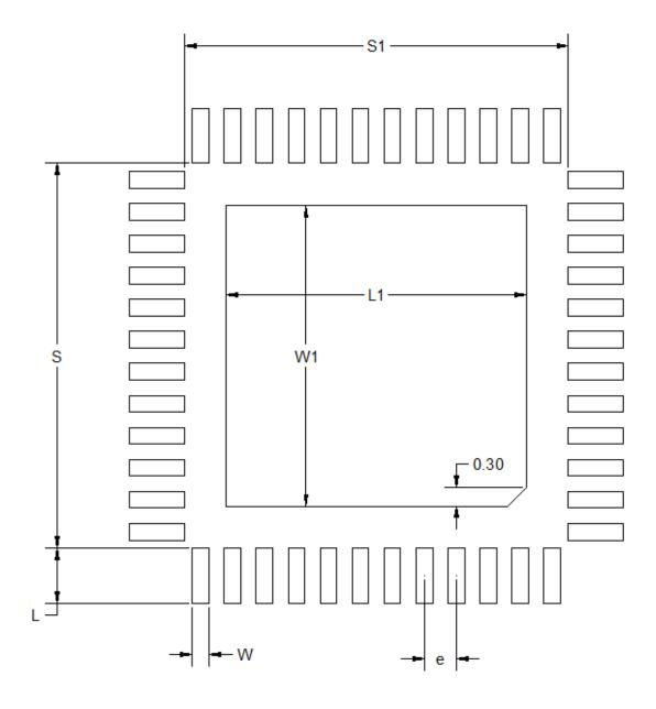
Figure 7.2. QFN48 PCB Land Pattern Drawing
