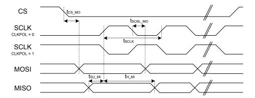
Figure 4.1. SPI Master Timing Diagram
