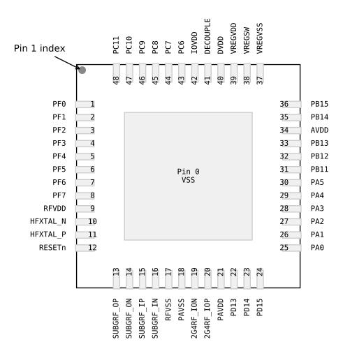
Figure 6.1. QFN48 2.4 GHz and Sub-GHz Device Pinout
