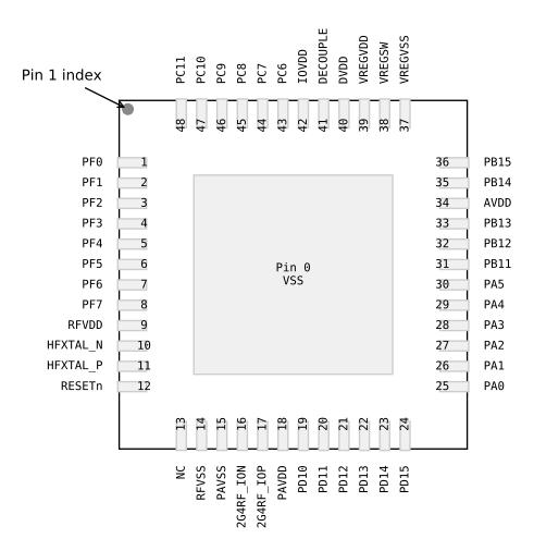
Figure 6.2. QFN48 2.4 GHz Device Pinout
