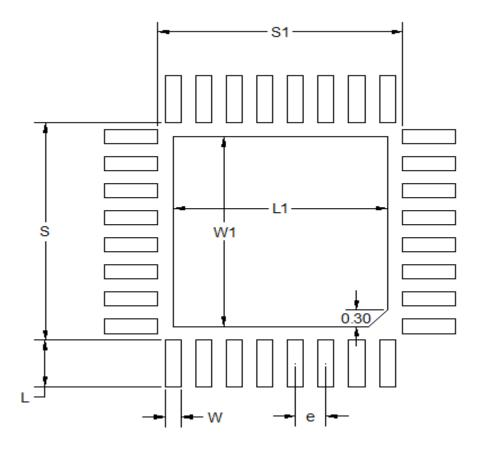
Figure 8.2. RQFN32 PCB Land Pattern Drawing
