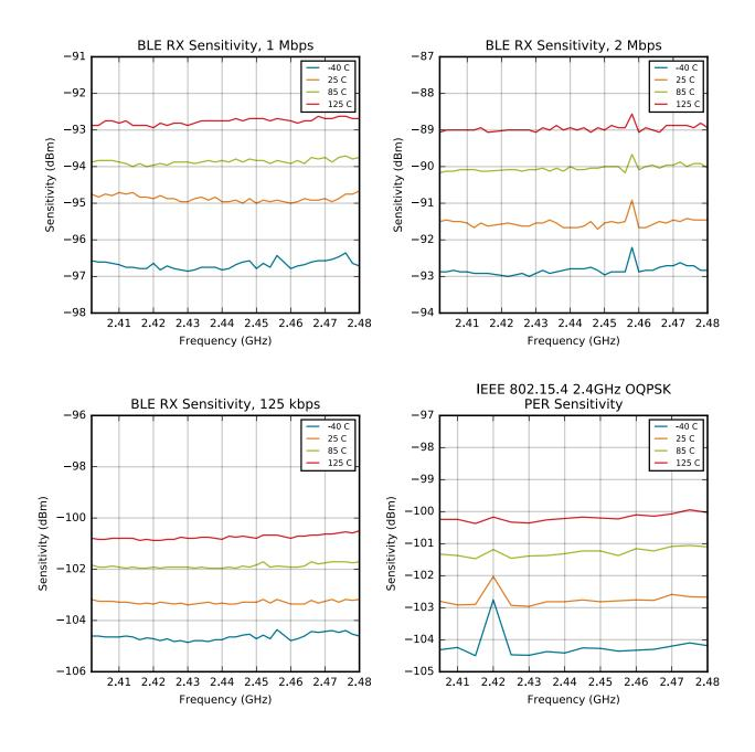
Figure 4.12. 2.4 GHz RF Receiver Sensitivity
