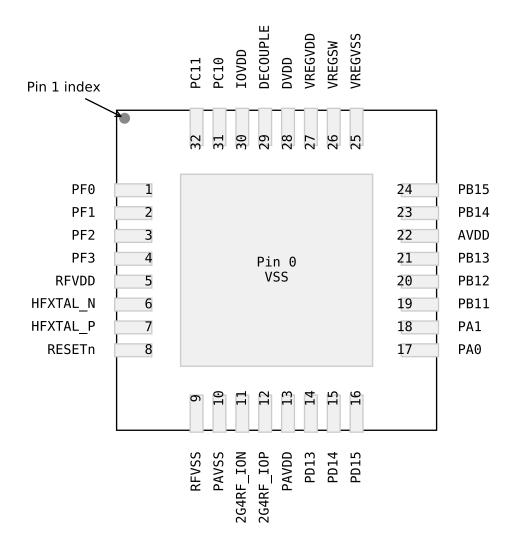
Figure 6.3. QFN32 2.4 GHz Device Pinout
