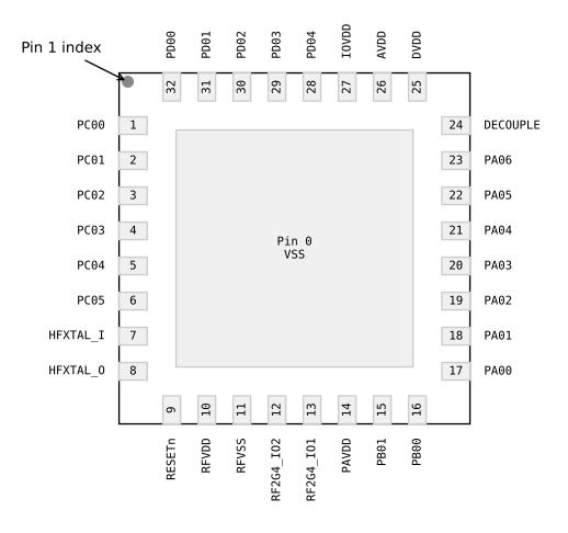
Figure 6.1. QFN32 Device Pinout
