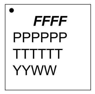
Figure 7.3. QFN32 Package Marking
