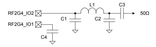
Figure 5.2. Typical 0 dBm 2.4 GHz RF impedance-matching network circuit
