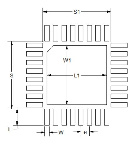
Figure 7.2. QFN32 PCB Land Pattern Drawing
