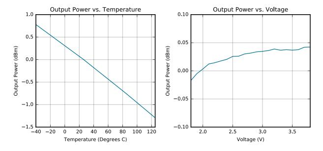
Figure 4.8. 2.4 GHz 0 dBm PA RF Transmitter Output Power
