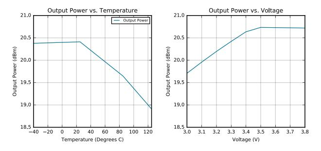
Figure 4.6. 2.4 GHz 20 dBm PA RF Transmitter Output Power
