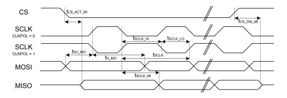
Figure 4.13. SPI Secondary Timing
