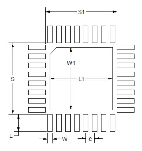
Figure 7.2. QFN32 PCB Land Pattern Drawing
