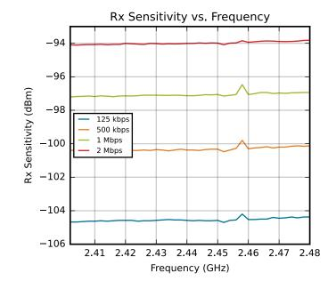
Figure 4.20. 2.4 GHz BLE RF Receiver Sensitivity
