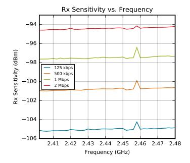
Figure 4.10. 2.4 GHz BLE RF Receiver Sensitivity
