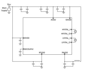
Figure 5.1. EFR32MG21 Typical Application Circuit: Direct Supply Configuration
