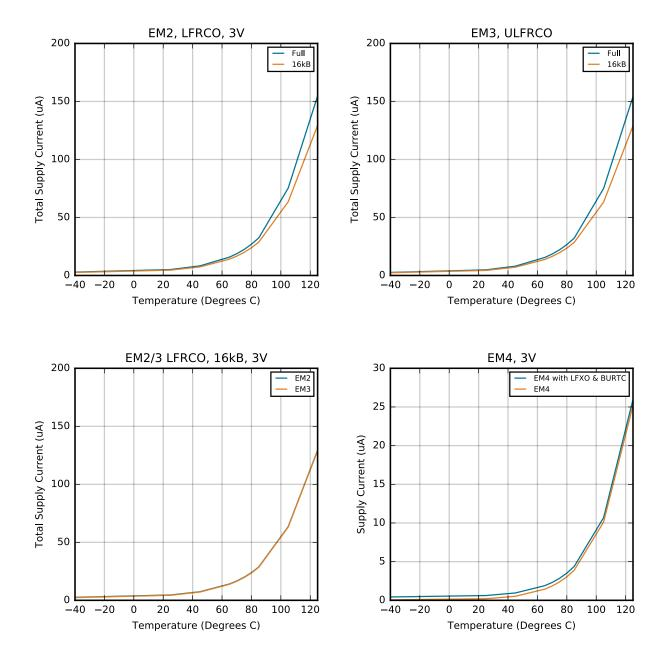
Figure 4.5. EM2, EM3, and EM4 Sleep Mode Typical Supply Current vs. Temperature
