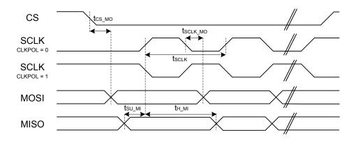
Figure 4.1. SPI Main Timing (SMSDELAY = 0)
