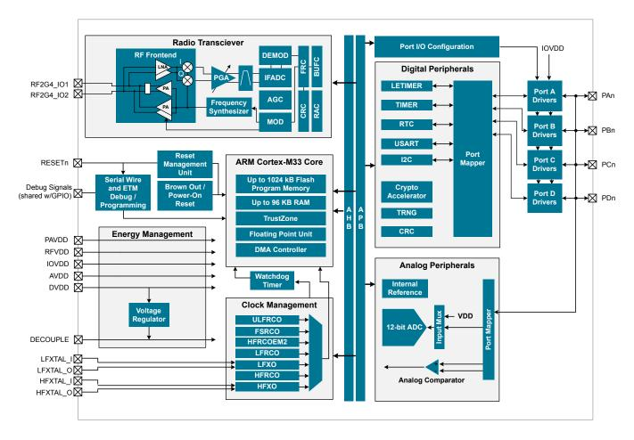
Figure 3.1. Detailed EFR32MG21 Block Diagram
