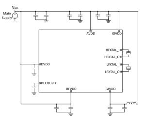
Figure 5.1. EFR32MR21 Typical Application Circuit: Direct Supply Configuration
