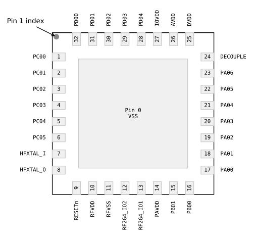
Figure 6.1. QFN32 Device Pinout
