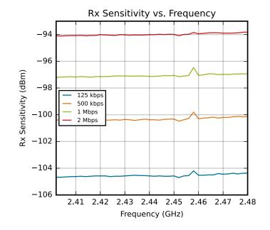
Figure 4.7. 2.4 GHz BLE RF Receiver Sensitivity
