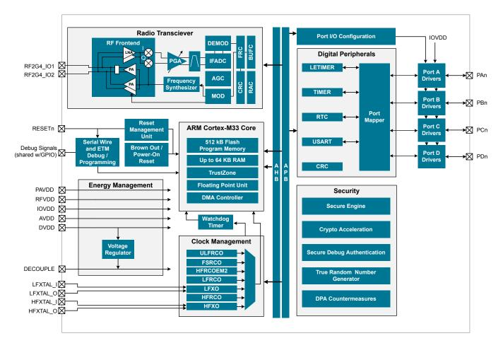
Figure 3.1. Detailed EFR32MR21 Block Diagram
