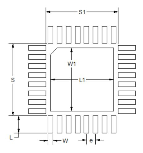
Figure 7.2. QFN32 PCB Land Pattern Drawing
