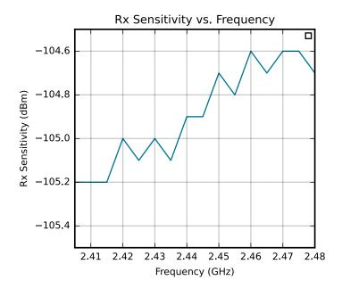
Figure 4.6. 2.4 GHz 802.15.4 RF Receiver Sensitivity
