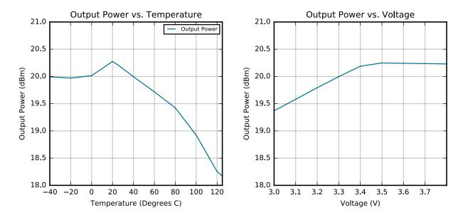
Figure 4.5. 2.4 GHz 20 dBm PA RF Transmitter Output Power
