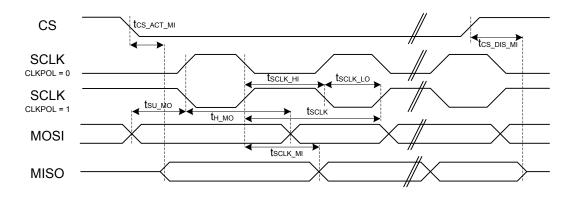
Figure 4.3. SPI Secondary Timing
