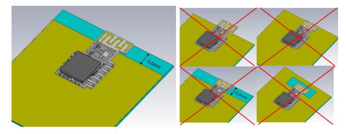
Figure 7.2. Horizontal Mounting
