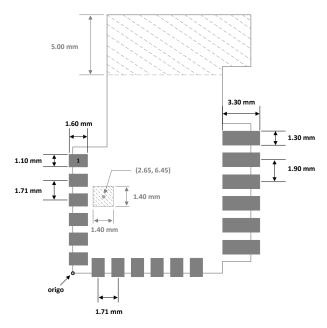
Figure 8.3. Recommended Module PCB Land Pattern
