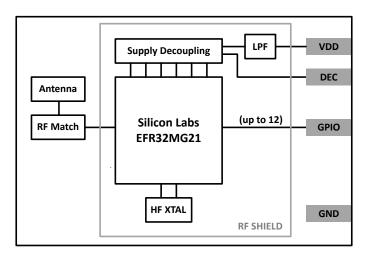
Figure 3.1. MGM210L Block Diagram
