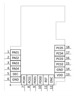
Figure 6.1. MGM210L Lighting Module Pinout
