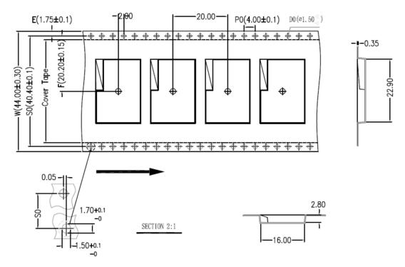
Figure 10.1. Carrier Tape Dimensions
