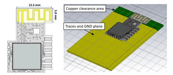
Figure 7.1. Inverted-F Antenna Clearance
