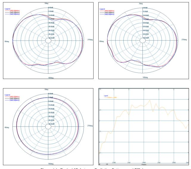
Figure 4.1. Typical 2D Antenna Radiation Patterns and Efficiency
