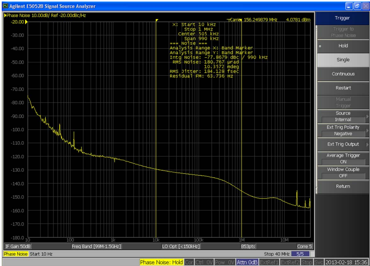
Figure 1. Si535/536 Typical Phase Noise at 156.25 MHz
