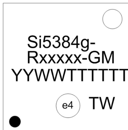
Figure 12.2. Si5384 Top Marking
