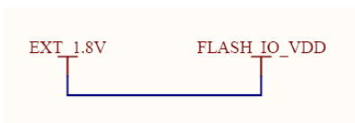
Figure 8.27. Option 2: In-Package PSRAM Powered From External 1.8 V Supply
