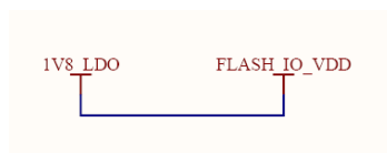
Figure 8.22. Option 1: In-Package Common Flash (NWP + MCU) Powered From On-Chip LDO Supply
