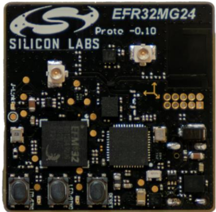
Example board supporting 2 antenna paths
