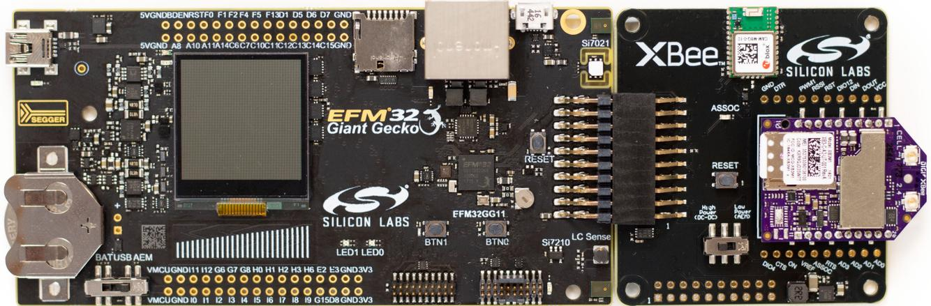
2. Once the expansion board is connected, the EFM32GG11 STK can then be powered by connecting the USB connector on the left and setting the switch to the AEM position.
