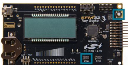
6. The fourth screen shows data coming from the capacitive sense slider. The EFM32TG11 Tiny Gecko has an advanced SAR-based capacitive touch peripheral with up to 64 inputs that provides the touch measurements. The top line of the display, next to "F", displays the force of the capacitive touch, while the line next to "POS" displays the position of the touch on the slider, from 0 to 64, from left to right.
