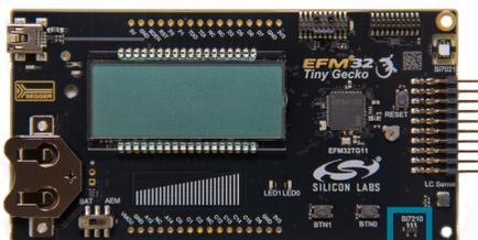
5. The third screen shows the temperature and humidity measured by the Silicon Labs Si7021 Humidity and Temperature Sensor, mounted on the top-right of the kit. Pressing the pushbutton **[BTN1]** will toggle the temperature between Fahrenheit and Celsius.
