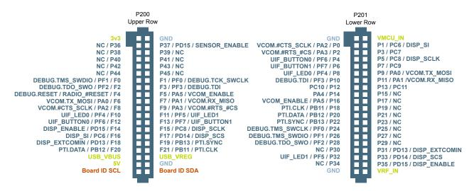
Figure 2.1. BRD4255A Radio Board Connector Pin Mapping
