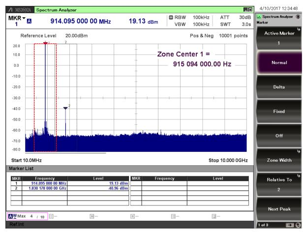
Figure 7.1. Typical Output Spectrum of the BRD4255A
