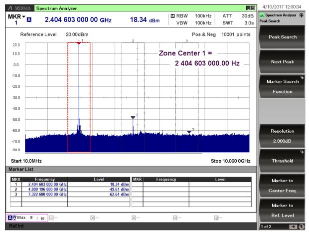
Figure 7.2. Typical Output Spectrum of the BRD4255A
