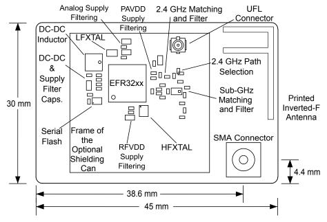
Figure 5.1. BRD4255A Top View
