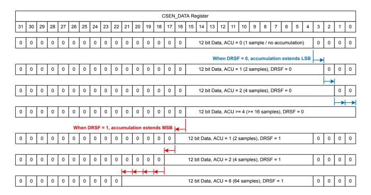
Figure 34.7. Data Encoding for Different Accumulator Settings
