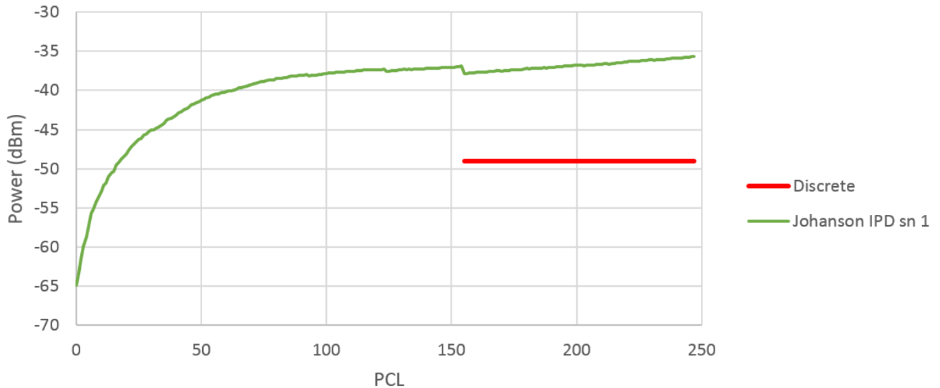
Figure 3.3. Conducted Transmit Second Harmonic Performance of One Johanson IPD
