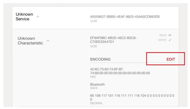
**Question** - Were you able to write the characteristic data? Check the access counters on the bottom of the LCD for help! **In case of pairing request, you need to accept pairing with PB0 button on the WSTK.**
