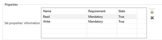
These properties ensure that reading and writing the *Public Data* characteristic is without any restriction. It does not require Authentication or Encrypted link. Any GATT client can read or write it.
