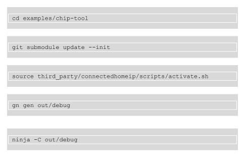
Now, generated binaries for chip-tool are under '~/examples/chip-tool/out/debug' folder. Using chip-tool you can now control the lock status with on/off command. But before that we need to add ipv6 route in next step.
