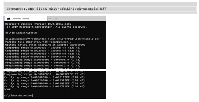
**Note:** You can also manually launch GUI interface of commander.exe file from (C:\SiliconLabs\SimplicityStudio\v5\developer\adapter\_packs\commander) and flash the file to the board
