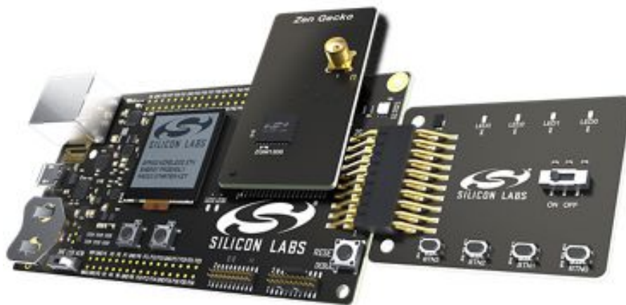
Figure 1: Main development board with Z-Wave SiP module
