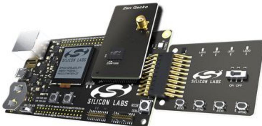
Figure 1: Main Development Board with Z-Wave SiP Module
