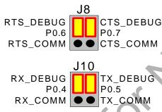
Figure 14. Shorting Block Configuration when Using the USB Debug Adapter
