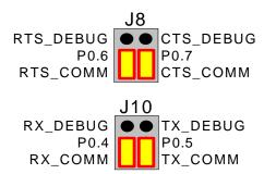
Figure 13. Shorting Block Configuration when Using the CP2103
