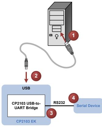
Figure 1. Hardware Setup
