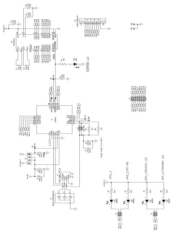
Figure 4. CP2104 Evaluation Board Schematic
