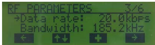
Figure 9. Menu Page: RF Parameters 3/6 (Modulation is OOK)
