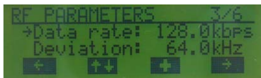
Figure 8. Menu Page: RF Parameters 3/6 (Modulation is 2GFSK)
