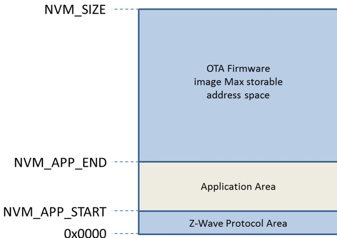
Figure 9, NVM layout for 128Kbytes and 256Kbyte EEPROM.
