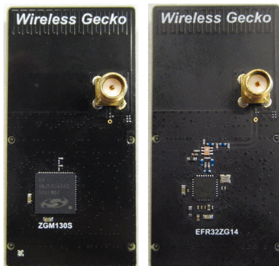
Figure 3: Z-Wave Development Radio Boards (Left: BRD4207A, Right: BRD4206A)
