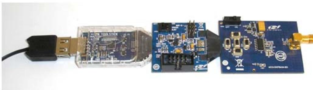
**Note:** Although burning is also possible with this setup, it is not practical since Si4010 is soldered on the key fob development board.
