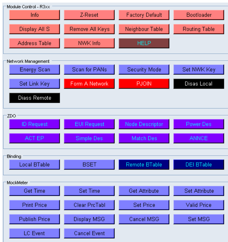
Figure 2. Button layout of the Mock meter panel
